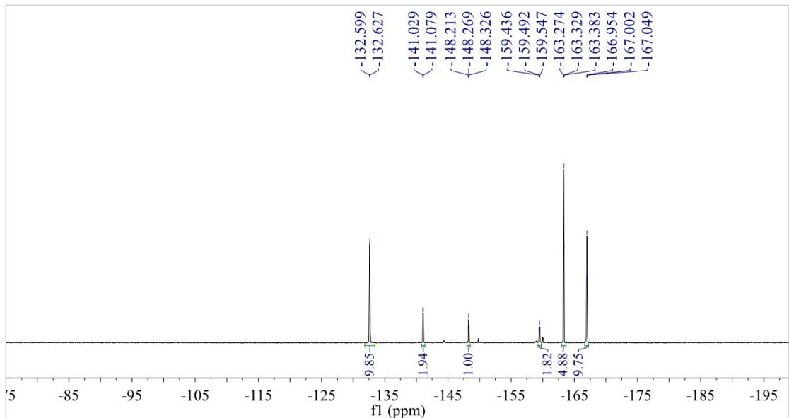
$^{19}\text{F}$  NMR spectrum of **6** (377 MHz,  $\text{CDCl}_3$ ).
