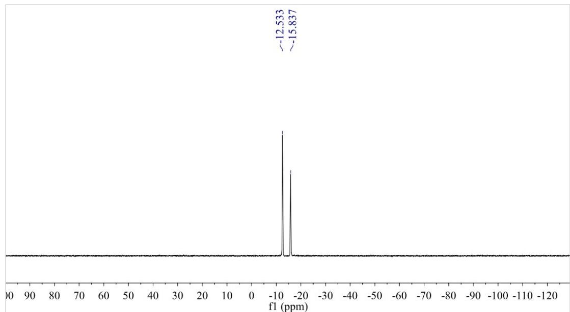
${}^3\text{P}$  NMR spectrum of **1** (162 MHz,  $\text{CDCl}_3$ ):
