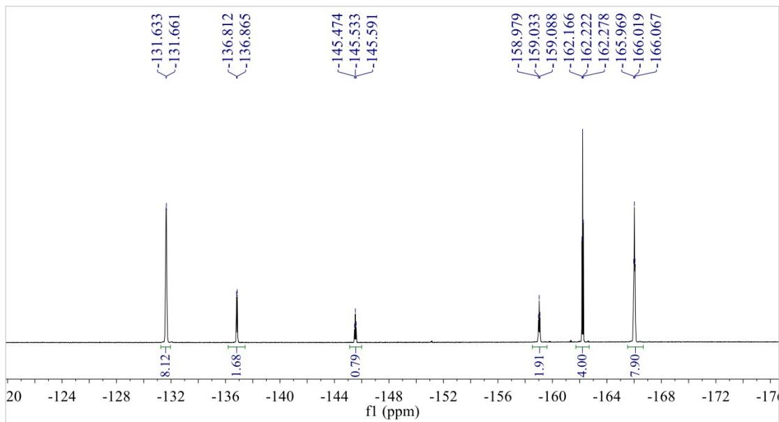
$^{19}\text{F}$  NMR spectrum of **4** (377 MHz,  $\text{C}_6\text{D}_5\text{Br}$ ):
