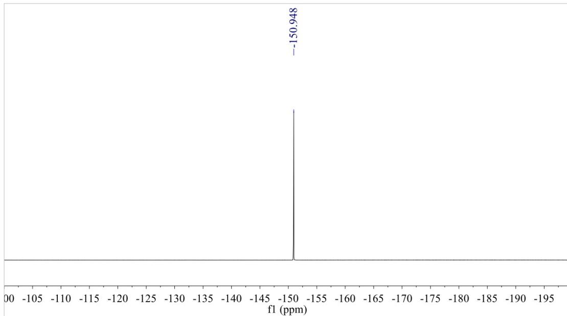
$^{19}\text{F}$  NMR spectrum of **1** (377 MHz,  $\text{CDCl}_3$ ).
