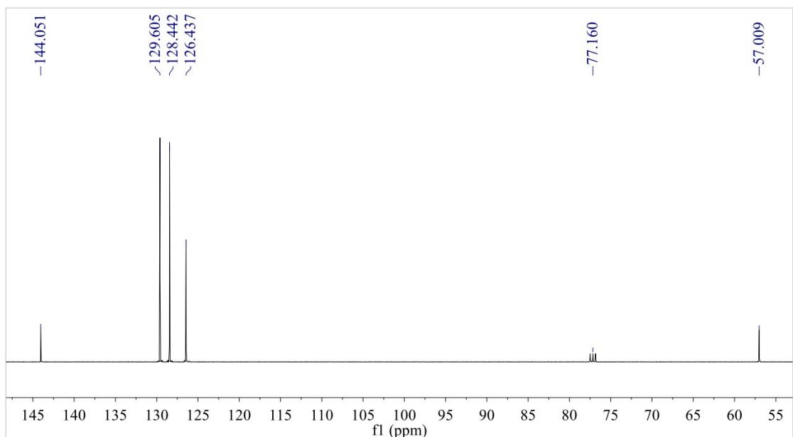
$^{13}\text{C}\{^1\text{H}\}$  NMR spectrum of triphenylmethane (100 MHz, CDCl<sub>3</sub>):
