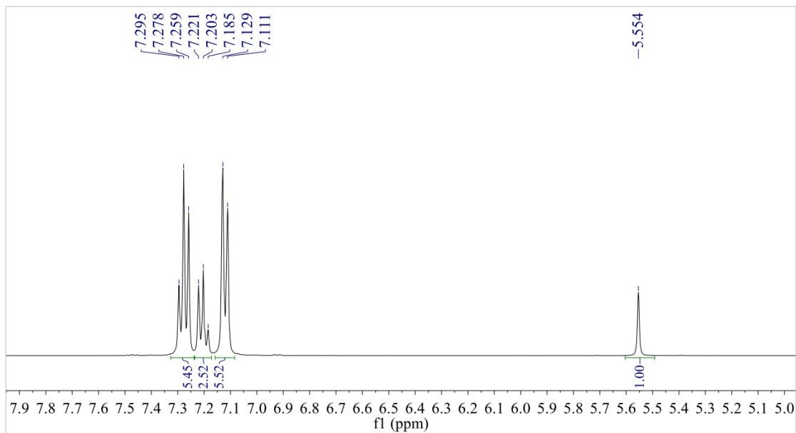
$^1\text{H}$  NMR spectrum of triphenylmethane (400 MHz, CDCl<sub>3</sub>).
