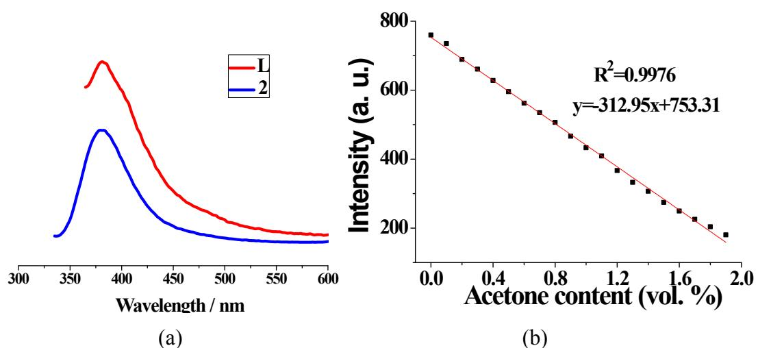
**Fig. S8** (a) Solid-state photoluminescent spectra of free L ligand and **2** at room temperature. (b) Photoluminescence intensities of **2** in  $\text{CH}_3\text{CN}$  as a function of acetone content.
