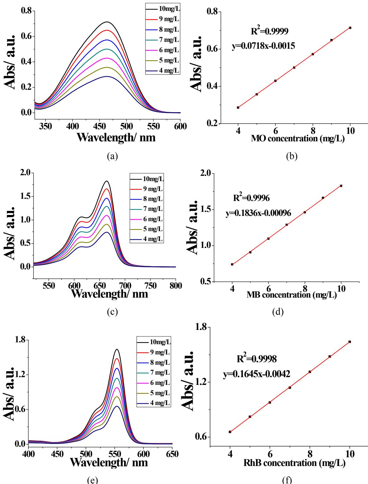
**Fig. S6** UV-vis spectra of a solution of Methyl Orang (a), Methylene blue (c), Rhodamine B (e) at different concentration, standard curves for MO (b), standard curves for MB (d), standard curves for RhB (f).
