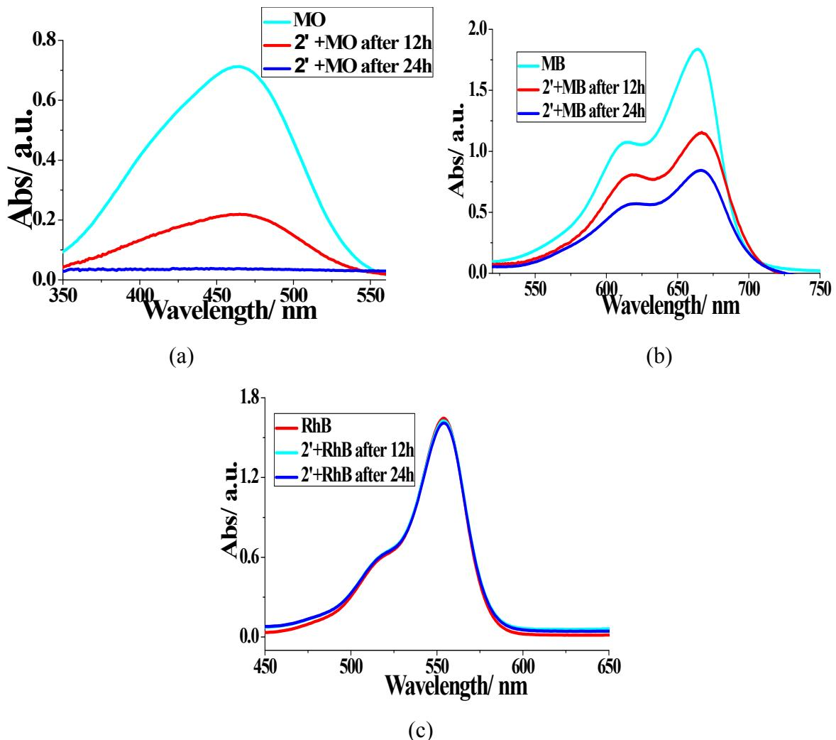
**Fig. S7** Adsorption capability of **2'** toward MO (a), MB (b) and RhB (c) (experiment conditions:  $C_0$  (MB):  $10 \text{ mg L}^{-1}$ ,  $C_0$  (MO):  $10 \text{ mg L}^{-1}$ , adsorbent dose:  $10 \text{ mg}/20 \text{ mL}$ ).
