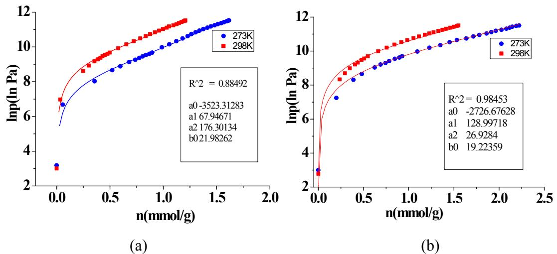
**Fig. S5** The calculated virial equation isotherms parameters fit to the experimental CO<sub>2</sub> data of **1'** (a) and **2'** (b).
