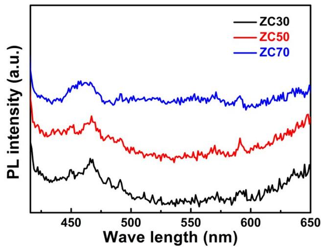
**Fig. S10.** Room temperature photoluminescence (PL) excitation spectra of the solid solutions with different Cd content derived from ZIF-8.
