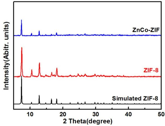
**Fig. S1.** The X-ray diffraction patterns of the ZIF-8 and ZnCo-ZIF with Co content of 0.5 at%.
