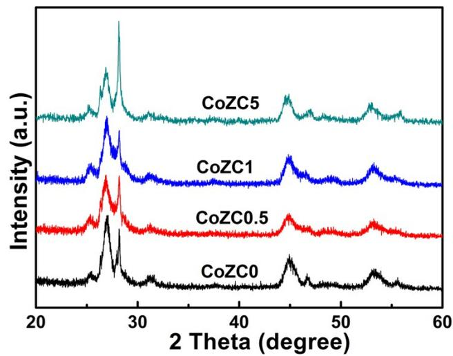
**Fig. S2.** Effect of the Co doping on the X-ray diffraction patterns of the Zn<sub>0.5</sub>Cd<sub>0.5</sub>C<sub>x</sub>S samples. Due to the tiny content of Co, there was no dramatically differences in the XRD patterns of the as-prepared samples.
