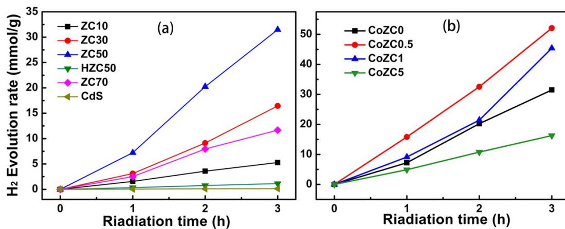
**Fig. S7.** Comparison of the action spectra of H<sub>2</sub>-evolution for the samples with the (a) different Cd content derived from ZIF-8 and (b) different Co doping derived from ZnCo-ZIF.
