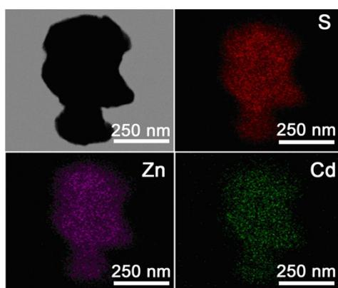
**Fig. S6.** The element mapping images of the  $Zn_{0.5}Cd_{0.5}S$  with Co content of 0.5 at% derived from ZnCo-ZIF.
