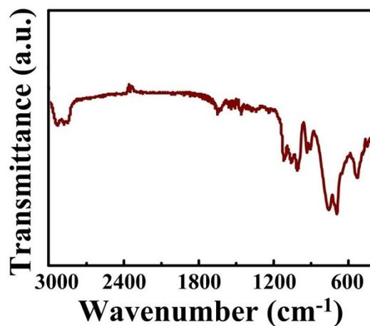
**Figure S2** FT-IR spectrum of the  $\text{Nb}_3(\text{C}_3\text{H}_5\text{O}_3)_5$  precursor.
