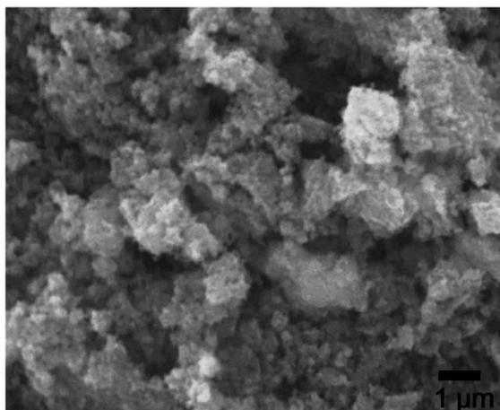
**Figure S6** SEM image of H-Nb<sub>2</sub>O<sub>5</sub> nanoparticles as isopropanol is replaced by 30 mL distilled water with other reaction parameters unchanged.
