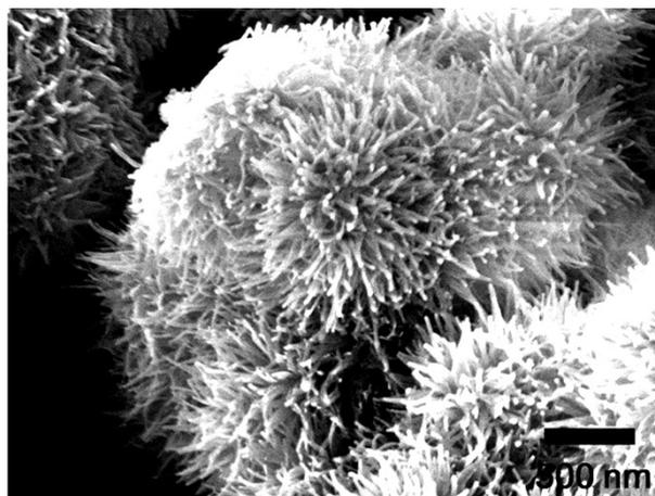
**Figure S4** SEM image of the Nb<sub>3</sub>(C<sub>3</sub>H<sub>5</sub>O<sub>3</sub>)<sub>5</sub> precursor.
