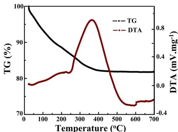
**Figure S3** TG-DTA curves of the  $\text{Nb}_3(\text{C}_3\text{H}_5\text{O}_3)_5$  precursors
