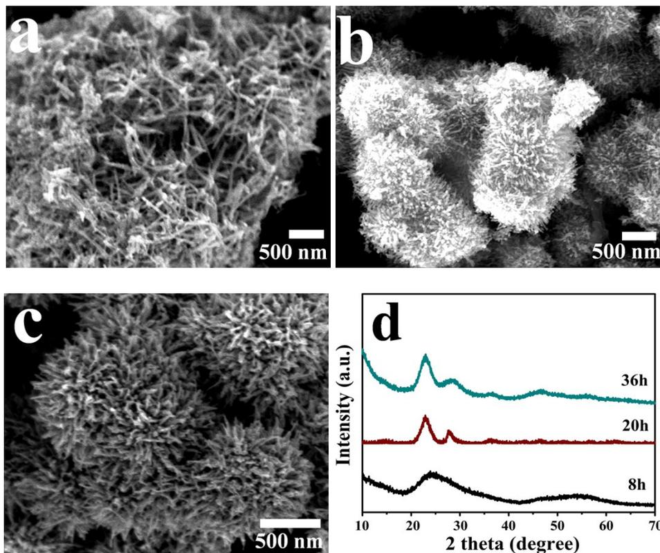
**Figure S5** SEM images of the precursors formed at different reaction times with the other reaction parameters unchanged: (a) 8 h; (b) 20 h; and (c) 36 h; (d) XRD patterns of the precursors formed at different reaction times.
