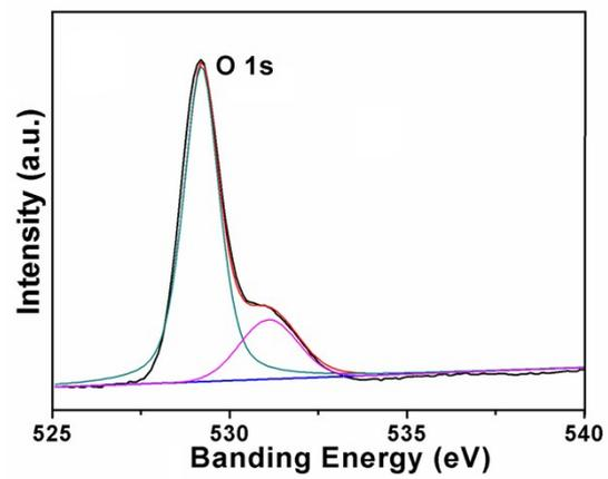
**Figure S1** High-resolution XPS O 1s spectrum of urchin-like H-Nb<sub>2</sub>O<sub>5</sub> microspheres.
