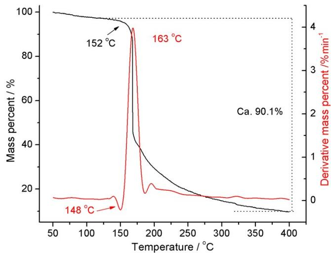
**Figure S13** TG and DTG curves of **12** under nitrogen with a heating rate of  $5\text{ }^{\circ}\text{C min}^{-1}$ .
