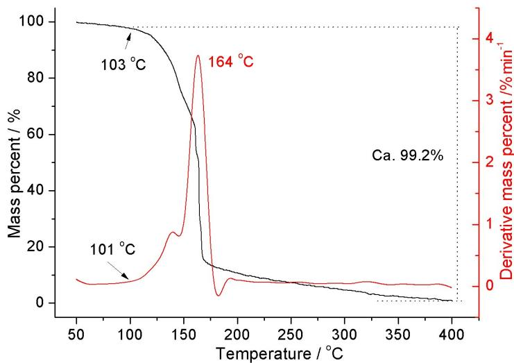
**Figure S10** TG and DTG curves of **9** under nitrogen with a heating rate of  $5\text{ }^{\circ}\text{C min}^{-1}$ .
