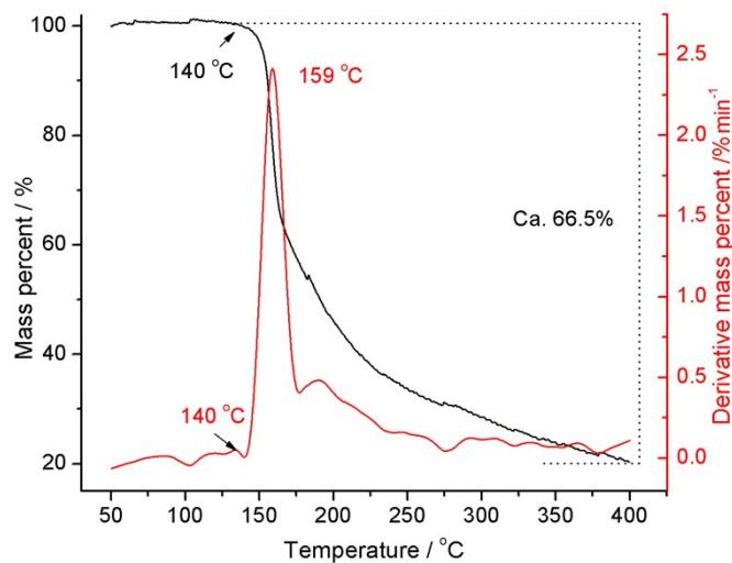
**Figure S7** TG and DTG curves of **6** under nitrogen with a heating rate of 5 °C min<sup>-1</sup>.
