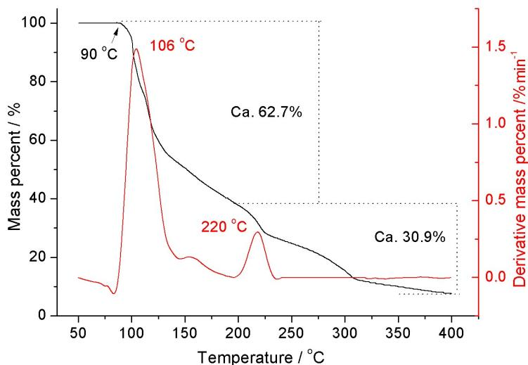
**Figure S3** TG and DTG curves of **2** under nitrogen with a heating rate of 5 °C min<sup>-1</sup>.
