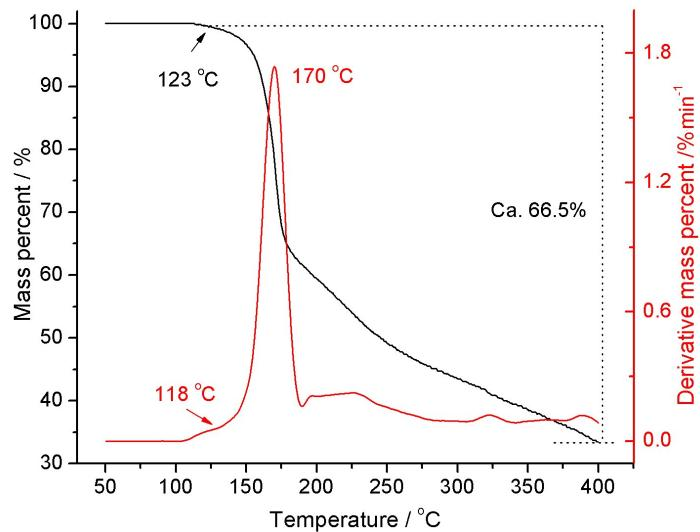
**Figure S11** TG and DTG curves of **10** under nitrogen with a heating rate of  $5\text{ }^{\circ}\text{C min}^{-1}$ .
