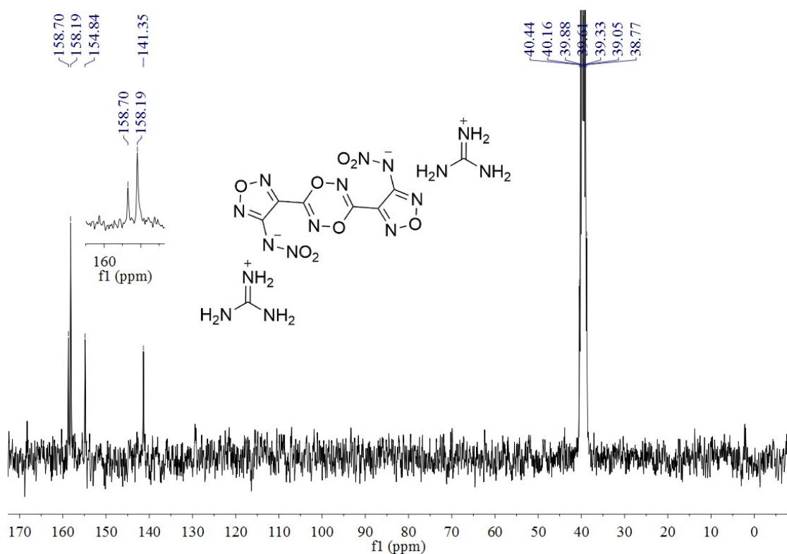
**Figure S33**  $^{13}\text{C}$ -NMR spectrum of **8** in  $d_6$ -DMSO.
