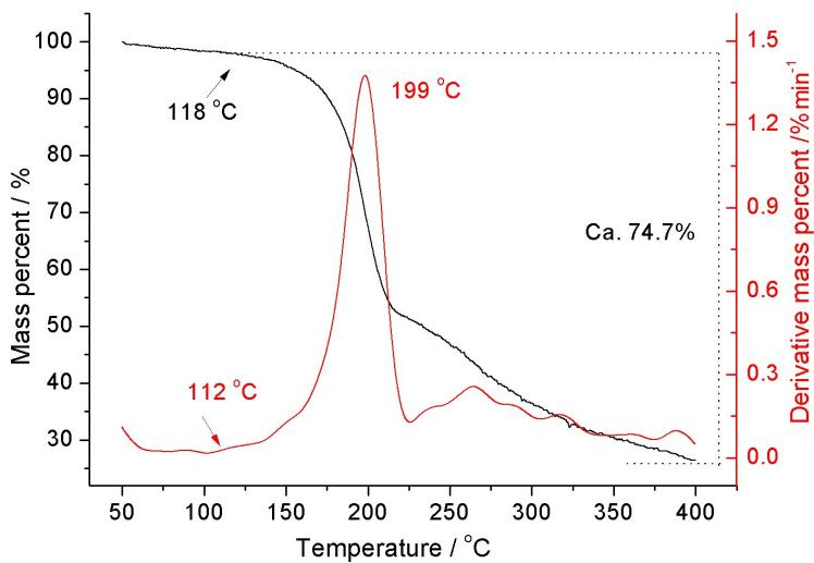
**Figure S12** TG and DTG curves of **11** under nitrogen with a heating rate of  $5\text{ }^{\circ}\text{C min}^{-1}$ .
