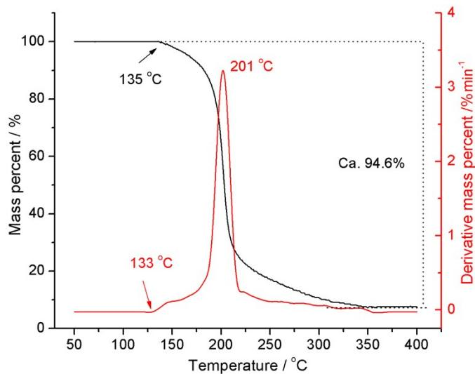
**Figure S2** TG and DTG curves of **1** under nitrogen with a heating rate of 5 °C min<sup>-1</sup>.
