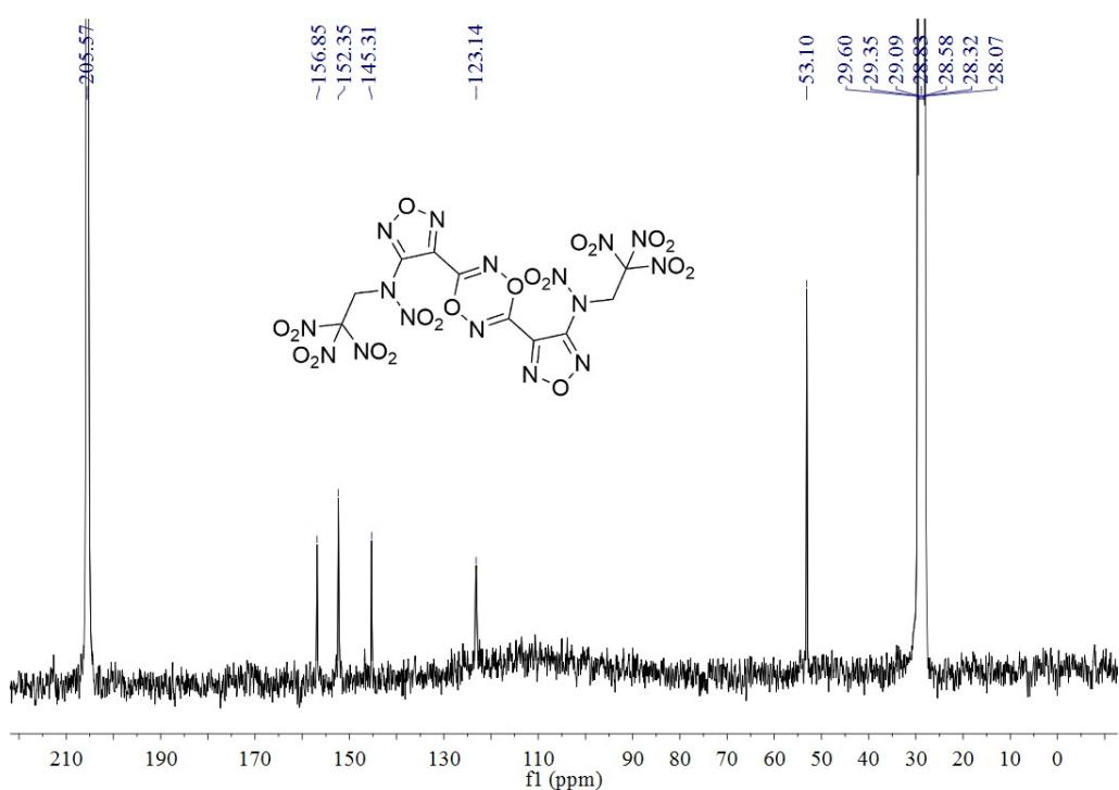
**Figure S21**  $^{13}\text{C}$ -NMR spectrum of **2** in  $d_6$ -Acetone.
