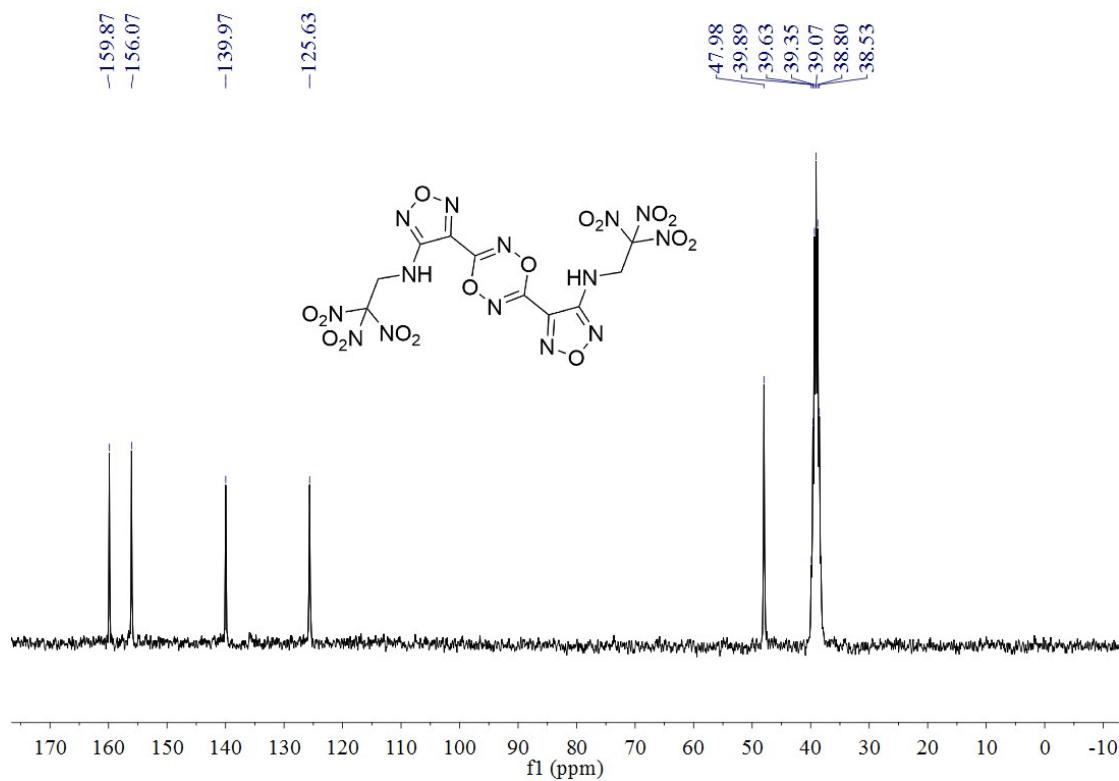
**Figure S19**  $^{13}\text{C}$ -NMR spectrum of **1** in  $d_6$ -DMSO.
