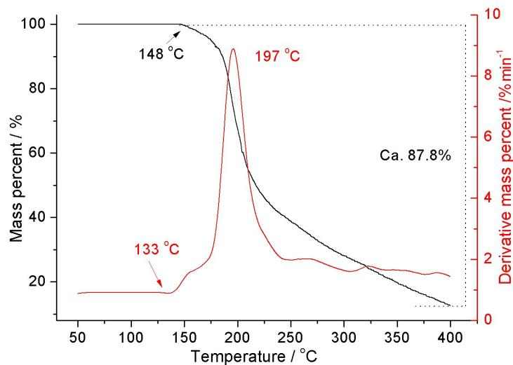
**Figure S9** TG and DTG curves of **8** under nitrogen with a heating rate of 5 °C min<sup>-1</sup>.
