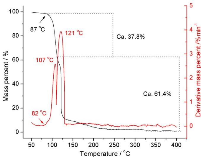
**Figure S4** TG and DTG curves of **3** under nitrogen with a heating rate of 5 °C min<sup>-1</sup>.
