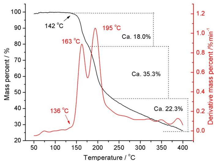
**Figure S8** TG and DTG curves of **7** under nitrogen with a heating rate of 5 °C min<sup>-1</sup>.
