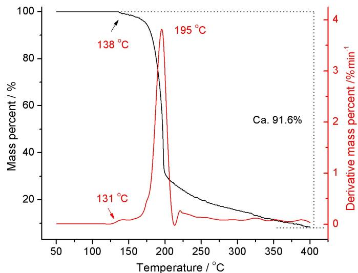
**Figure S6** TG and DTG curves of **5** under nitrogen with a heating rate of 5 °C min<sup>-1</sup>.
