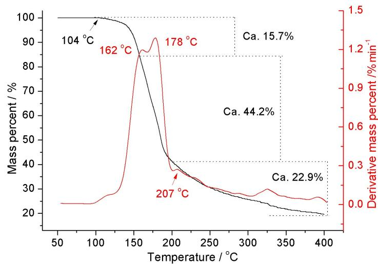
**Figure S5** TG and DTG curves of **4** under nitrogen with a heating rate of 5 °C min<sup>-1</sup>.
