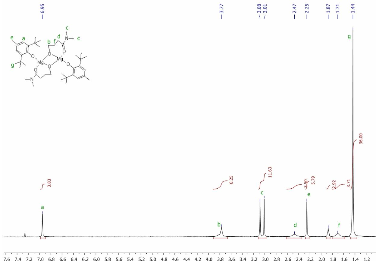
**Fig. S9.** <sup>1</sup>H NMR spectrum (400 MHz, CDCl<sub>3</sub>, 20 °C) of [(BHT)(O(CH<sub>2</sub>)<sub>3</sub>CONMe<sub>2</sub>)Mg]<sub>2</sub> (7)
