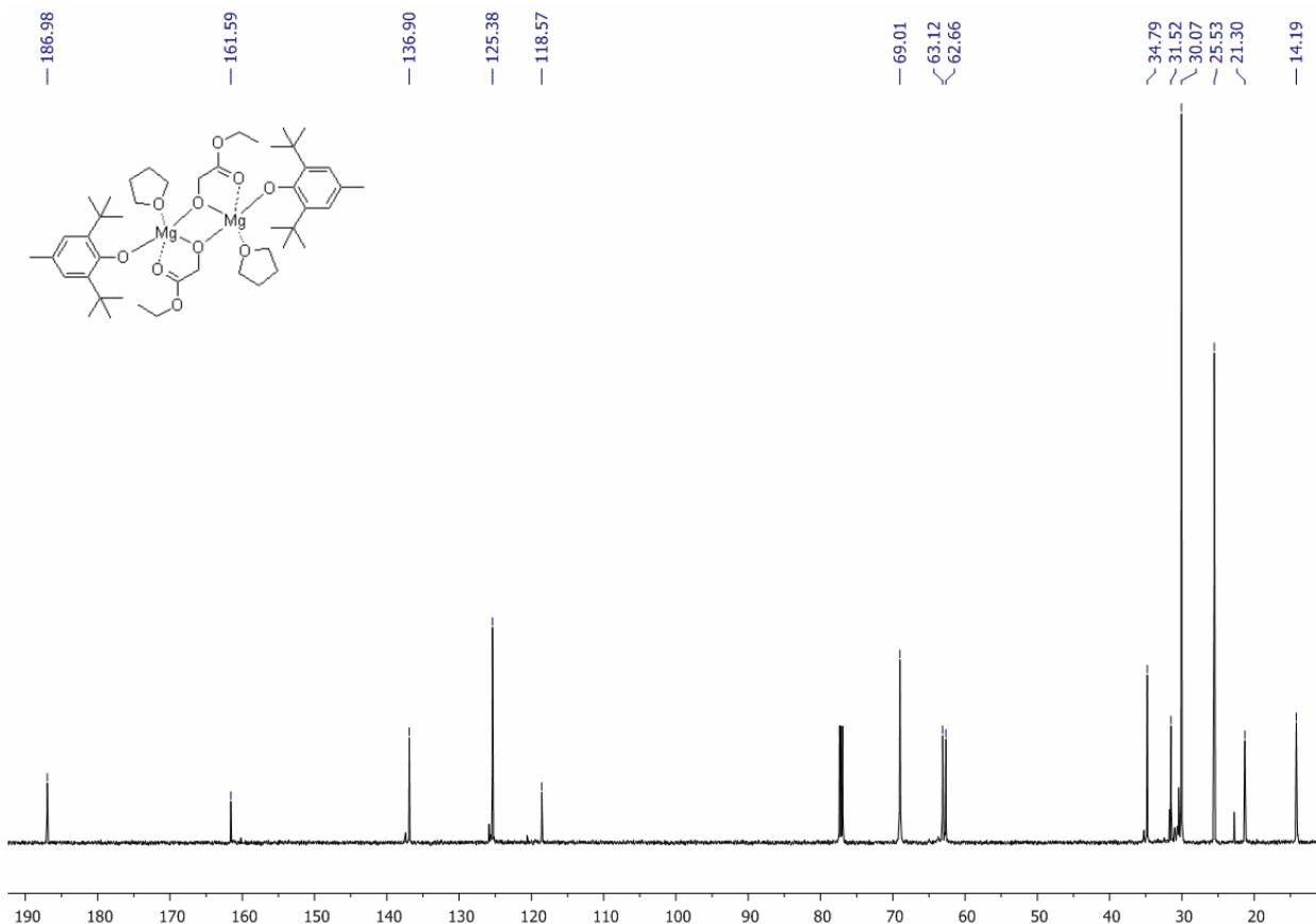
**Fig.S8.**  $^{13}\text{C}\{^1\text{H}\}$  NMR spectrum (151 MHz,  $\text{CDCl}_3$ , 20 °C) of  $[(\text{BHT})\text{Mg}(\mu\text{-OCH}_2\text{COOEt})(\text{THF})]_2$  (**5**)
