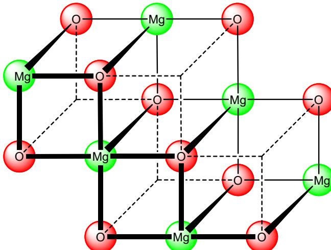
**Fig. S22.** An idealized  $\text{Mg}_6\text{O}_{10}$  tetracubic core of  $[\text{Mg}_6(\text{BHT})_2(\text{OCH}_2\text{COOEt})_{10}]$
