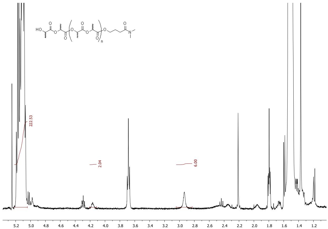
**Fig. S34.** <sup>1</sup>H NMR spectrum (400 MHz, CDCl<sub>3</sub>, 20 °C) of PLA obtained using complex 7 (Table 1, run 12)
