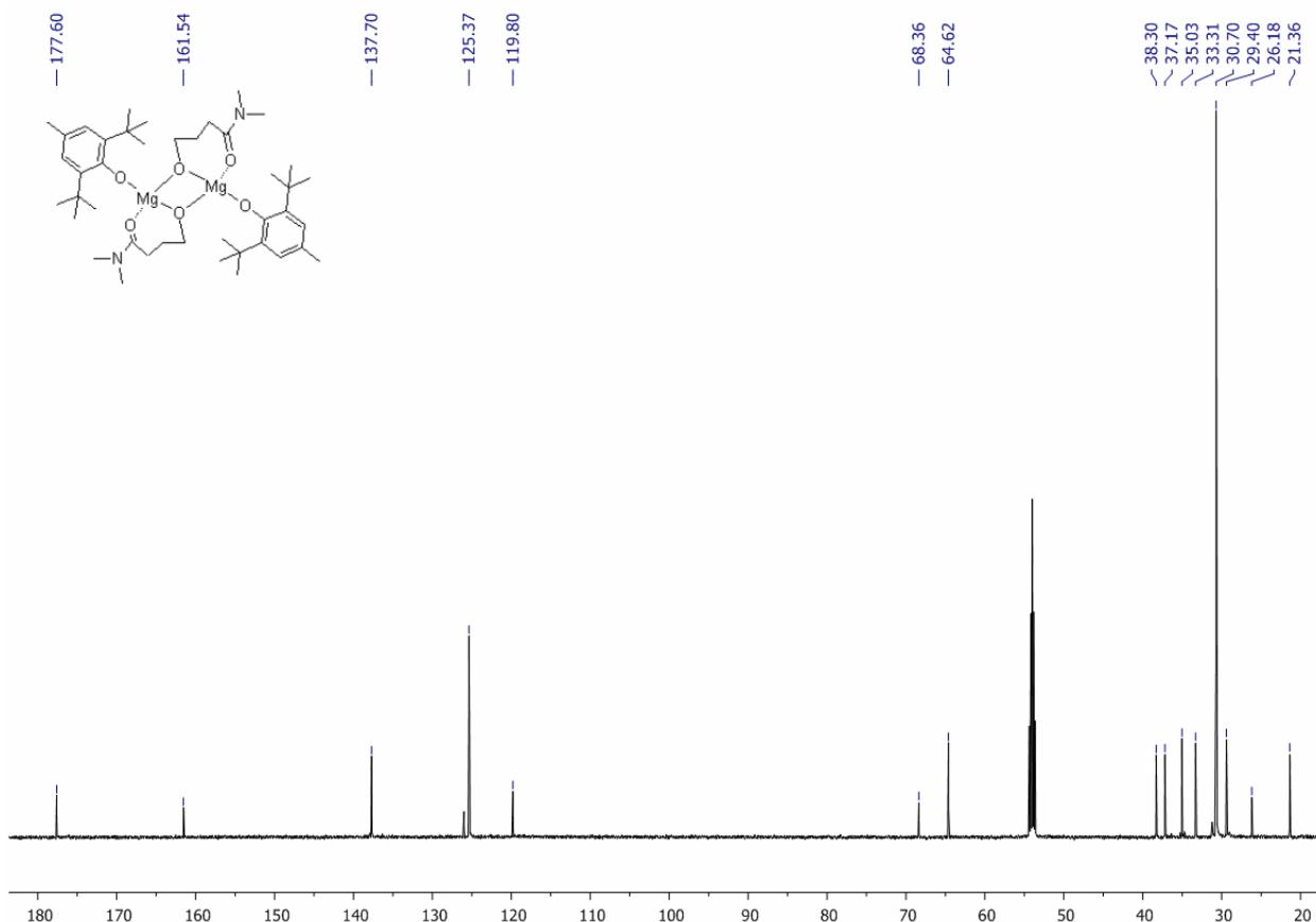
**Fig. S10.**  $^{13}\text{C}\{\text{H}\}$  NMR spectrum (151 MHz,  $\text{CD}_2\text{Cl}_2$ , 20 °C) of  $[(\text{BHT})(\text{O}(\text{CH}_2)_3\text{CONMe}_2)\text{Mg}]_2$  (**7**)
