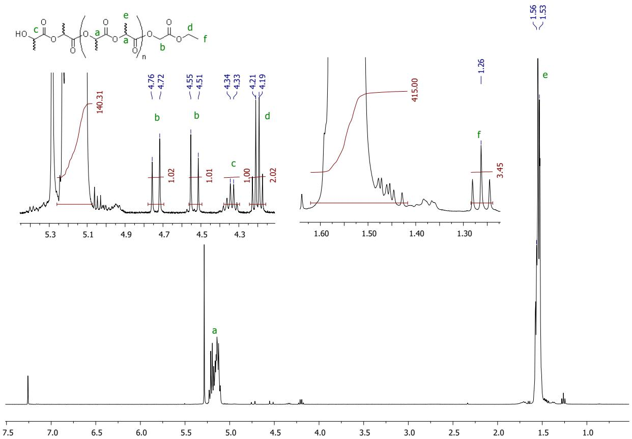
**Fig. S32.**  $^1\text{H}$  NMR spectrum (400 MHz,  $\text{CDCl}_3$ , 20 °C) of PLA obtained using complex 5 (Table 1, run 10)
