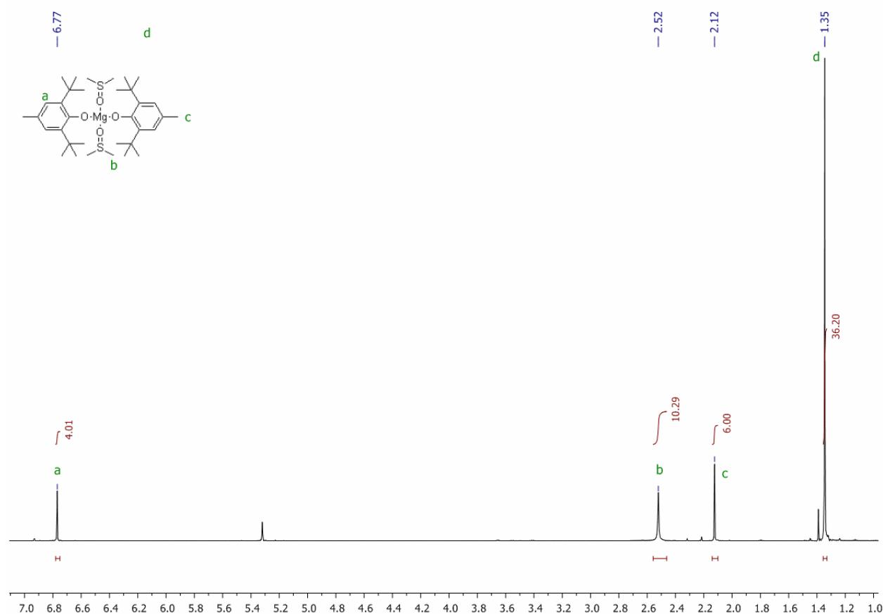
**Fig. S11.**  $^1\text{H}$  NMR spectrum (600 MHz,  $\text{CD}_2\text{Cl}_2$ , 20 °C) of  $(\text{BHT})_2\text{Mg}(\text{DMSO})_2$  (8)
