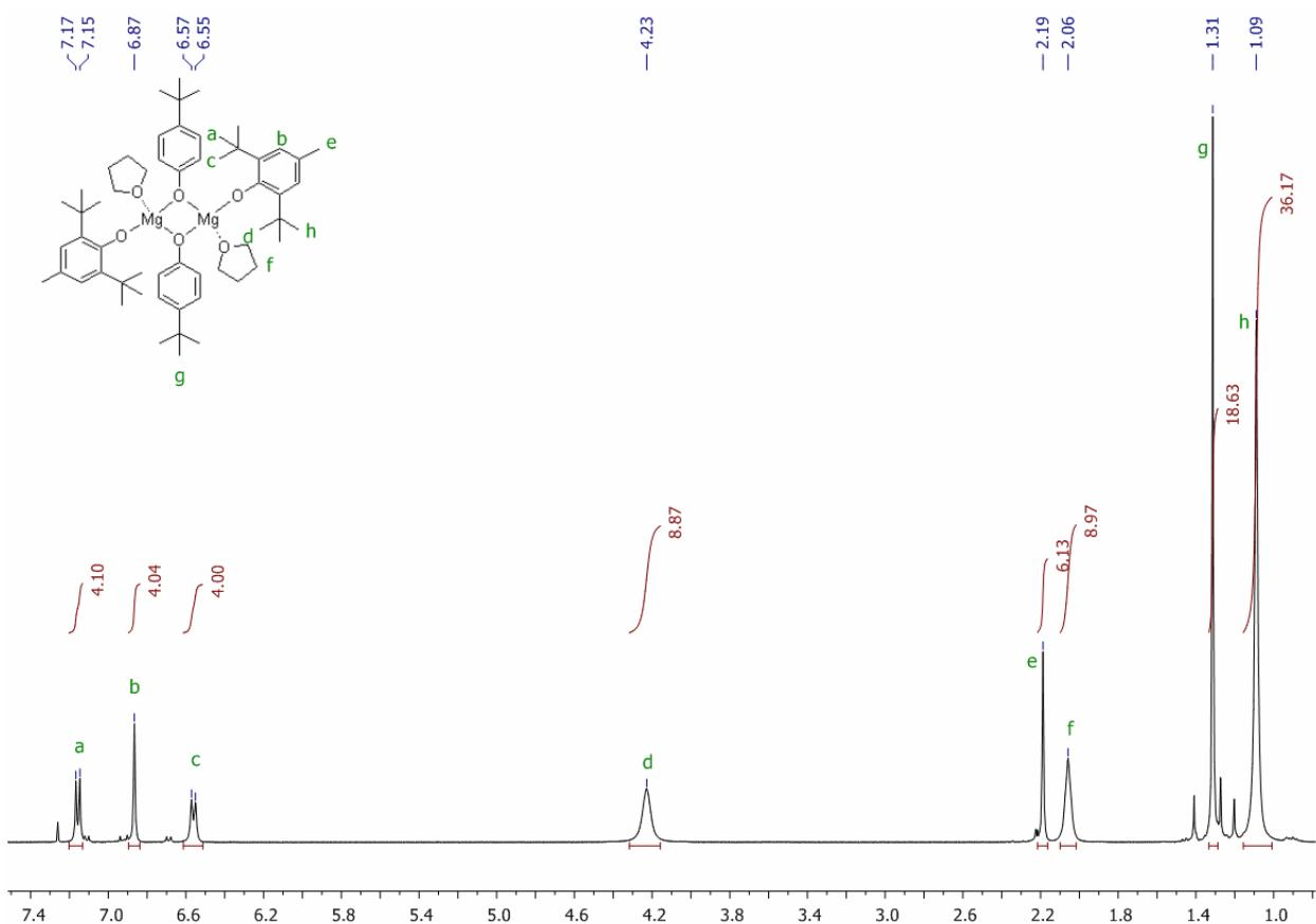
**Fig. S5.**  $^1\text{H}$  NMR spectrum (400 MHz,  $\text{CDCl}_3$ , 20 °C) of  $[(\text{BHT})\text{Mg}(\mu\text{-OC}_6\text{H}_4\text{-4-tBu})(\text{THF})]_2$  (**4**)
