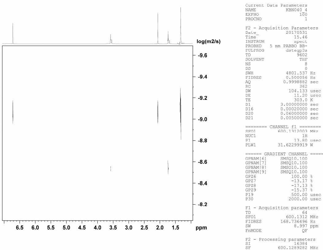
**Fig. S23.** DOSY NMR spectrum of  $(\text{BHT})_2\text{Mg}(\text{THF})_2$  (**1**) in  $\text{THFd}_8$  (600 Mhz, 303K)
