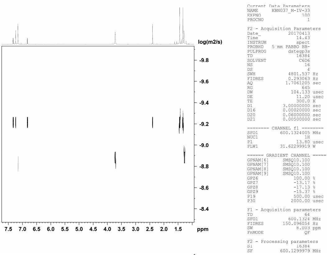
**Fig. S26.** DOSY NMR spectrum of  $[(\text{BHT})\text{Mg}(\text{OC}_6\text{H}_4\text{-}^t\text{Bu})(\text{thf})]_2$  (**4**) in  $\text{C}_6\text{D}_6$  (600 MHz, 303K)
