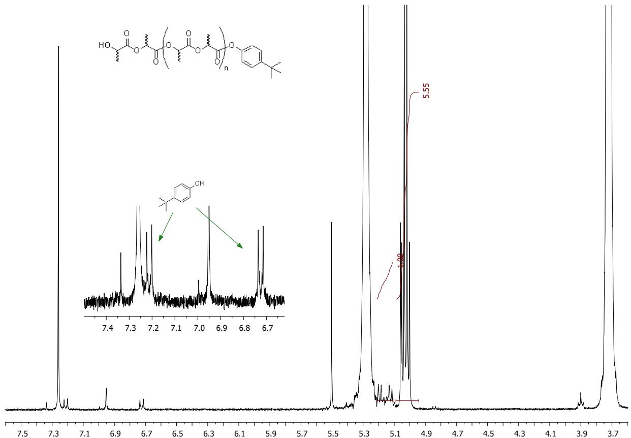
**Fig. S35.** <sup>1</sup>H NMR spectrum (400 MHz, CDCl<sub>3</sub>, 20 °C) of hydrolized and dried reaction mixture of rac-LA polymerization using complex 4 (Table 1, run 13)
