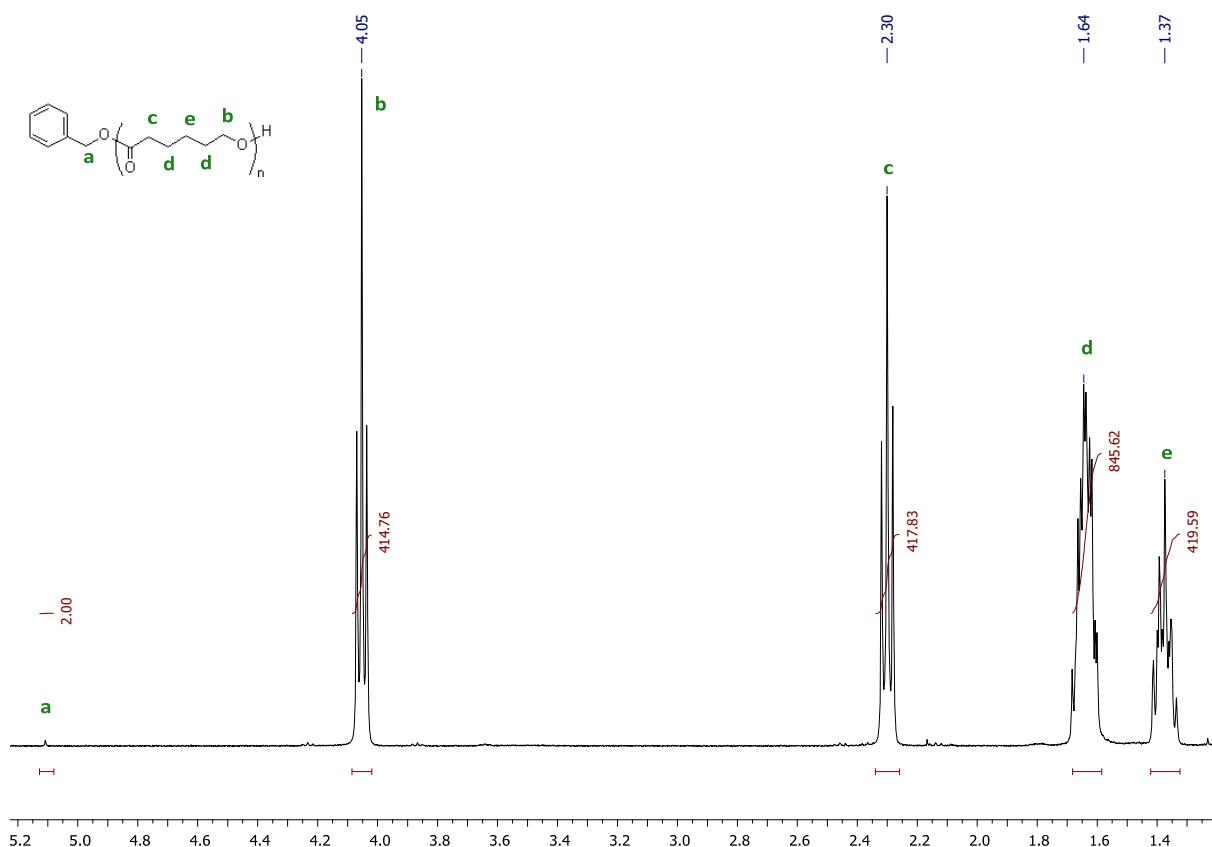
**Fig. S28.**  $^1\text{H}$  NMR spectrum (400 MHz,  $\text{CDCl}_3$ , 20 °C) of PCL obtained using complex 2 activated by  $\text{BnOH}$ ;  $[\varepsilon\text{CL}]/[2] = 200$  (Table 1, run 1)
