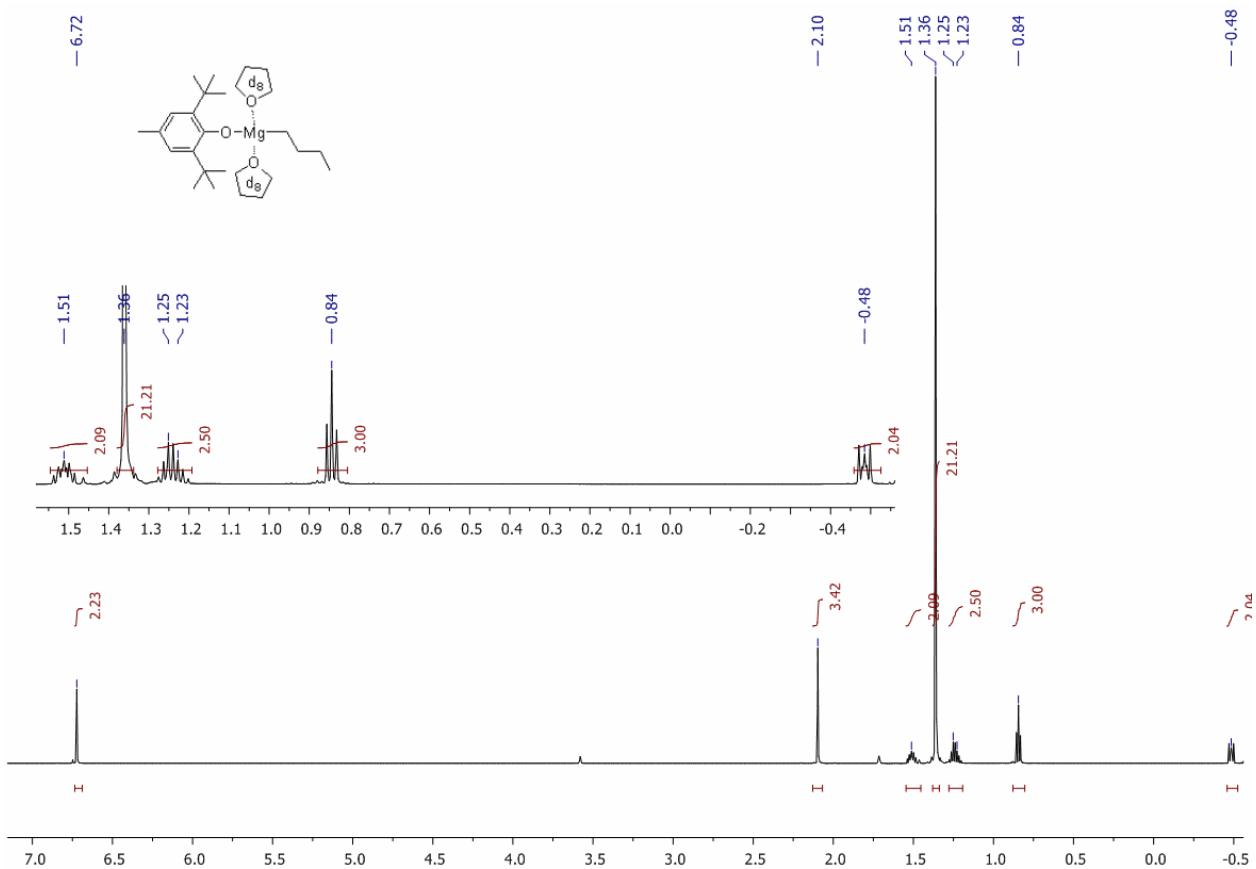
**Fig. S2.**  $^1\text{H}$  NMR spectrum (600 MHz, THF- $d_8$ , 20 °C) of [(BHT) $\text{Mg}(\text{n-Bu})_2$ ].
