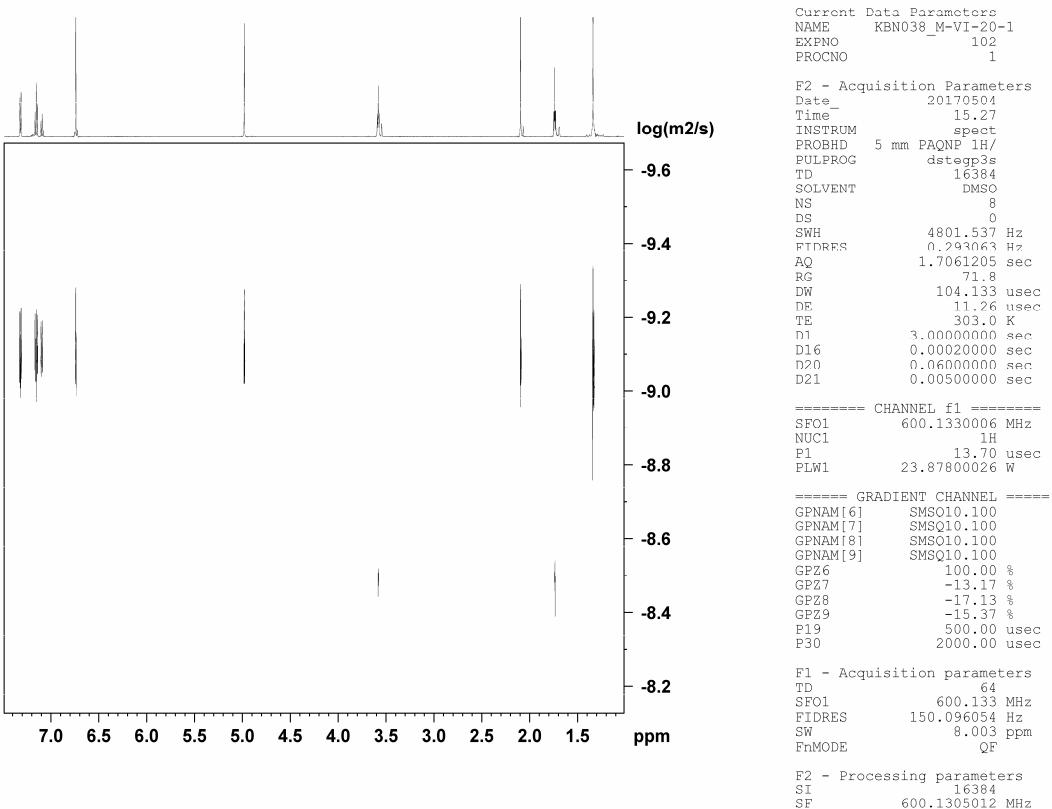
**Fig. S25.** DOSY NMR spectrum of [(BHT)Mg(Obn)(THF)]<sub>2</sub> (**3**) in THFd8 (600 MHz, 303K)
