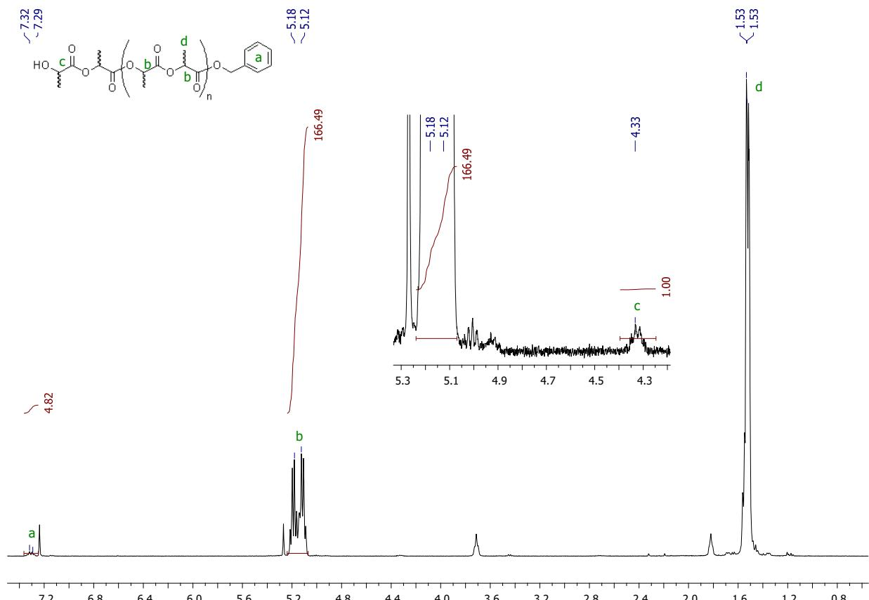
**Fig. S31.**  $^1\text{H}$  NMR spectrum (400 MHz,  $\text{CDCl}_3$ , 20 °C) of PLA obtained using complex **3** (Table 1, run 8)
