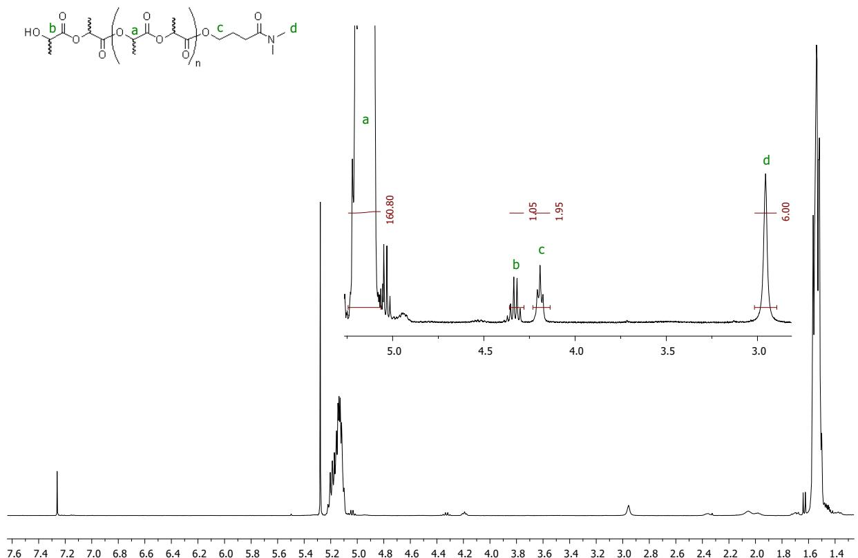
**Fig. S33.**  $^1\text{H}$  NMR spectrum (400 MHz,  $\text{CDCl}_3$ , 20 °C) of PLA obtained using complex 7 (Table 1, run 11)
