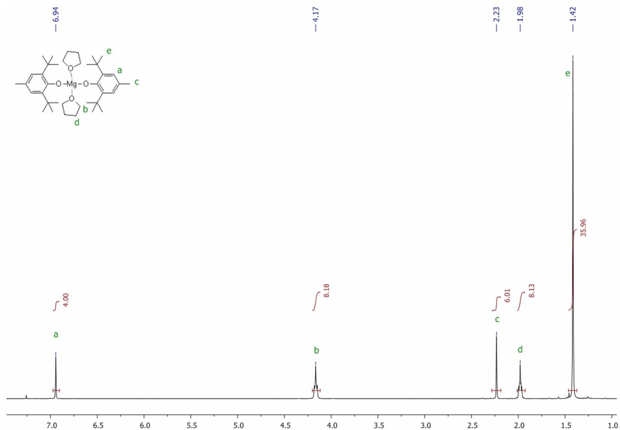
**Fig. S1.**  $^1\text{H}$  NMR spectrum (400 MHz,  $\text{CDCl}_3$ , 20 °C) of  $(\text{BHT})_2\text{Mg}(\text{THF})_2$  (**1**).
