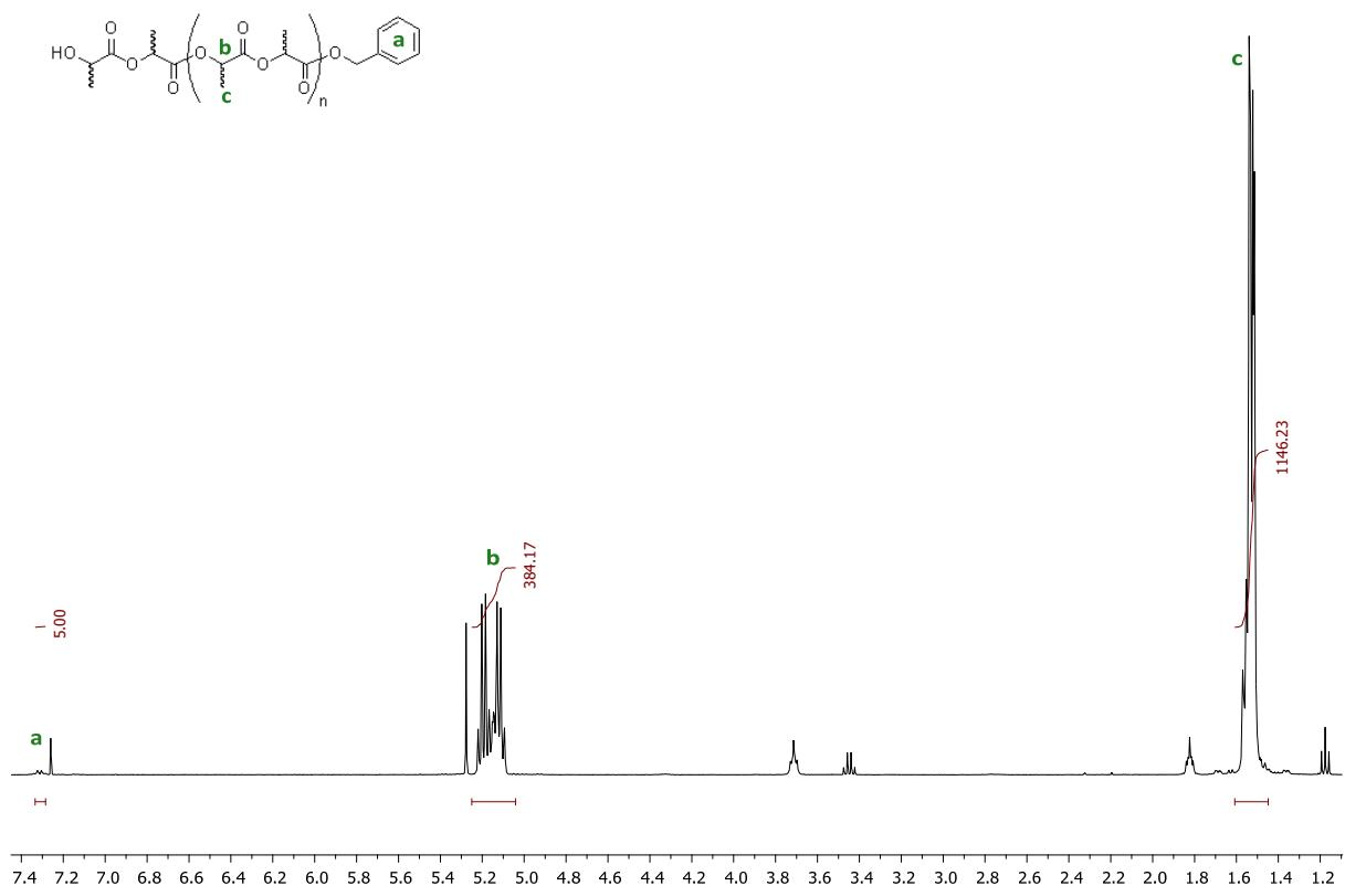
**Fig. S30.**  $^1\text{H}$  NMR spectrum (400 MHz,  $\text{CDCl}_3$ , 20 °C) of PLA obtained using complex **2** activated by  $\text{BnOH}$ ;  $[\text{LA}]/[2] = 200$  (Table 1, run 4)
