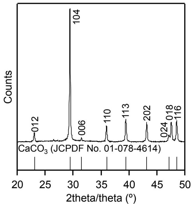
**Figure S1.** XRD pattern of the white precipitate obtained from saturated Ca(OH)<sub>2</sub> after through the gas evolved during the thermal decomposition of [Cu(ox)(dedap)<sub>2</sub>] under Ar flow.
