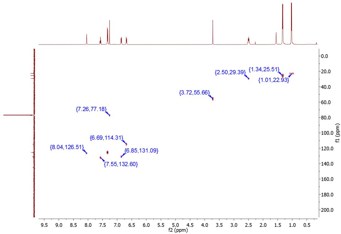
**Plot P12.**  $^1\text{H}$ - $^{13}\text{C}$  HMQC NMR spectrum of  $\{\text{IPr-(4-anisyl)}\}\text{Br}$  (**3d**).
