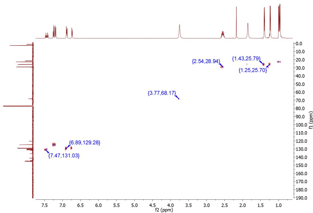
**Plot P53.**  $^1\text{H}$ - $^{13}\text{C}$  HMQC NMR spectrum of (aIPr<sup>4</sup>-tolyl)CuBr (**22**).
