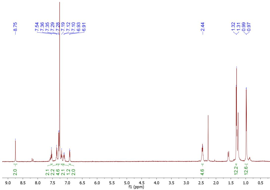
**Plot P27.**  $^1\text{H}$  NMR spectrum of (IPrPh)Cl (**4a**).
