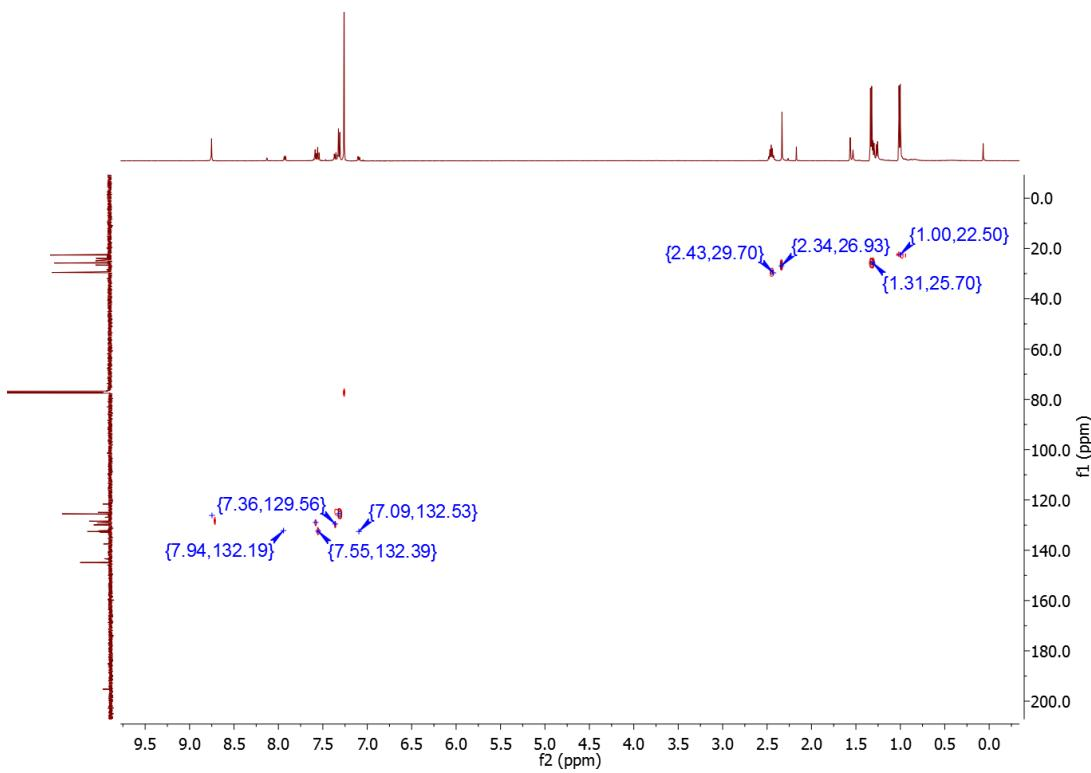
**Plot P20.**  $^1\text{H}$ - $^{13}\text{C}$  HMQC NMR spectrum of {IPr-(3-acetylphenyl)}Br (**3g**).
