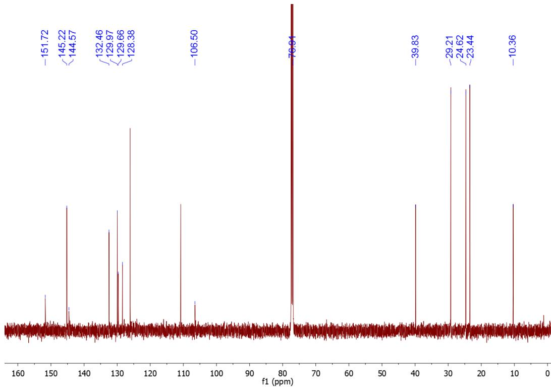
**Plot P49.**  $^{13}\text{C}\{^1\text{H}\}$  NMR spectrum of  $\{(\text{Me}_2\text{-IPr})\text{-}(4\text{-Me}_2\text{N-C}_6\text{H}_4)\}\text{Br}$  (**7c**).
