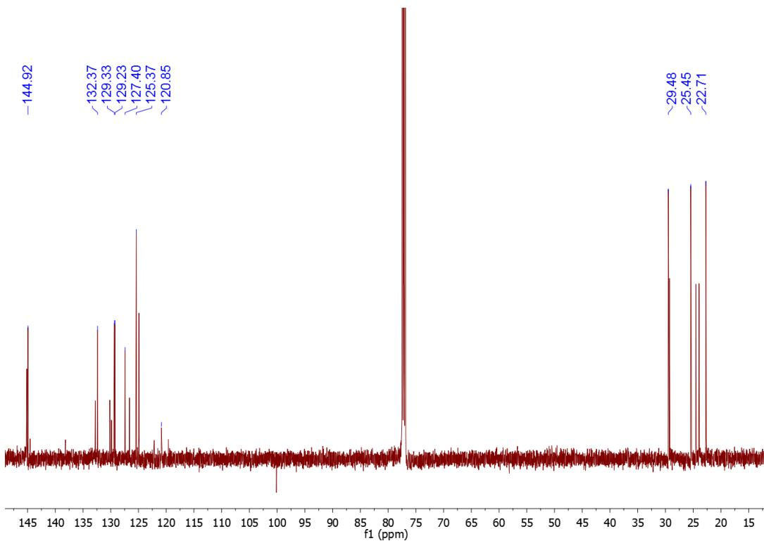
**Plot P34.**  $^{13}\text{C}\{\text{H}\}$  NMR spectrum of (IPrPh)OTf (**5**).
