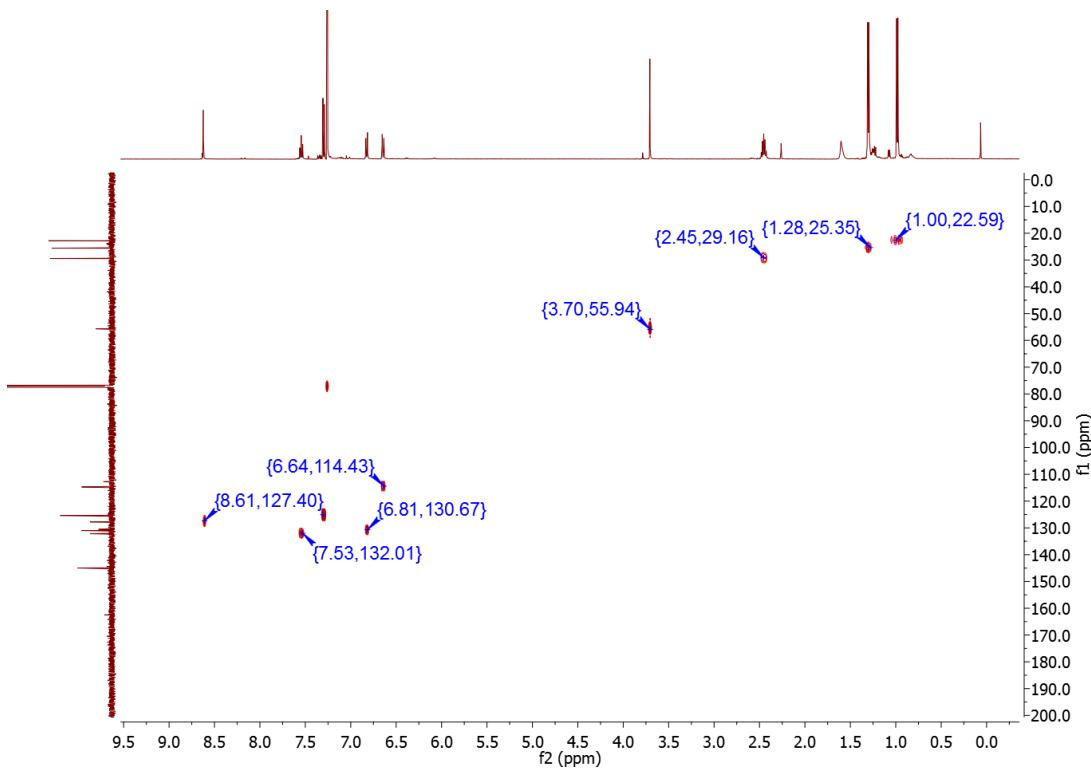
**Plot P32.**  $^1\text{H}-^{13}\text{C}$  HMQC NMR spectrum of  $\{\text{IPr-(4-anisyl)}\}\text{Cl}$  (**8**).
