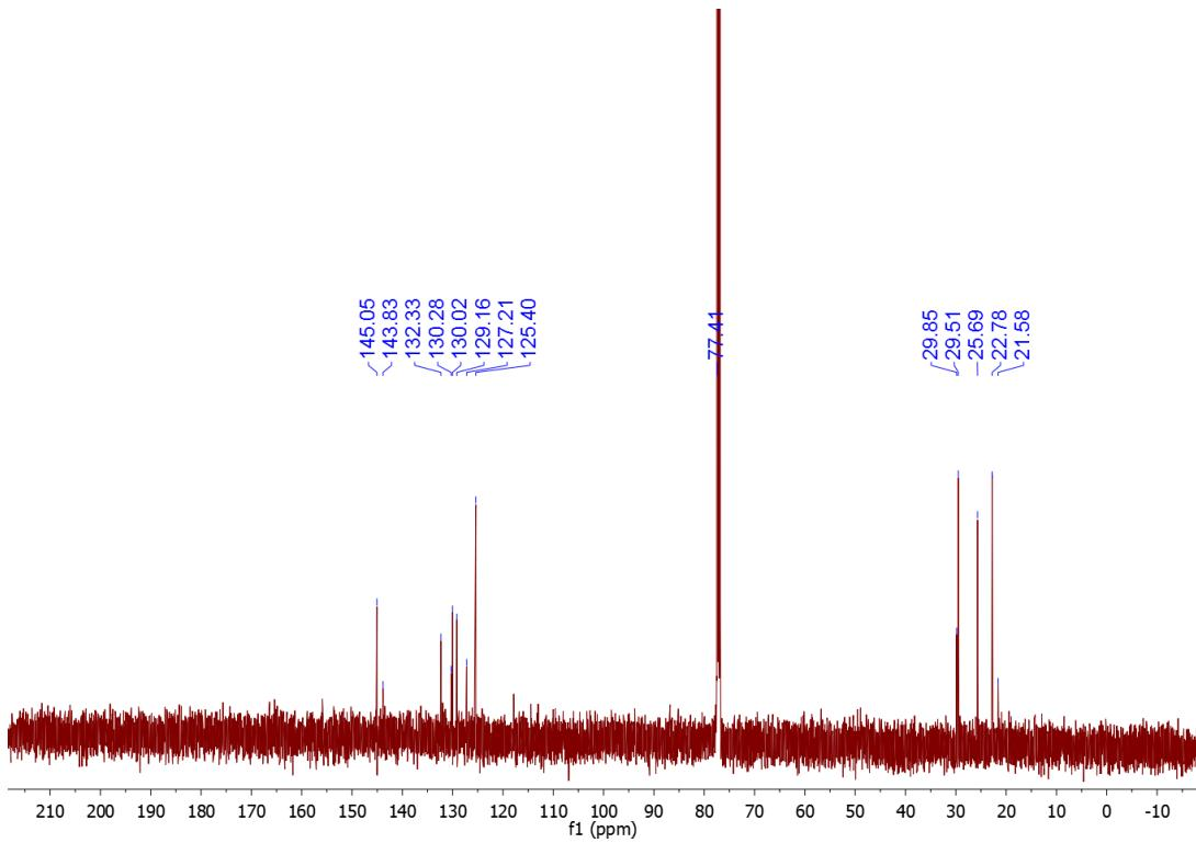
**Plot P5.**  $^{13}\text{C}\{\text{H}\}$  NMR spectrum of  $\{\text{IPr-(4-tolyl)}\}\text{Br}$  (**3b**).
