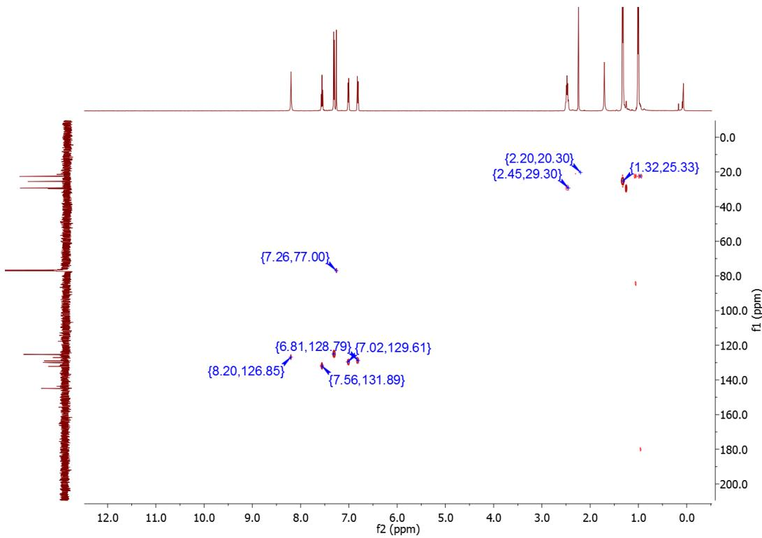
**Plot P6.**  $^1\text{H}-^{13}\text{C}$  HMQC NMR spectrum of  $\{\text{IPr-(4-tolyl)}\}\text{Br}$  (**3b**).
