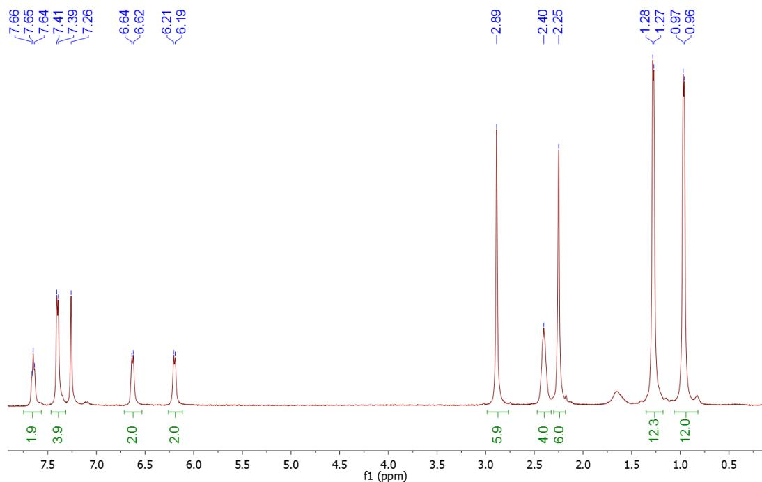
**Plot P48.**  $^1\text{H}$  NMR spectrum of  $\{\text{(Me}_2\text{-IPr)}\text{-(4-Me}_2\text{N-C}_6\text{H}_4\}\text{Br}$  (**7c**).
