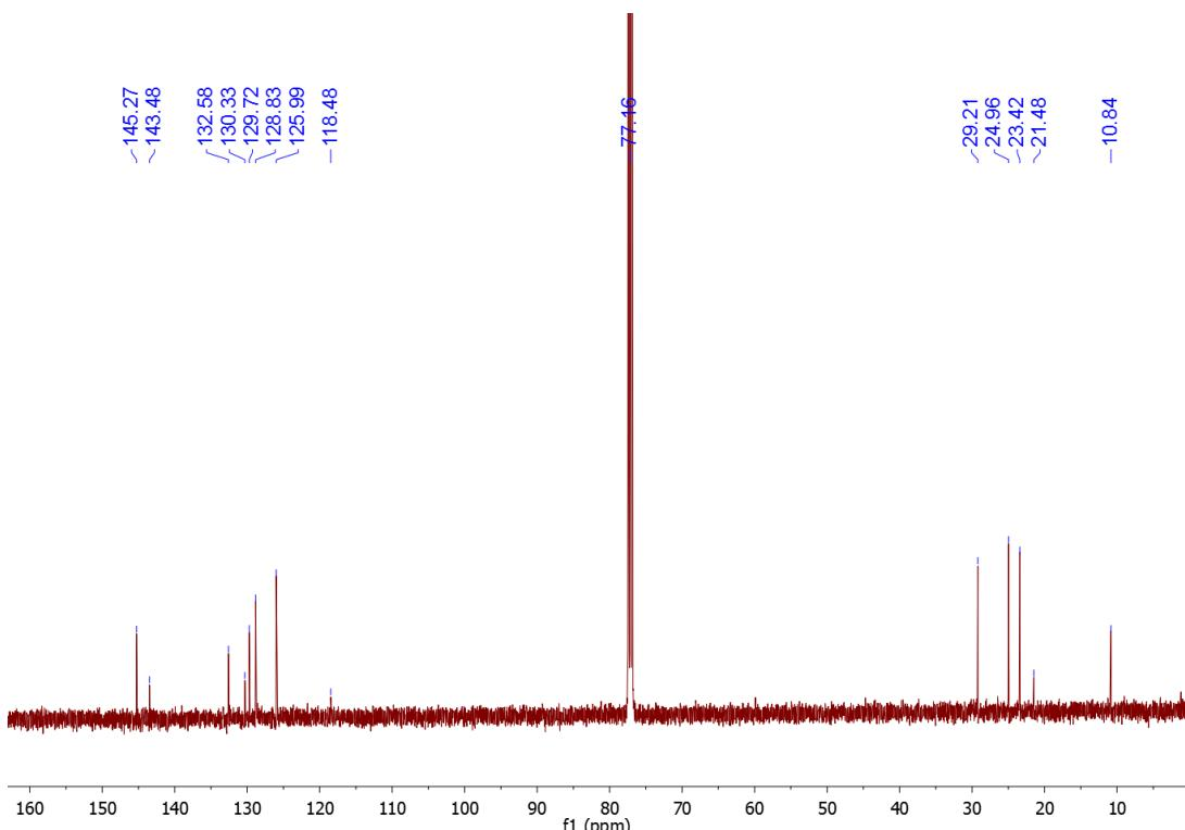
**Plot P46.**  $^{13}\text{C}\{\text{H}\}$  NMR spectrum of  $\{\text{Me}_2\text{-IPr}\text{-4-tolyl}\}\text{Br}$  (**7b**).
