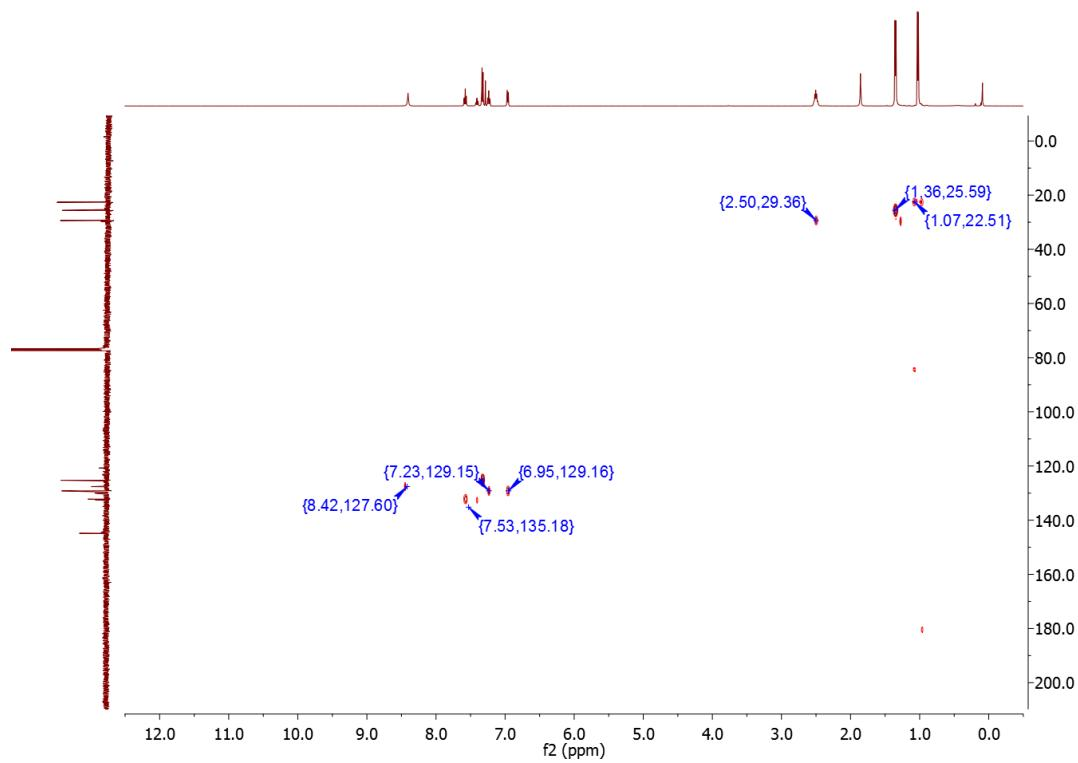
**Plot P3.**  $^1\text{H}$ - $^{13}\text{C}$  HMQC NMR spectrum of (IPrPh)Br (**3a**).
