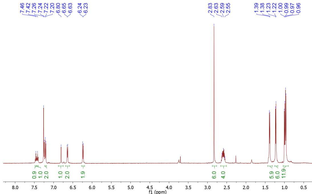
**Plot P54.**  $^1\text{H}$  NMR spectrum of {aIPr(4-Me<sub>2</sub>N-C<sub>6</sub>H<sub>4</sub>)}CuBr (**23**).
