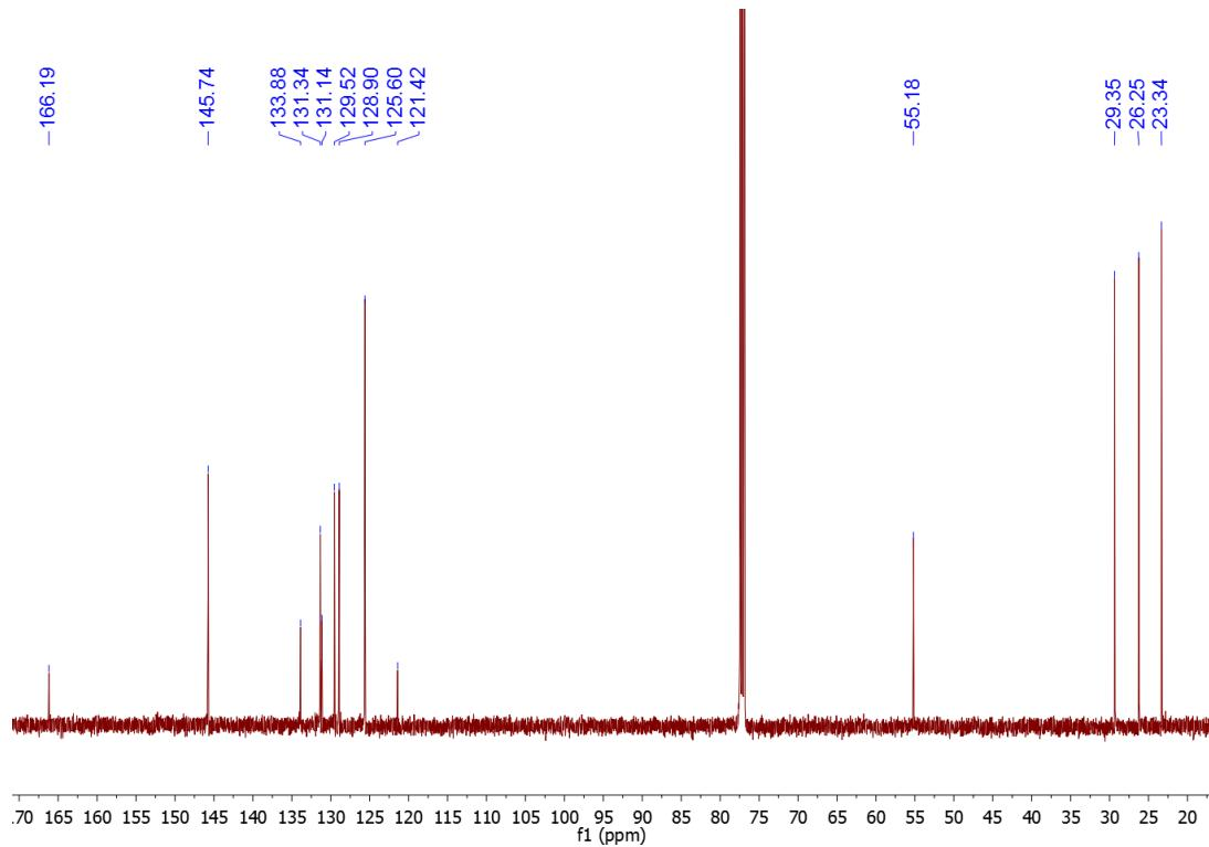
**Plot P37.**  $^{13}\text{C}\{\text{H}\}$  NMR spectrum of (SIPrPh)Br (6a).
