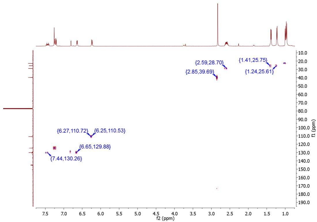
**Plot P56.**  $^1\text{H}$ - $^{13}\text{C}$  HMQC NMR spectrum of  $\{\text{aIPr}(4\text{-Me}_2\text{N-C}_6\text{H}_4)\text{CuBr}$  (**23**).
