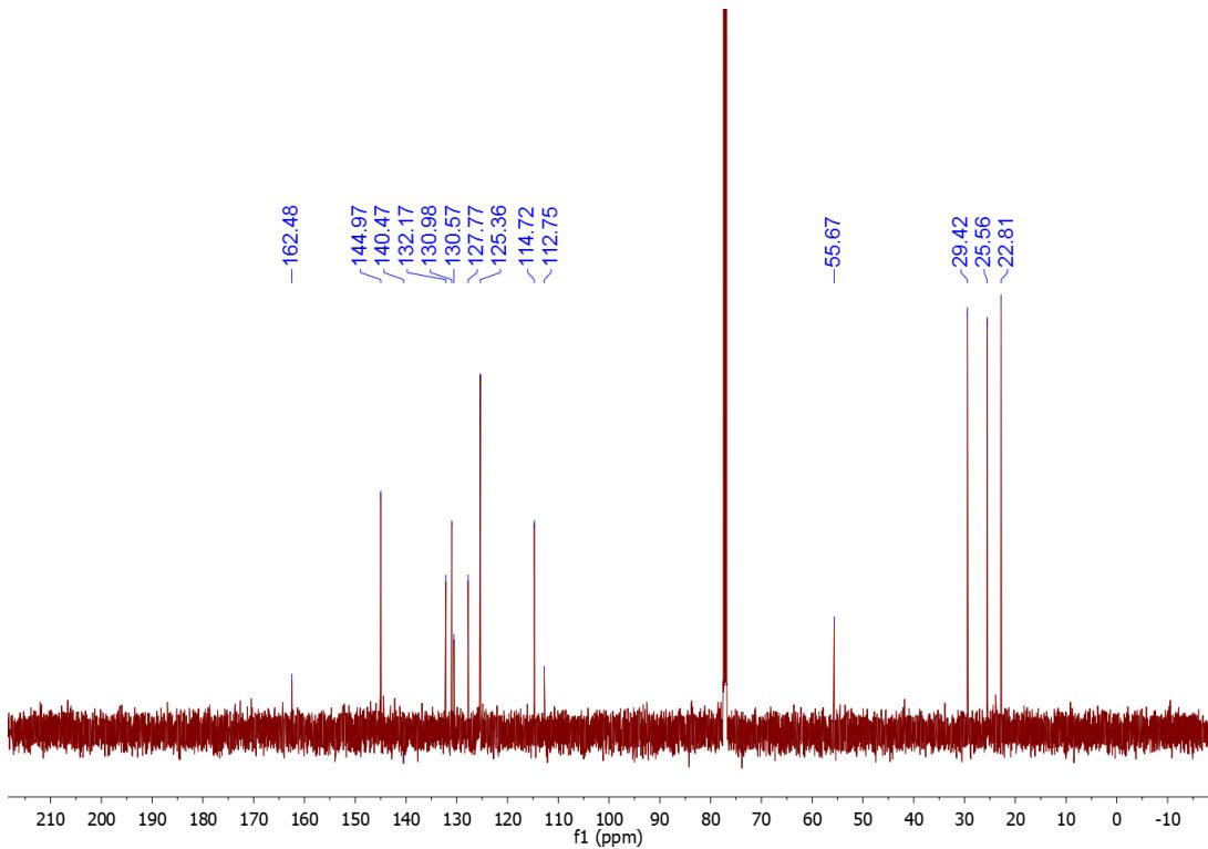
**Plot P31.**  $^{13}\text{C}\{\text{H}\}$  NMR spectrum of  $\{\text{IPr-(4-anisyl)}\}\text{Cl}$  (**8**).
