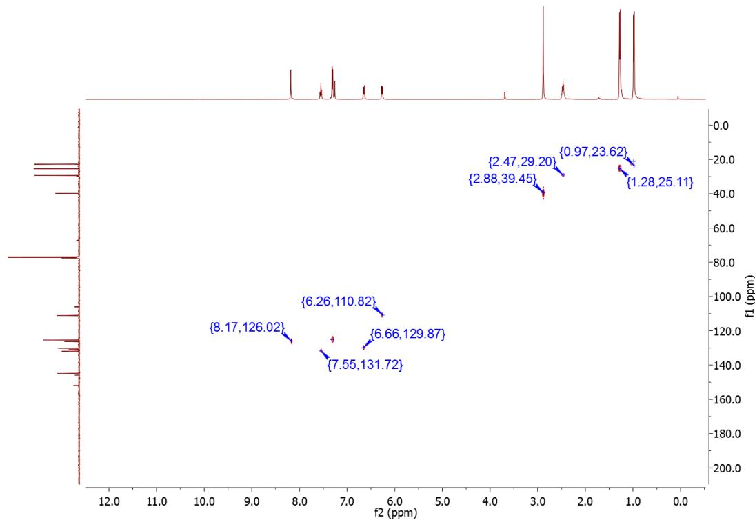
**Plot P26.**  $^1\text{H}$ - $^{13}\text{C}$  HMQC NMR spectrum of  $\{\text{IPr-(4-Me}_2\text{N-C}_6\text{H}_4\}\text{Br}$  (**3j**).
