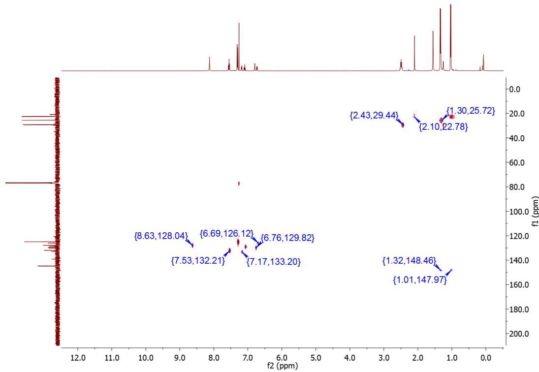
**Plot P9.**  $^1\text{H}$ - $^{13}\text{C}$  HMQC NMR spectrum of  $\{\text{IPr}-(3\text{-tolyl})\}\text{Br}$  (**3c**).
