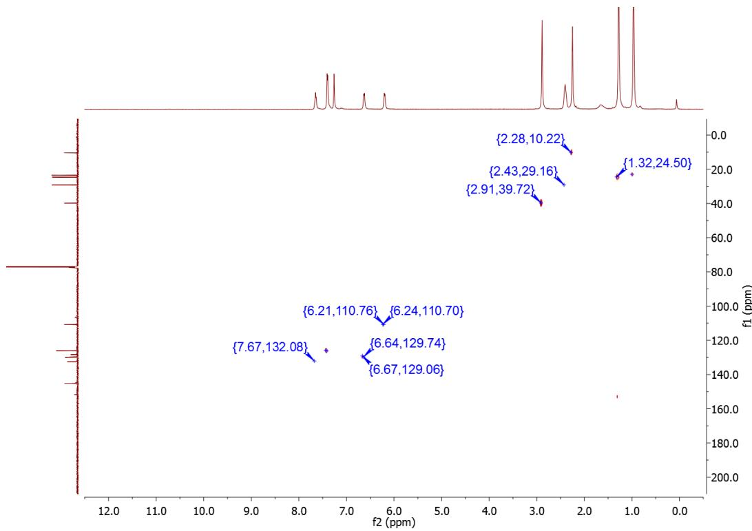
**Plot P50.**  $^1\text{H}$ - $^{13}\text{C}$  HMQC NMR spectrum of  $\{(\text{Me}_2\text{-IPr})\text{-}(4\text{-Me}_2\text{N-C}_6\text{H}_4)\}\text{Br}$  (**7c**).
