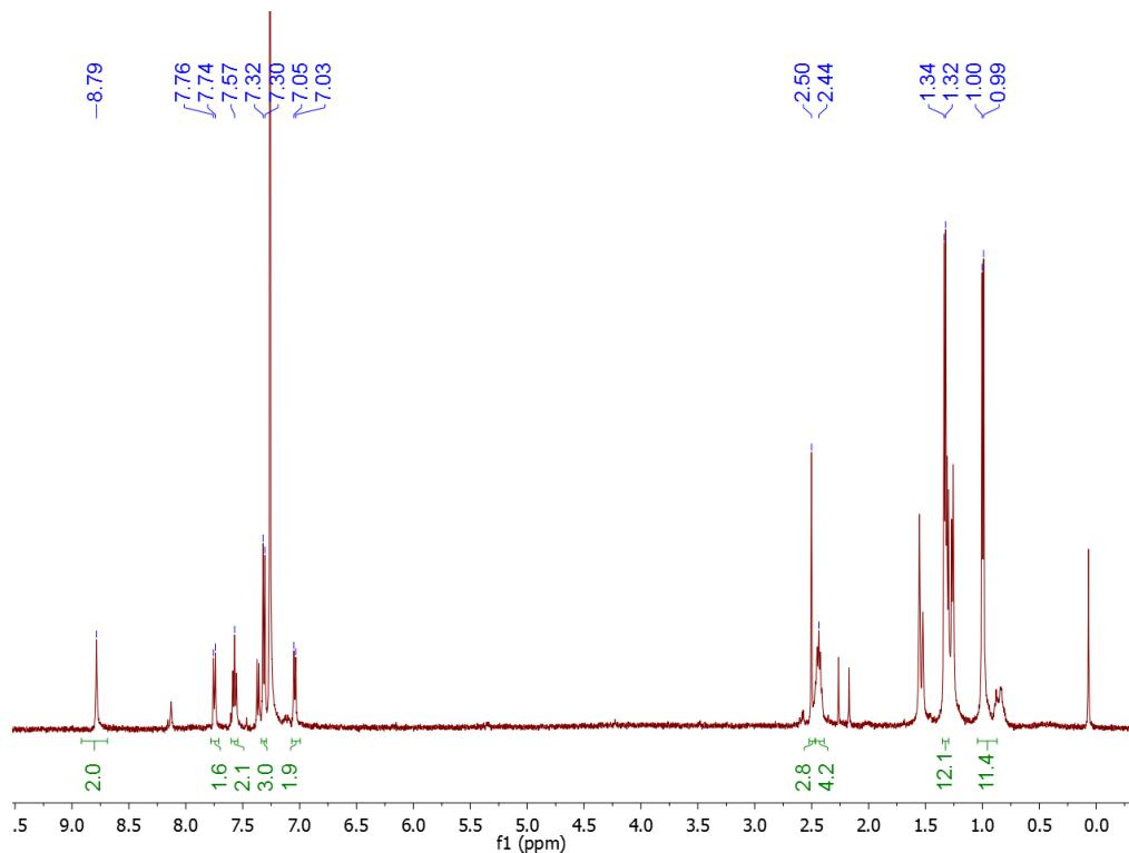
**Plot P16.**  $^1\text{H}$  NMR spectrum of {IPr-(4-acetylphenyl)}Br (**3f**).
