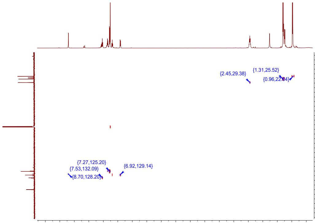
**Plot P29.**  $^1\text{H}$ - $^{13}\text{C}$  HMQC NMR spectrum of (IPrPh)Cl (**4**).
