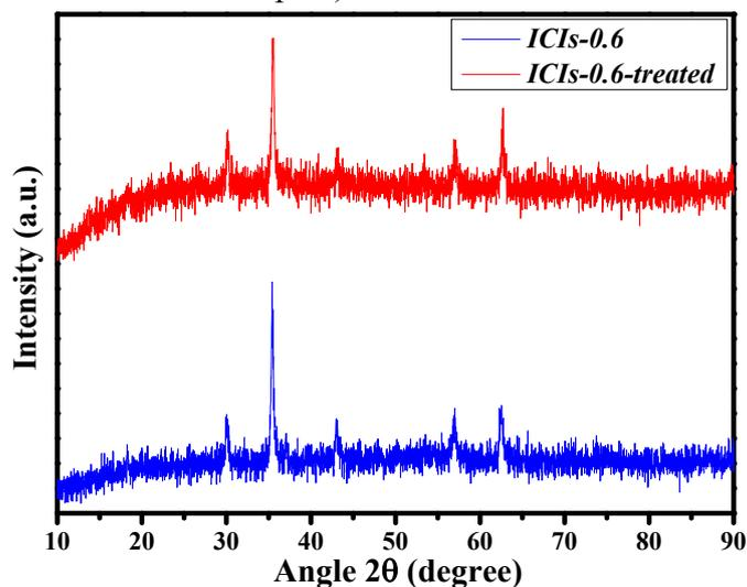
**Figure S4.** XRD patterns of ICIs-0.6 and ICIs-0.6 treated at 50 °C in air for 48 h.
