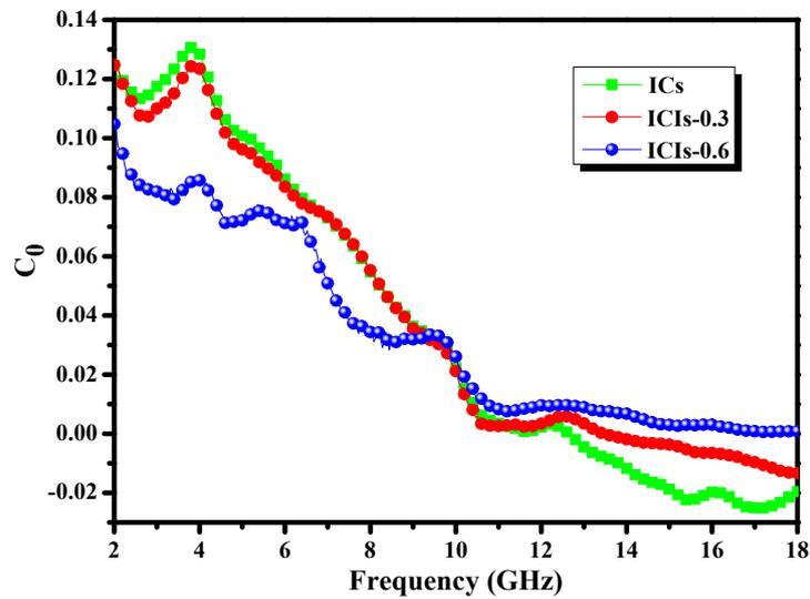
**Figure S9.** Eddy current loss of ICs, ICIs-0.3 and ICIs-0.6.
