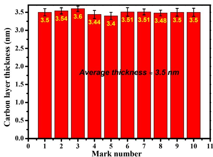
**Figure S2.** Carbon layer thickness statistics result. (Ten of the randomized nanospheres, each sphere with five measurement pots)
