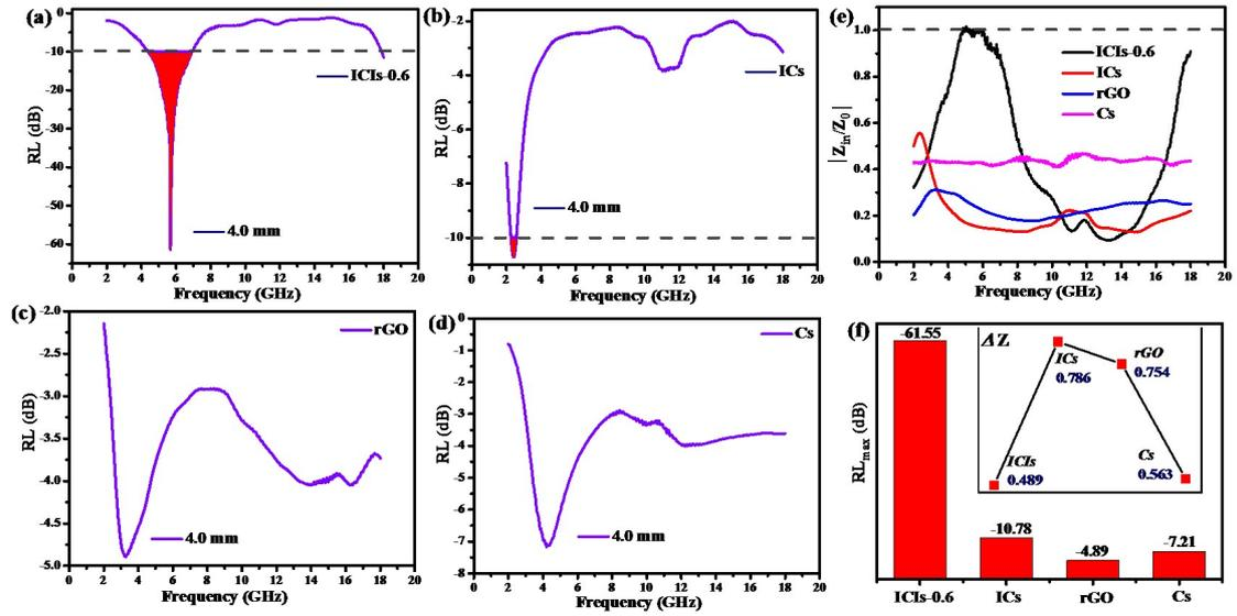
**Figure S8.** The calculated reflection loss of paraffin composites at 4.0 mm; (a) ICIs-0.6, (b) ICs, (c) rGO, (d) Cs. The modulus of normalized input impedance  $|Z_{in}/Z_0|$  (e) and the maximum RL values (f) for ICIs-0.6, ICs, rGO and Cs at 4.0 mm. Inset shows the proposed ACIM value ( $\Delta Z$ ) of the four samples.
