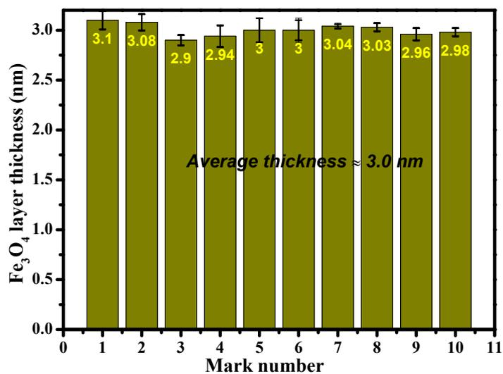
**Figure S3.** Fe<sub>3</sub>O<sub>4</sub> layer thickness statistics result. (Ten of the randomized nanospheres,
