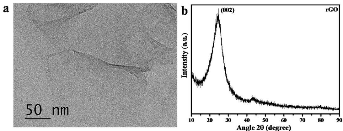
**Figure S1.** The TEM image (a) and XRD pattern (b) of prepared rGO.
