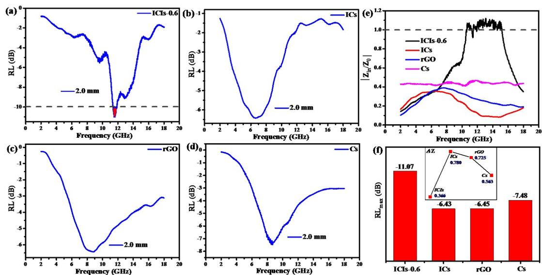
**Figure S5.** The calculated reflection loss of paraffin composites at 2.0 mm; (a) ICIs-0.6, (b) ICs, (c) rGO, (d) Cs. The modulus of normalized input impedance  $|Z_{in}/Z_0|$  (e) and the maximum RL values (f) for ICIs-0.6, ICs, rGO and Cs at 2.0 mm. Inset shows the proposed ACIM value ( $\Delta Z$ ) of the four samples.
