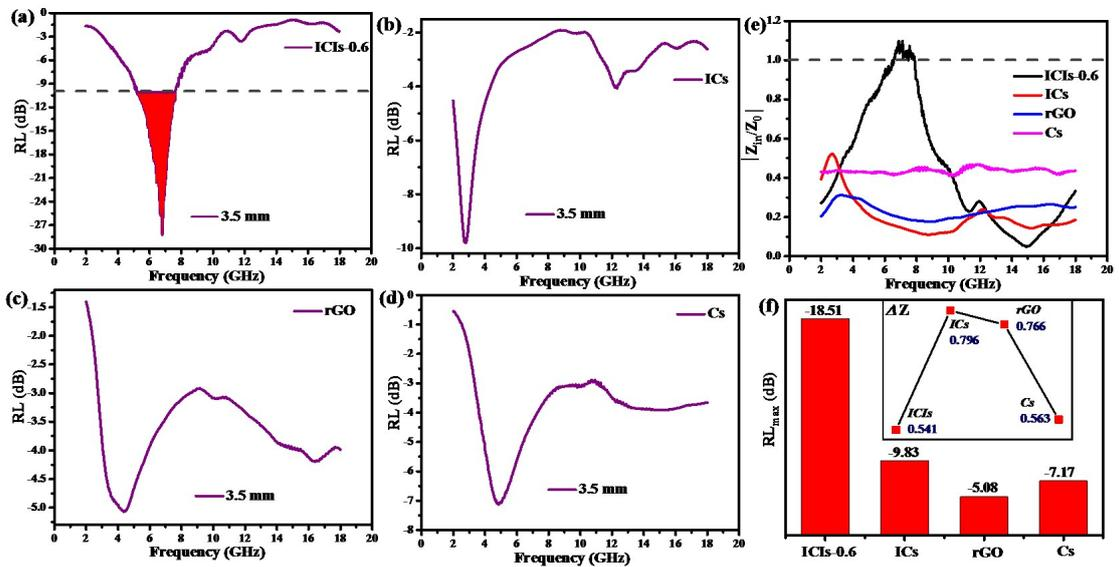
**Figure S7.** The calculated reflection loss of paraffin composites at 3.5 mm; (a) ICIs-0.6, (b) ICs, (c) rGO, (d) Cs. The modulus of normalized input impedance  $|Z_{in}/Z_0|$  (e) and the maximum RL values (f) for ICIs-0.6, ICs, rGO and Cs at 3.5 mm. Inset shows the proposed ACIM value ( $\Delta Z$ ) of the four samples.
