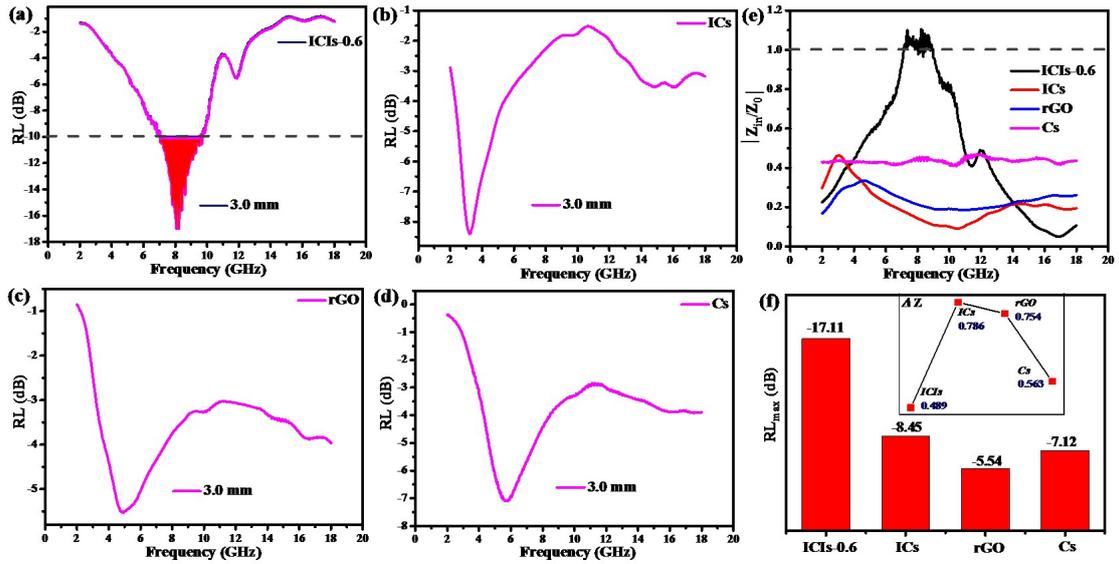
**Figure S6.** The calculated reflection loss of paraffin composites at 3.0 mm; (a) ICIs-0.6, (b) ICs, (c) rGO, (d) Cs. The modulus of normalized input impedance  $|Z_{in}/Z_0|$  (e) and the maximum RL values (f) for ICIs-0.6, ICs, rGO and Cs at 3.0 mm. Inset shows the proposed ACIM value ( $\Delta Z$ ) of the four samples.
