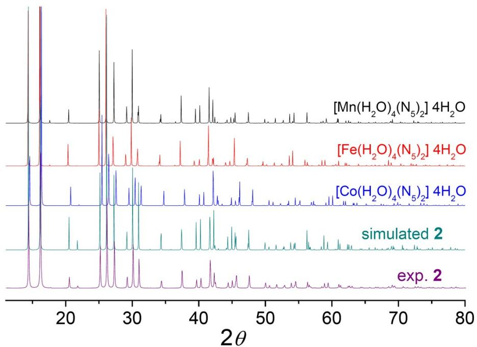
**Fig. S4** Powder X-ray diffraction pattern of complex **2** (purple). The patterns in black ( $[\text{Mn}(\text{H}_2\text{O})_4(\text{N}_5)_2]\cdot 4\text{H}_2\text{O}$ ), red ( $[\text{Fe}(\text{H}_2\text{O})_4(\text{N}_5)_2]\cdot 4\text{H}_2\text{O}$ ), blue ( $[\text{Co}(\text{H}_2\text{O})_4(\text{N}_5)_2]\cdot 4\text{H}_2\text{O}$ ), and dark green (**2**) are the calculated patterns from their single crystal structures.
