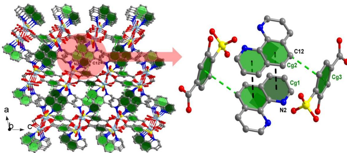
**Fig. S8** 3-D supramolecular network of complex **6-La**. The  $\pi\cdots\pi$  and C-H $\cdots\pi$  interactions were denoted as black and green dashed lines.
