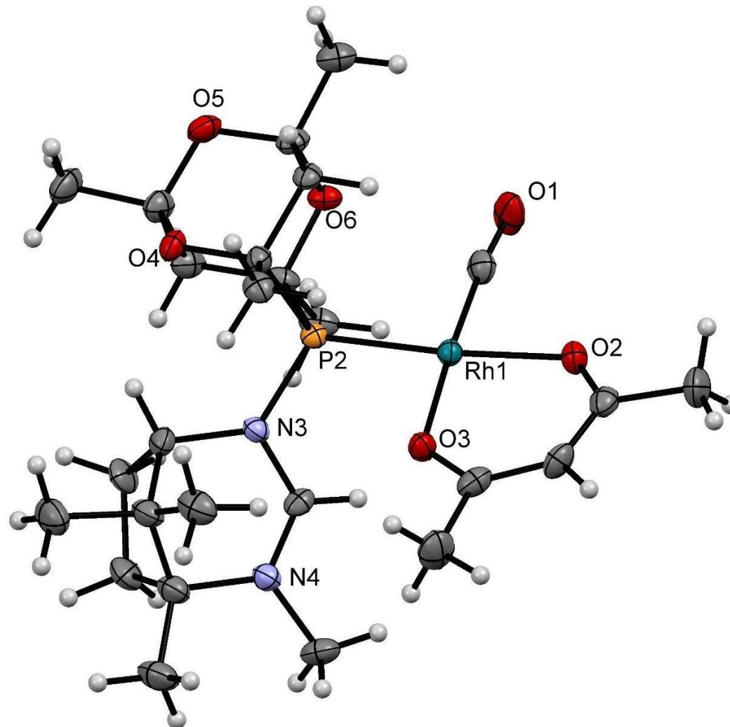
Thermal ellipsoid plot (ellipsoids drawn at 50% probability) of  $[\text{Rh}(\alpha,\beta\text{-CgPAmH})(\text{CO})\text{Cl}_2]$ . One of two diastereomers in the asymmetric unit.
