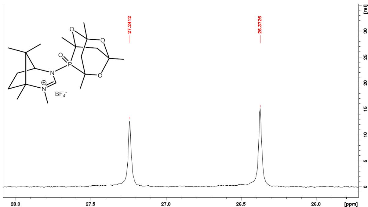
$^1\text{H}$  NMR spectrum of  $[\alpha,\beta\text{-CgP(O)AmMe}]BF_4$  recorded at 400 MHz in  $\text{CD}_3\text{CN}$ .
