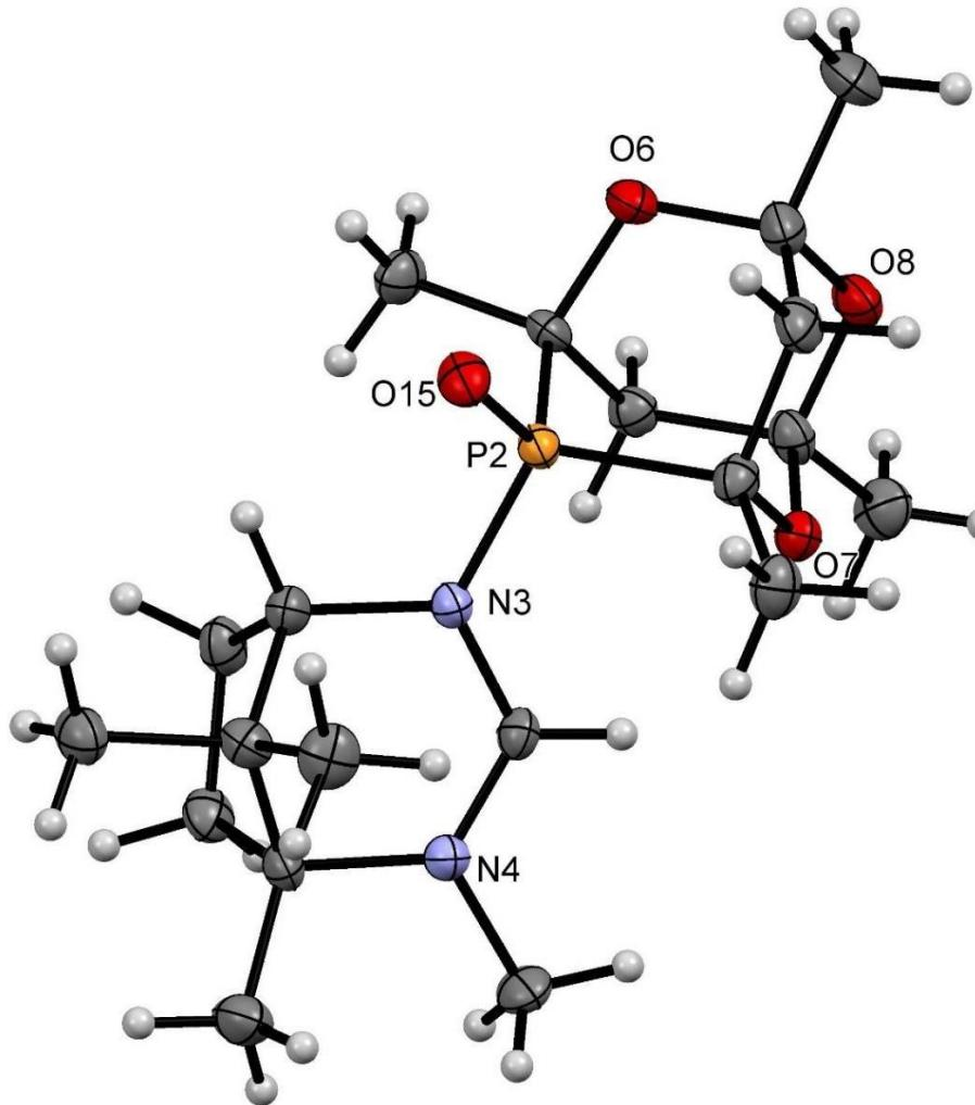
Thermal ellipsoid plot (ellipsoids drawn at 50% probability) of  $[\text{Rh}(\alpha,\beta\text{-CgPAm})(\text{acac})(\text{CO})]\text{BF}_4\text{PAmMe}\text{BF}_4$ . One of two diastereomers in the asymmetric unit with  $\text{BF}_4^-$  counterion and  $\text{CH}_2\text{Cl}_2$  solvate molecule omitted for clarity.
