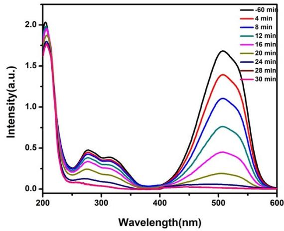
**Fig.S2.** UV-Vis spectral changes during the photodegradation of MO mediated by  $\text{SiW}_{12}/\text{C}_3\text{N}_4\text{-3}$  under visible light irradiation.
