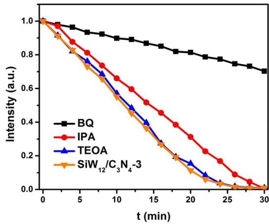
**Fig.S3** Photocatalytic degradation of MO over  $\text{SiW}_{12}/\text{C}_3\text{N}_4\text{-3}$ , photocatalyst alone and with the addition of IPA or BQ and TEOA.
