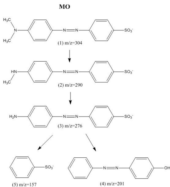
**Fig. S11.** Proposed degradation pathway of aqueous MO in the visible-light irradiating  $\text{SiW}_{12}/\text{g-C}_3\text{N}_4$  system.
