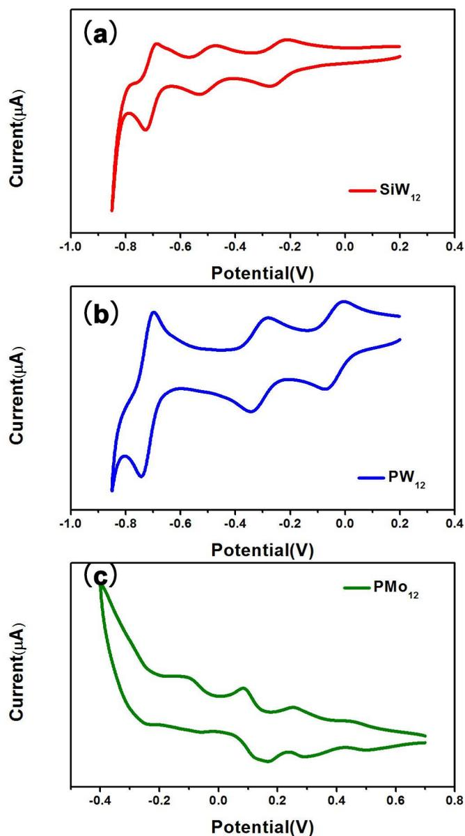
**Fig.S7.** The CV curves of Keggin POMs (a)  $\text{SiW}_{12}$ , (b)  $\text{PW}_{12}$  and (c)  $\text{PMo}_{12}$ . Cyclic voltammograms were recorded on a CHI660E Electrochemical Workstation, using glassy carbon electrode as the working electrode, a Pt wire as the counter electrode, and Ag/AgCl reference electrode. Electrolyte is 0.1M  $\text{Na}_2\text{SO}_4/\text{H}_2\text{SO}_4$  aqueous solution (pH=1.5), the concentration of POM is 1 mmol/L.
