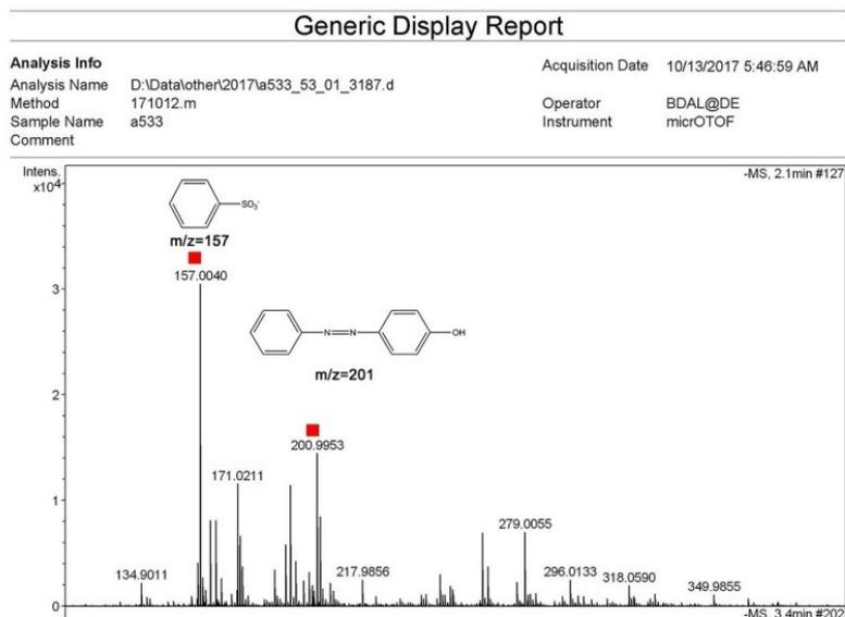
**Fig. S10.** The main intermediate products generated during the course of photocatalytic degradation of MO over  $\text{SiW}_{12}/\text{g-C}_3\text{N}_4$  after 30 min visible light irradiation.
