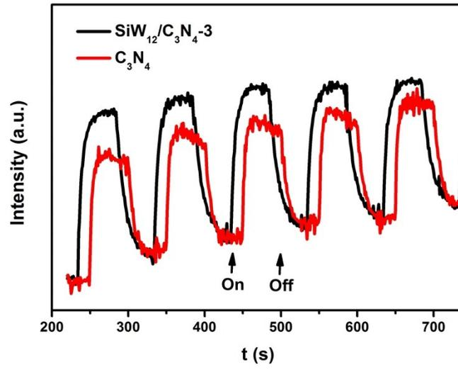
Fig.S6. Photocurrent response test of  $\text{SiW}_{12}/\text{C}_3\text{N}_4\text{-3}$  and  $\text{C}_3\text{N}_4$ .
