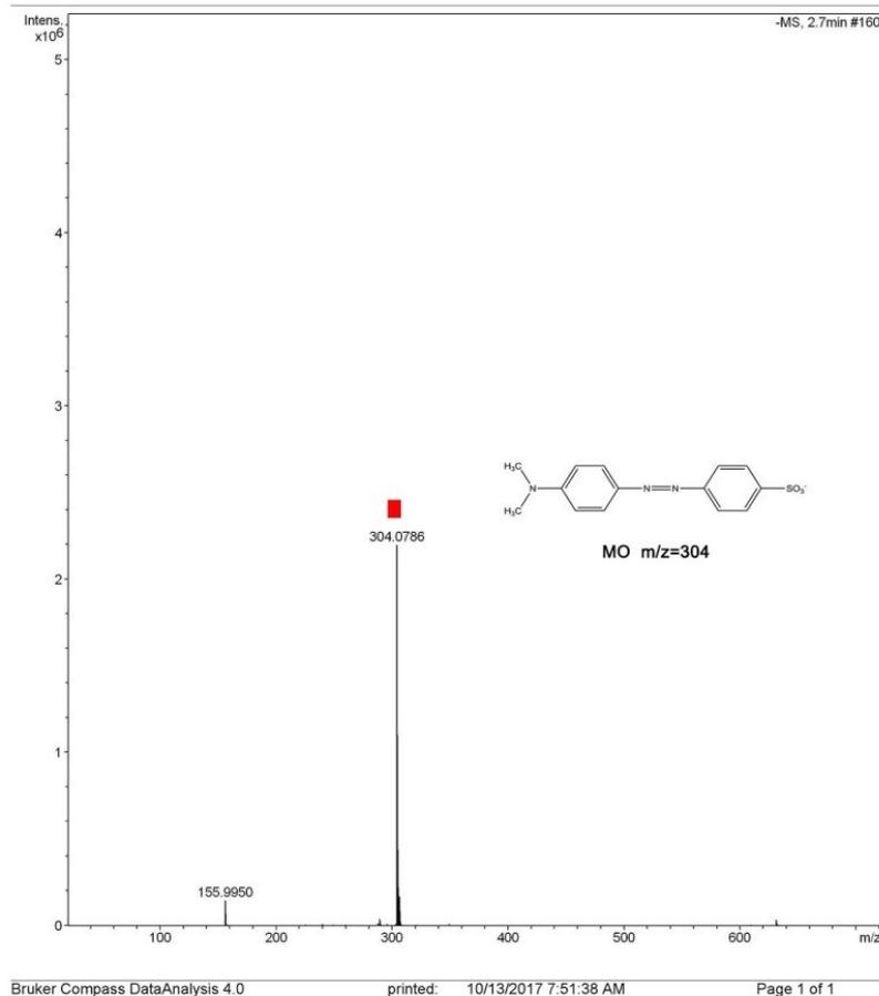
**Fig. S8.** The HPLC/MS image of MO without light irradiation. HPLC/MS identified intermediate products yielded during the process of visible-light photocatalytic degradation of MO. C<sub>18</sub> column, UV detector ( $\lambda=227\text{nm}$ ), and acetonitrile/water (60/40, v/v) was used as a mobile phase at a flow rate of 1.0 mL/min.
