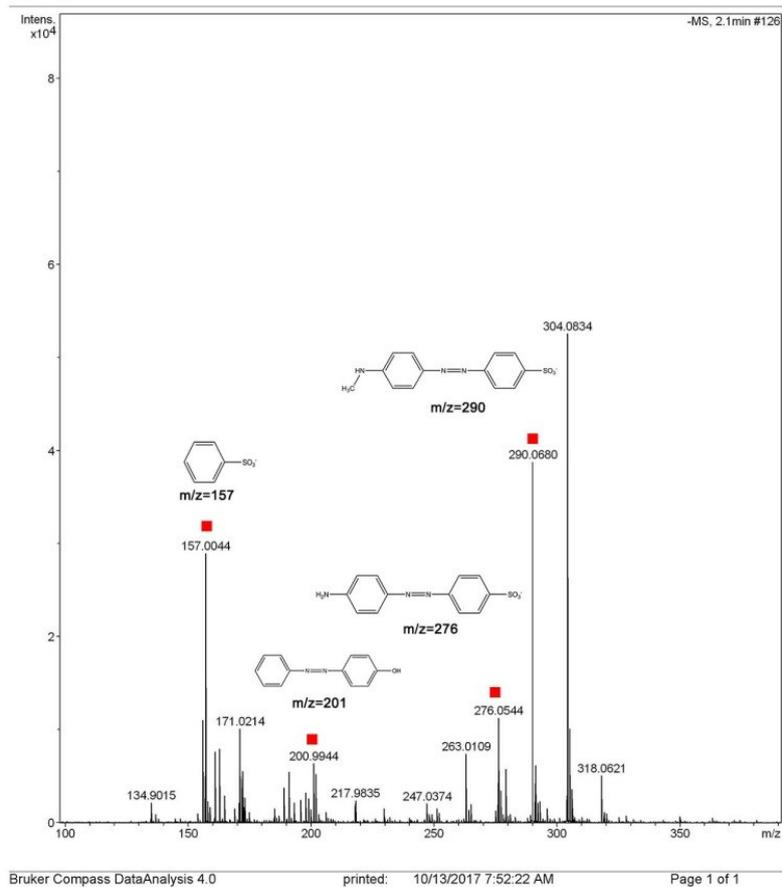
**Fig. S9.** The main intermediate products generated during the process of photocatalytic degradation of MO using SiW<sub>12</sub>/g-C<sub>3</sub>N<sub>4</sub> as catalysts after 15 min visible light irradiation.
