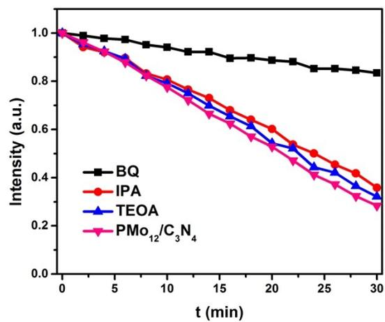
**Fig.S5** Photocatalytic degradation of MO over PMo<sub>12</sub>/C<sub>3</sub>N<sub>4</sub> photocatalyst alone and with the addition of IPA or BQ and TEOA.
