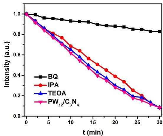
**Fig.S4** Photocatalytic degradation of MO over PW<sub>12</sub>/C<sub>3</sub>N<sub>4</sub> photocatalyst alone and with the addition of IPA or BQ and TEOA.
