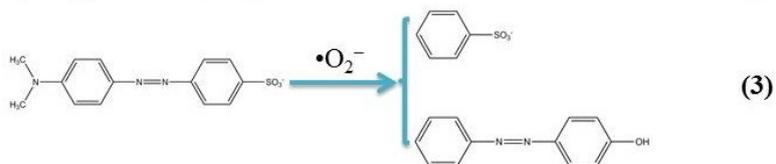
**Fig. S12.** Proposed degradation process and product.
