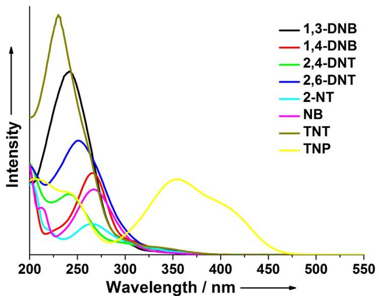
**Fig. S16** The absorption spectrum of the selected analytes in water.
