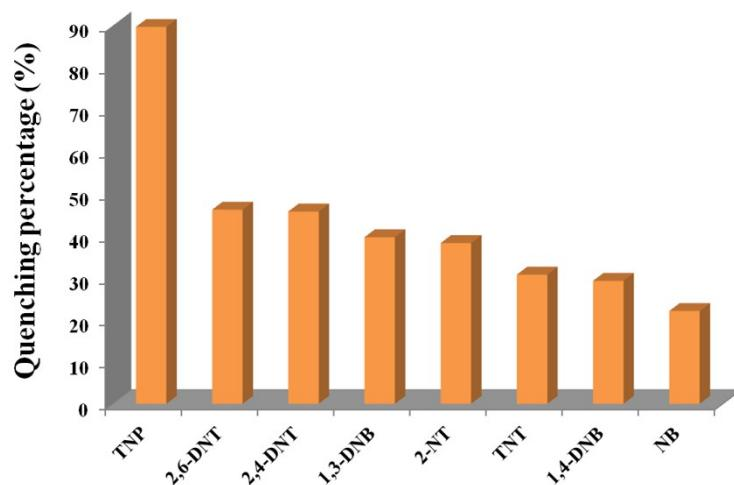
**Fig. S12** Quenching efficiency of the fluorescent intensity for **2** dispersed in 1 mM or saturated aqueous solutions of the selected analytes at room temperature.
