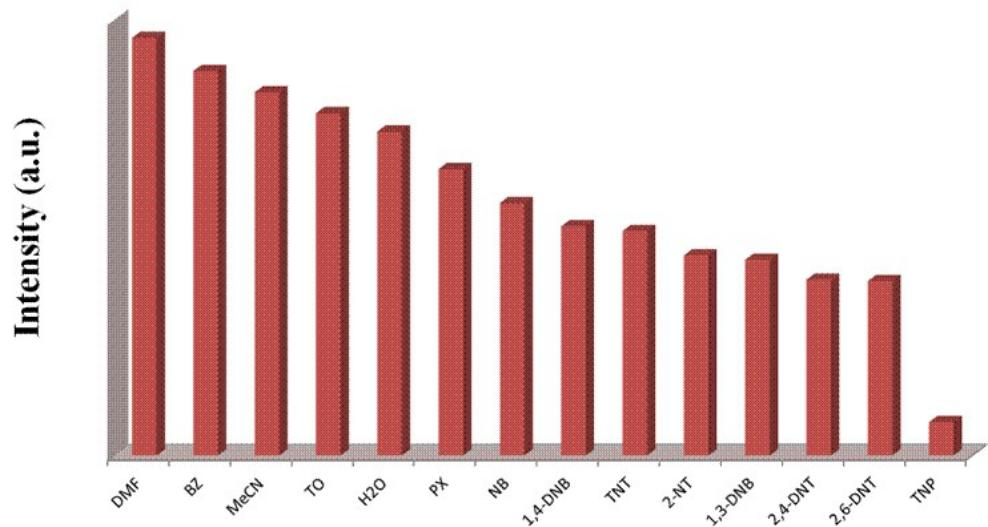
**Fig. S11** The fluorescent intensity (544 nm) for **2** dispersed in  $\text{H}_2\text{O}$ , MeCN, DMF, BZ, TO, PX and 1 mM or saturated aqueous solutions of seven different analytes at room temperature.
