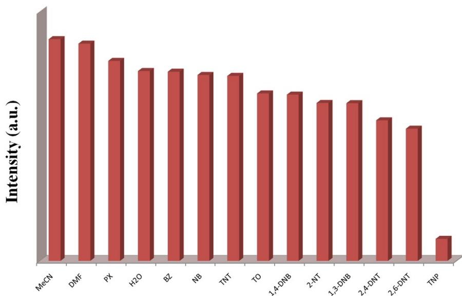
**Fig. S8** The fluorescent intensity (609 nm) for **1** dispersed in H<sub>2</sub>O, MeCN, DMF, BZ, TO, PX and 1 mM or saturated aqueous solutions of seven different analytes at room temperature.
