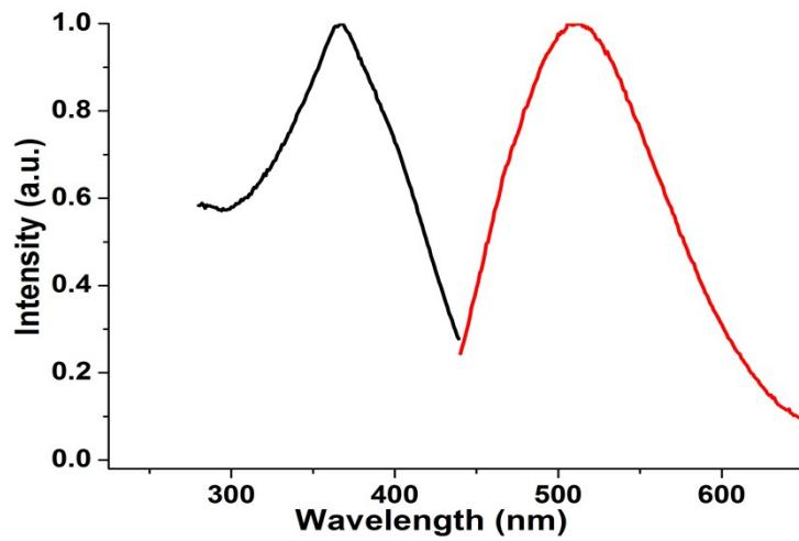
**Fig. S6** Solid-state excitation and emission spectra for  $\text{H}_2\text{L}$ .
