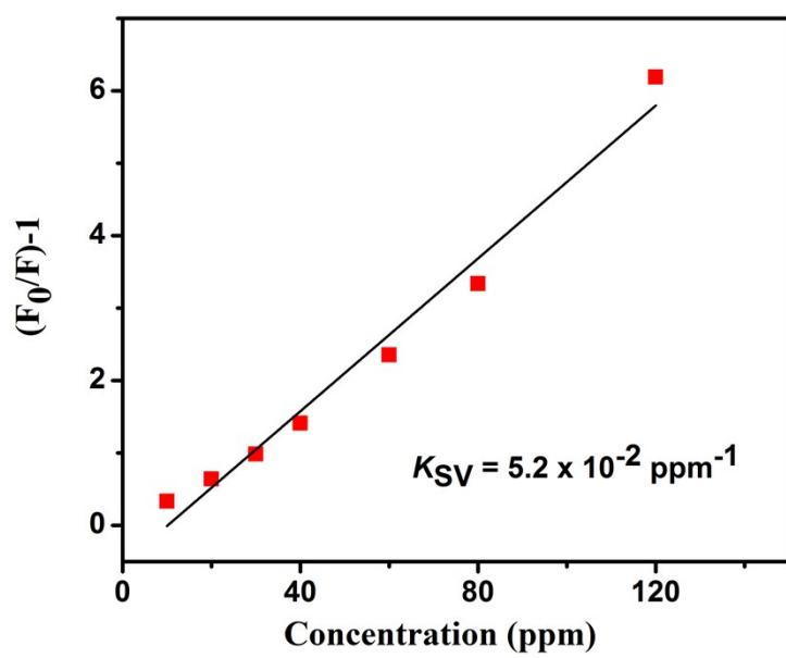
**Fig. S14** Stern-Volmer plot of  $F_0/F$  vs. TNP concentration in aqueous solution for **1**.
