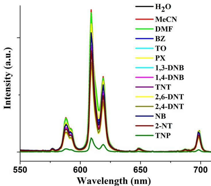
**Fig. S7** The emission spectra for **1** dispersed in  $\text{H}_2\text{O}$ , MeCN, DMF, BZ, TO, PX and 1 mM or saturated aqueous solutions of seven different analytes at room temperature.
