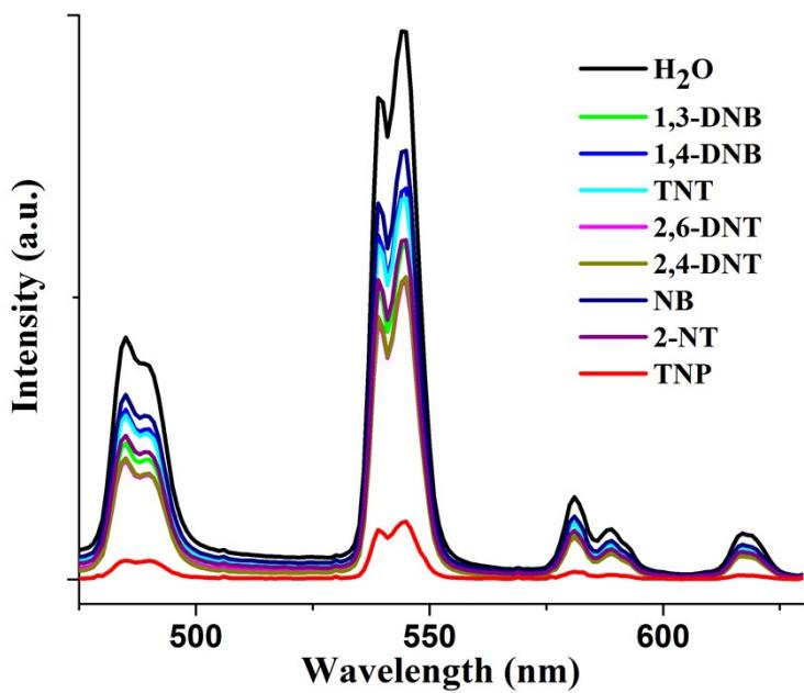
**Fig. S10** The emission spectra for **2** dispersed in  $\text{H}_2\text{O}$  and 1 mM or saturated aqueous solutions of the selected analytes at room temperature.
