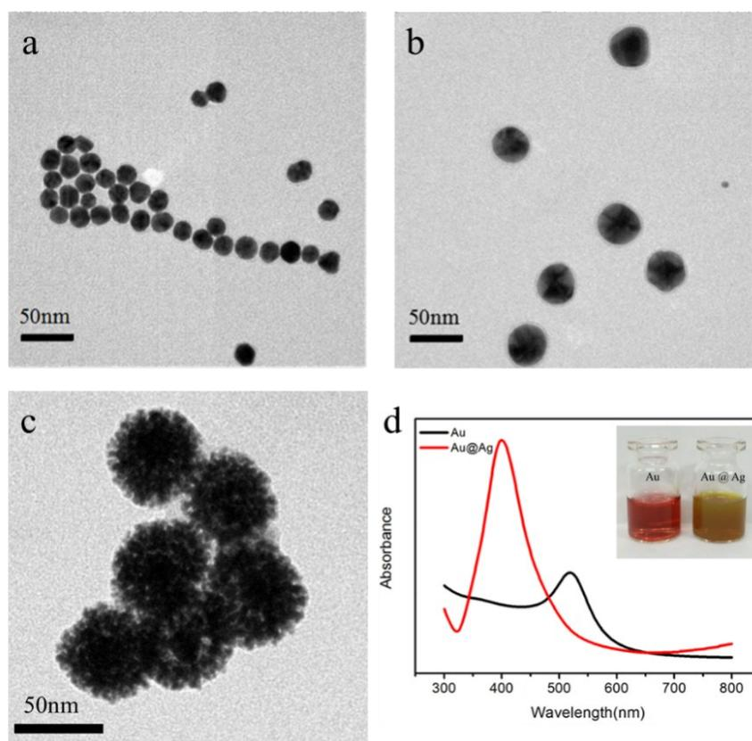
Fig. S4. TEM images of nanoparticles: (a) Au, (b) Au@Ag, (c) Au@porous Ag/Pt yolk-shell. (d) UV-vis absorption spectra of Au@Ag and Au.
