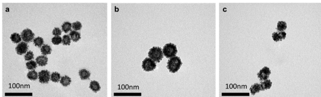
Fig. S3. TEM images of nanoparticles synthesized at different reaction temperatures: (a) 25 °C, (b) 50 °C, and (c) 80 °C.
