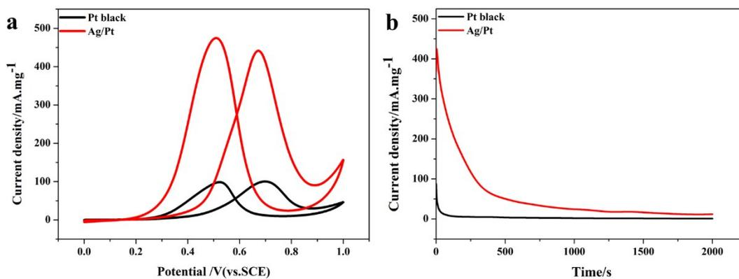
Fig. S7. CV (a) and CA (b) curves for methanol oxidation over commercial Pt black and hollow dendritic Ag/Pt alloy nanoparticles in 0.5 M H<sub>2</sub>SO<sub>4</sub> containing 1 M CH<sub>3</sub>OH.
