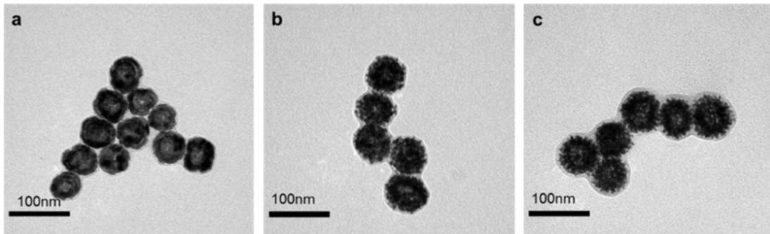
Fig. S1. TEM images of nanoparticles obtained using different surfactants: (a) P123, (b) F127, and (c) Brij58.
