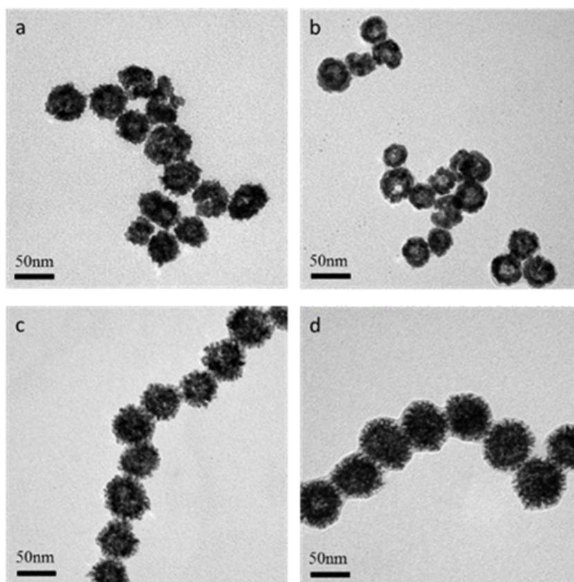
Fig. S2. TEM images of nanoparticles obtained at different surfactant concentrations: (a) 0 mg/mL, (b) 0.1 mg/mL, (c) 1 mg/mL, and (d) 10 mg/mL.
