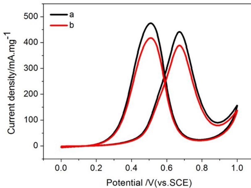
Fig. S8. CV curves for methanol oxidation over Ag/Pt nanoparticles: (a) fresh electrode, (b) the same electrode stored after a week.
