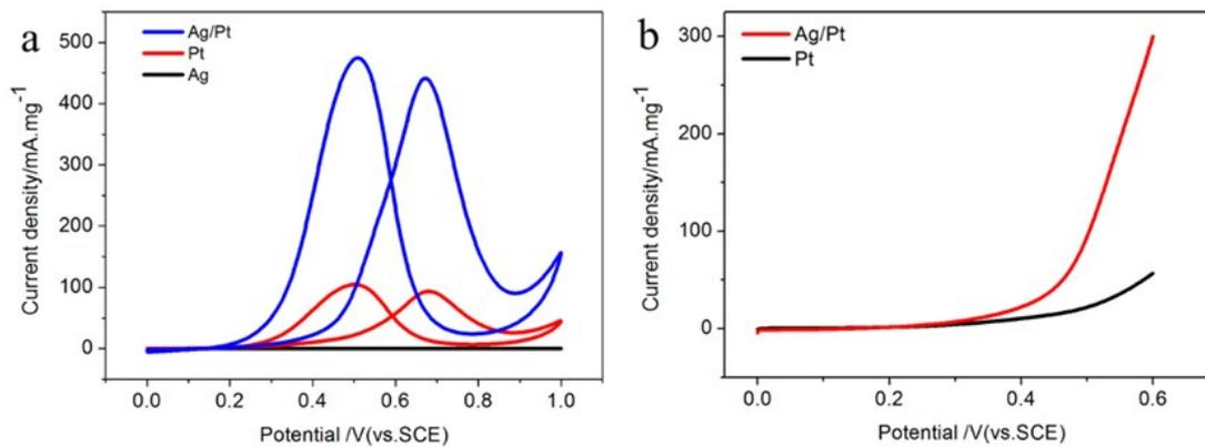
Fig. S6. CV (a) and LSV (b) curves for methanol oxidation over hollow dendritic Ag/Pt alloy nanoparticles, pure Pt and pure Ag nanoparticles in 0.5 M  $\text{H}_2\text{SO}_4$  containing 1 M  $\text{CH}_3\text{OH}$ .
