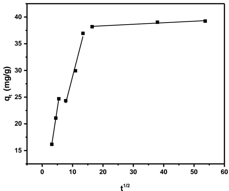
Figure S9. Intraparticle diffusion kinetic plot for arsenic adsorption onto the activated MOF
