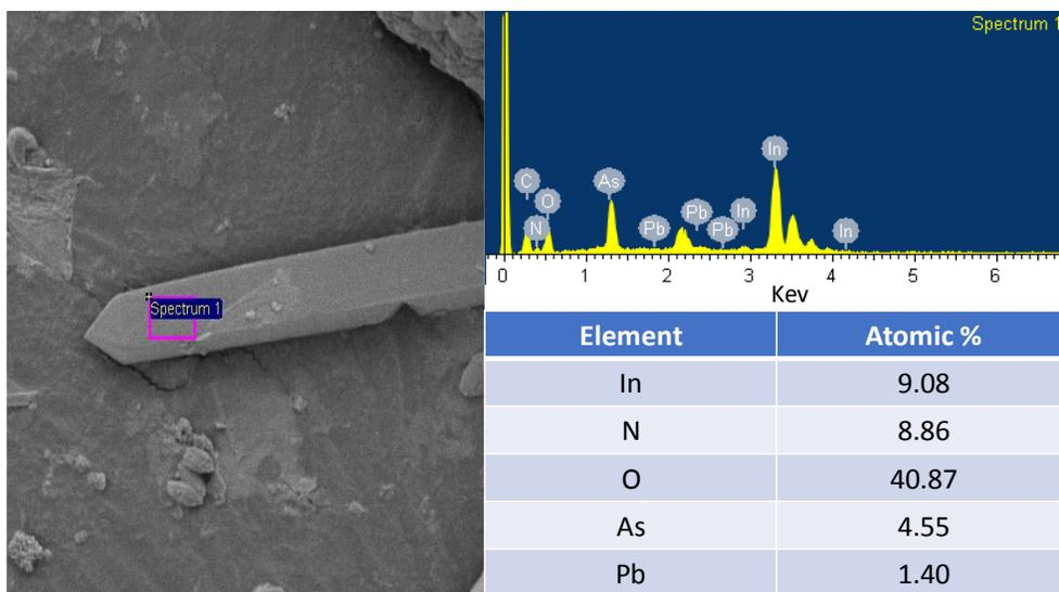
**Figure S14.** Arsenic removal in the presence of  $Pb^{2+}$  (A). SEM-EDX of the collected sample after the adsorption test showing the adsorption of both As and Pb on the surface of the MOF crystals (B).  $[As]_0 = [Pb]_0 = 25$  ppm  $m_{AUBM-1} = 10$  mg.
