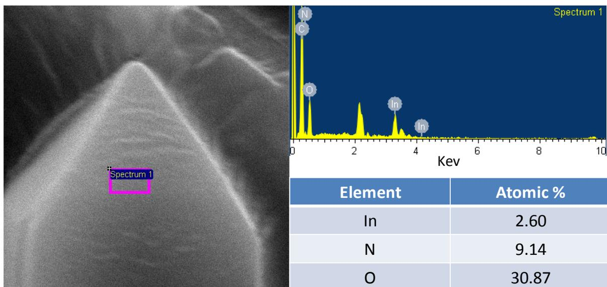
**Figure S4.** SEM EDX of washed In-MOF
