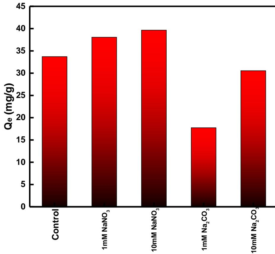
**Figure S13.** As adsorption by AUBM-1 in the presence of anions.  $m_{\text{AUBM-1}} = 10$  mg;  $[\text{As}]_0 = 40$  mg/L, contact time = 12 h. the control experiment was performed in the absence of anions.
