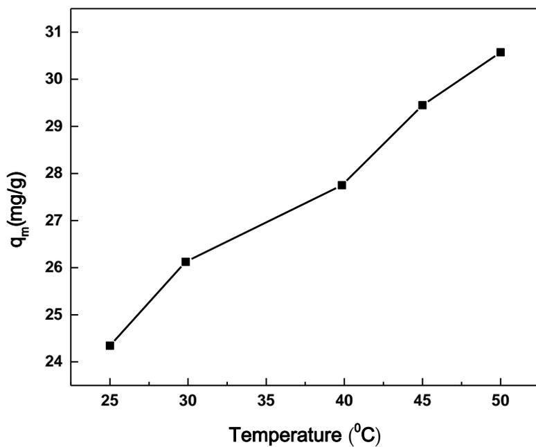
Figure S10. Effect of temperature on the As removal by the MOF
