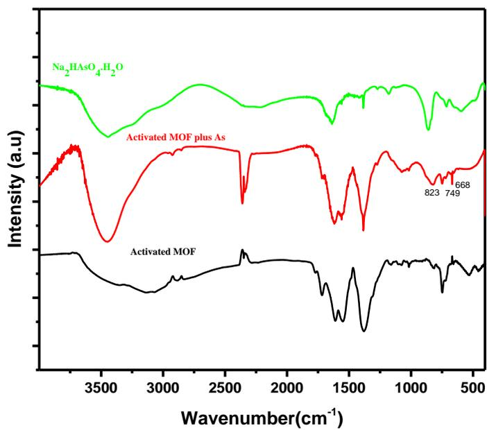
**Figure S11.** IR spectrum of  $\text{Na}_2\text{HAsO}_4 \cdot \text{H}_2\text{O}$  (green), activated MOF plus As (red), and activated MOF (black)
