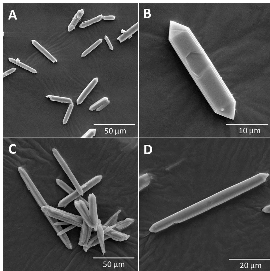
**Figure S2.** HRSEM images of AUBM-1 after dispersion in solutions of pH 2 (A and B) and pH 8 (C and D).
