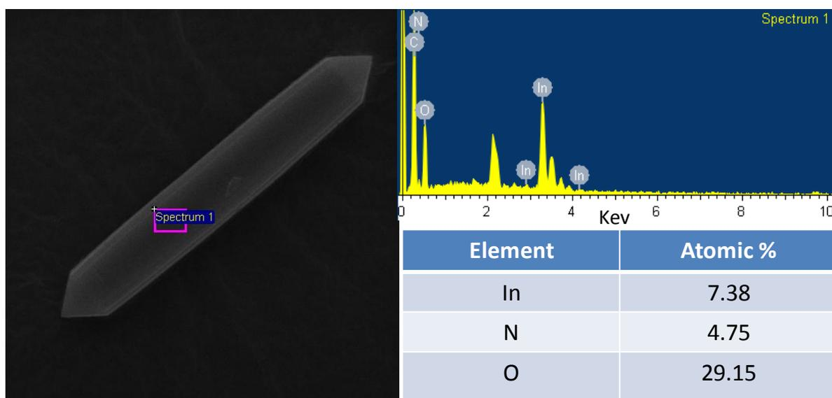
**Figure S5.** SEM-EDX of activated In-MOF
