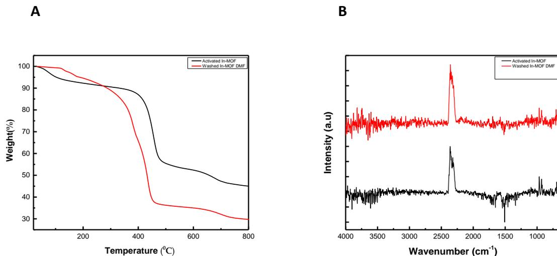
**FigureS6.** TGA curves of the washed In-MOF and activated one (A), FTIR spectra recorded for the produced species (ammonia) from the combustion of the washed sample between 560 to 706 °C (max appeared at 635°C) and for activated sample between 485 - 755 °C (max appeared at 647 °C); For the washed In-MOF NH<sub>3</sub> gas was detected.
