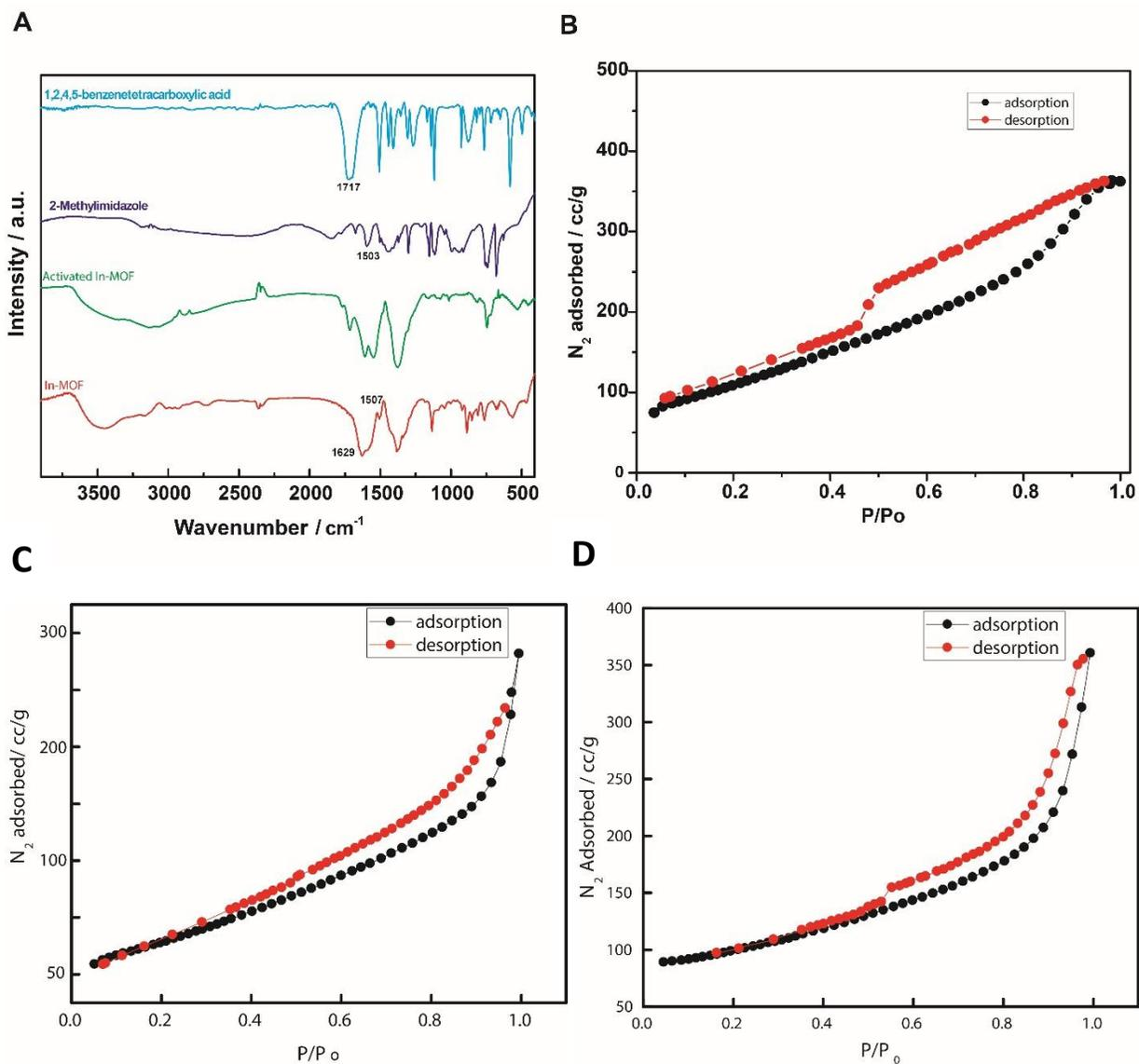
**Figure S3.** (A) IR spectra of the as synthesized MOF, 2-methylimidazole and 1,2,4,5 benzenetetracarboxylic acid, (B) N<sub>2</sub> isotherm of the MOF at 77 K. (C) N<sub>2</sub> isotherm of the MOF after treatment with acid (pH =2) (D) N<sub>2</sub> isotherm of the MOF after treatment with basic solution (pH =8).
