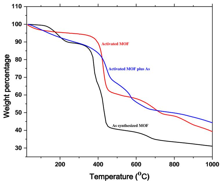
**Figure S12.** TGA curve as synthesized MOF (red), activated MOF plus As (blue), and As-synthesized MOF (black).
