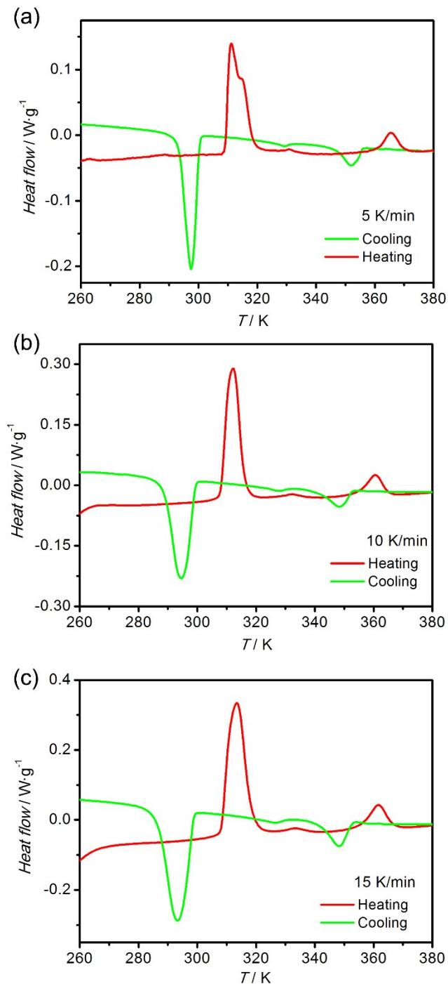
**Figure S2.** DSC curve of **1** measured at sweeping rates of (a) 5 K/min, (b) 10 K/min and (c) 15 K/min in a heating-cooling cycle.
