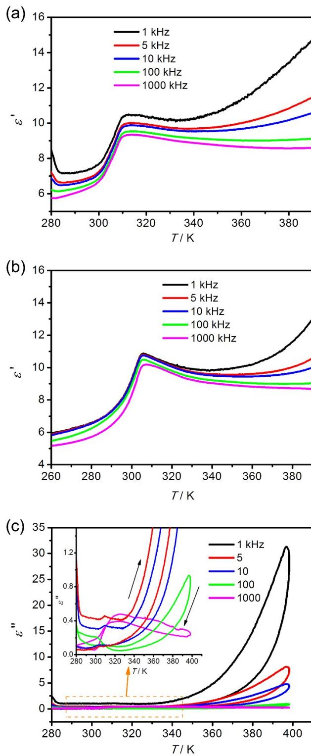
**Figure S7.** (a) Heating and (b) cooling modes of the real part and (c) imaginary part of dielectric constant of polycrystalline sample **1** measured at selected frequencies 1–1000 kHz in a heating/cooling cycle.
