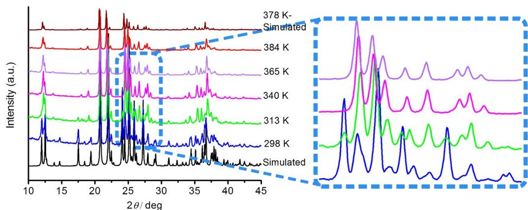
**Figure S5.** Variable-temperature PXRD patterns of **1** measured upon heating, together with simulated patterns from single-crystal X-ray diffraction data.
