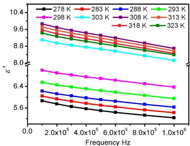
**Figure S8.** Frequency dependence of  $\epsilon'$  of polycrystalline sample **1** from 273 K to 323 K.
