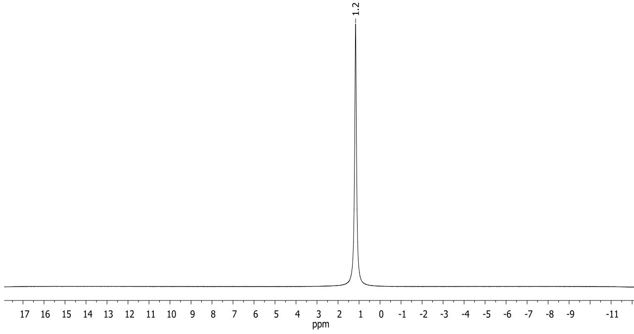
**Fig 3.**  $^7\text{Li}\{\text{H}\}$  NMR spectrum of  $1,8\text{-C}_{10}\text{H}_6[\text{N}(\text{SiMe}_3)\text{Li}(\text{OEt}_2)]_2$  (**1<sup>Et2O</sup>**) (155.5 MHz,  $\text{C}_6\text{D}_6$ , 293K).
