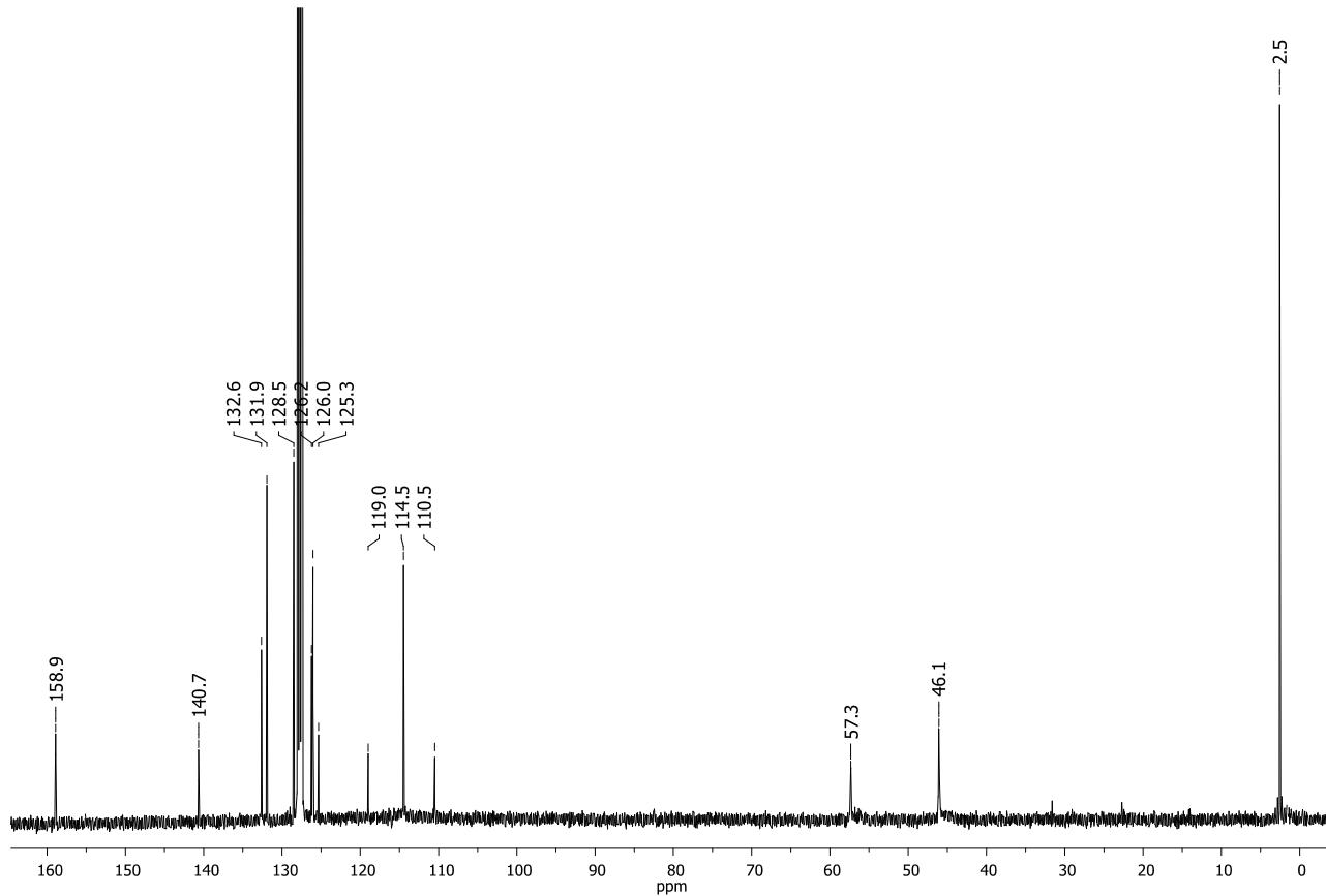
**Fig 11.**  $^{13}\text{C}\{^1\text{H}\}$  NMR spectrum of  $1,8\text{-C}_{10}\text{H}_6[\text{N}(\text{SiMe}_3)\text{Li}(\text{N}\equiv\text{CPh})][\text{N}(\text{SiMe}_3)\text{Li(TMEDA)}]$  ( $\text{2}^{\text{TMEDA}}$ ) (100 MHz,  $\text{C}_6\text{D}_6$ , 293 K).
