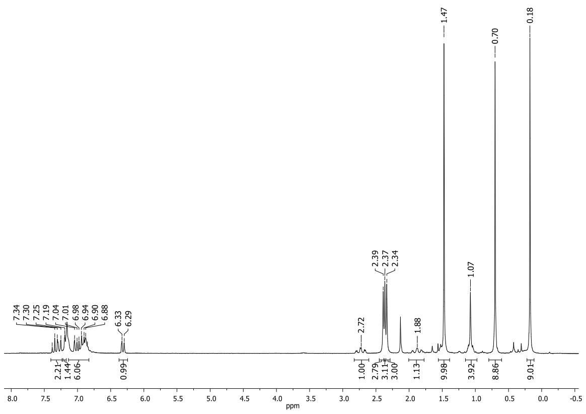
**Fig. 21.**  $^1\text{H}$  NMR spectrum of  $\{1,8-\text{C}_{10}\text{H}_6[\text{NSiMe}_3][\text{NC}(\text{Ph})\text{NSiMe}_3]\}\text{YOtBu(TMEDA)}$  (**8**) (400 MHz,  $\text{C}_6\text{D}_6$ , 293 K).
