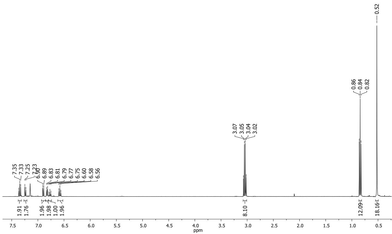
**Fig 7.**  $^1\text{H}$  NMR spectrum of  $1,8\text{-C}_{10}\text{H}_6[\text{N}(\text{SiMe}_3)\text{Li}(\text{N}\equiv\text{CPh})(\text{OEt}_2)][\text{N}(\text{SiMe}_3)\text{Li}(\text{OEt}_2)]$  ( $\mathbf{2}^{\text{Et2O}}$ ) (400 MHz,  $\text{C}_6\text{D}_6$ , 293 K).
