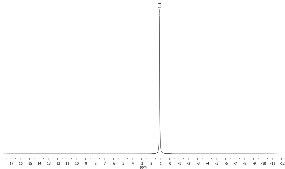
**Fig 6.**  $^7\text{Li}\{^1\text{H}\}$  NMR spectrum of  $1,8\text{-C}_{10}\text{H}_6[\text{N}(\text{SiMe}_3)\text{Li(TMEDA)}]_2$  ( $\mathbf{1}^{\text{TMEDA}}$ ) (155.5 MHz,  $\text{C}_6\text{D}_6$ , 293 K).
