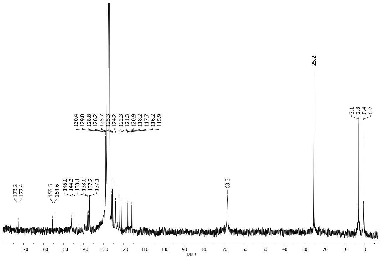
**Fig. 14.**  $^{13}\text{C}\{^1\text{H}\}$  NMR spectrum of  $\{\{1,8-\text{C}_{10}\text{H}_6[\text{NSiMe}_3][\text{NC}(\text{Ph})\text{NSiMe}_3]\}\{1,8-\text{C}_{10}\text{H}_6[\text{N(H)SiMe}_3][\text{NC}(\text{Ph})\text{NSiMe}_3]\}\text{YCl}\}[\text{Li}(\text{THF})_4]$  (**3Y**) (50 MHz,  $\text{C}_6\text{D}_6$ , 293 K).
