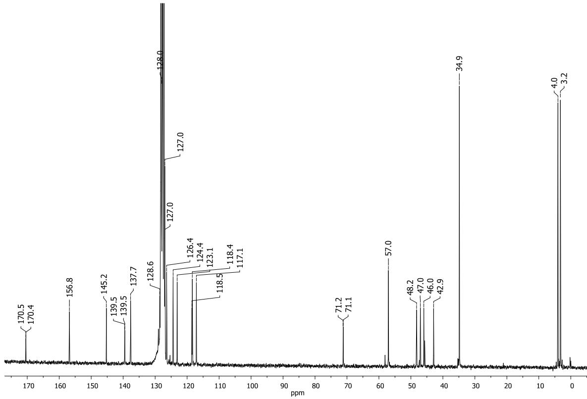
**Fig. 22.**  $^{13}\text{C}\{^1\text{H}\}$  NMR spectrum of  $\{1,8-\text{C}_{10}\text{H}_6[\text{NSiMe}_3][\text{NC}(\text{Ph})\text{NSiMe}_3]\}\text{YOtBu(TMEDA)}$  (**8**) (50 MHz,  $\text{C}_6\text{D}_6$ , 293 K).
