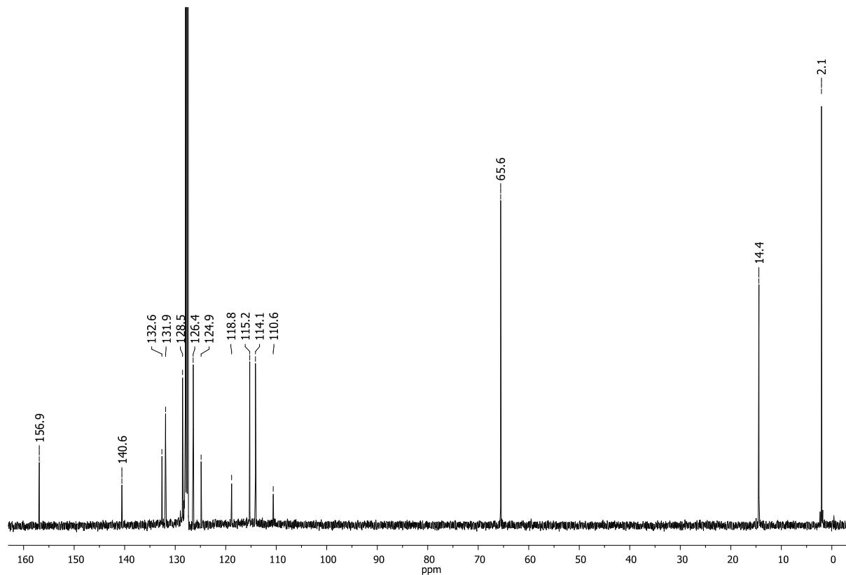
**Fig 8.**  $^{13}\text{C}\{^1\text{H}\}$  NMR spectrum of  $1,8\text{-C}_{10}\text{H}_6[\text{N}(\text{SiMe}_3)\text{Li}(\text{N}\equiv\text{CPh})(\text{OEt}_2)][\text{N}(\text{SiMe}_3)\text{Li}(\text{OEt}_2)]$  ( $\mathbf{2}^{\text{Et2O}}$ ) (100 MHz,  $\text{C}_6\text{D}_6$ , 293 K).
