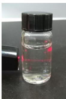
**Figure S12.** The photographic of using laser to irradiate the solution after solvent exchange. We can see very weak Tyndall Effect.
