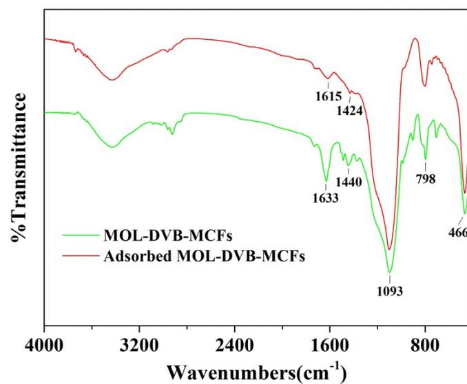
**Fig. S6** FTIR spectra of MOL-DVB-MCFs and MOL-DVB-MCFs loaded with  $\text{Eu}^{3+}$ .
