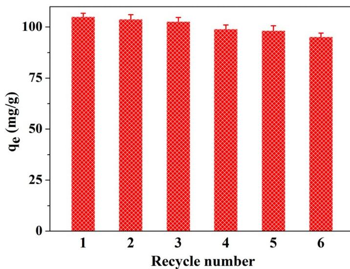
**Fig. S7** Reusability evaluation of the composite by repeated adsorption of  $\text{Eu}^{3+}$  and evaluating the obtained adsorption capacity  $q_e$ .
