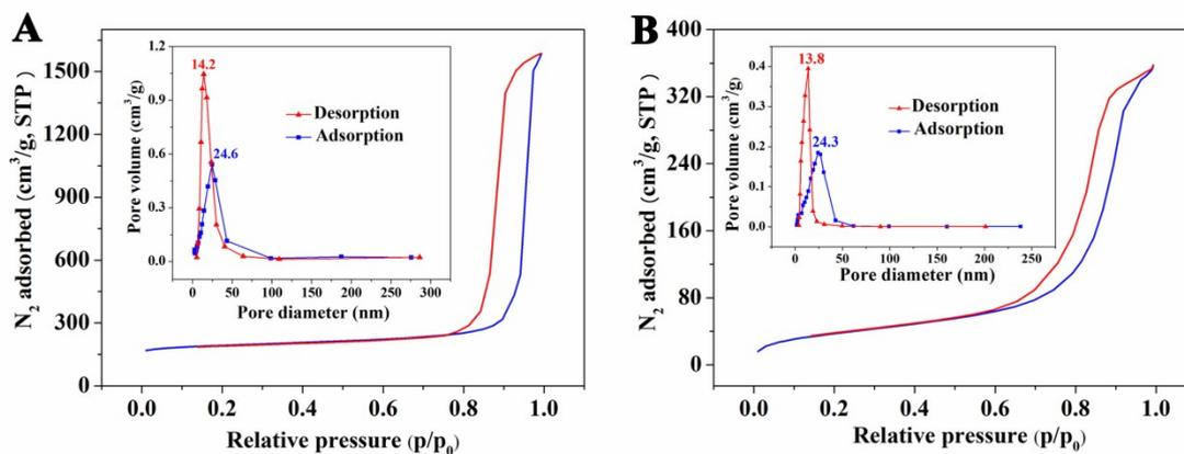
**Fig. S2** Nitrogen sorption isotherms and corresponding pore size analyses based on the Barrett-Joyner-Halenda (BJH) pore analysis method for MCFs (A) and MOL-DVB-MCFs (B).
