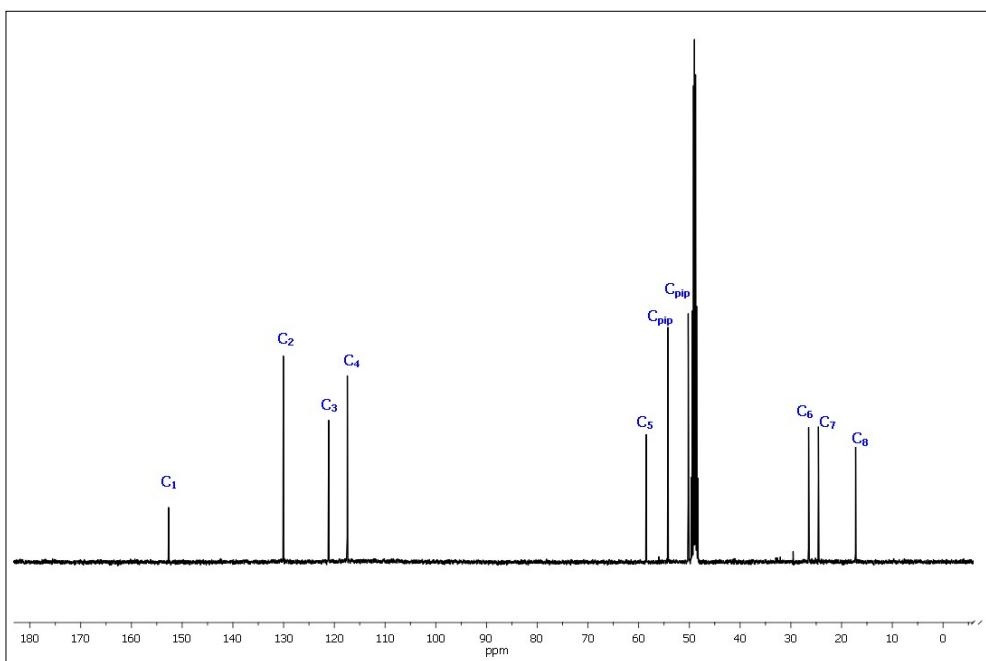
**Figure 6.**  $^{13}\text{C}$  NMR ( $\text{CDCl}_3$ ) phenyl piperazine (**2b**).
