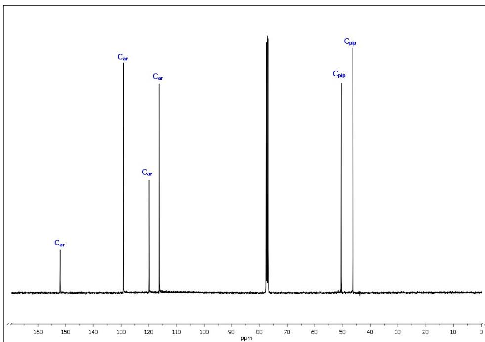
**Figure 2.**  $^{13}\text{C}$  NMR ( $\text{CDCl}_3$ ) cyclophenyl piperazine (**1b**).
