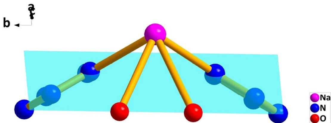
Fig. S8 Coordination environment of Na3 in crystal 2.
