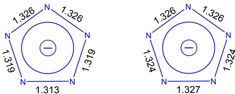
**Fig. S3** The two forms of  $N_5^-$  rings. Bond lengths in Å.
