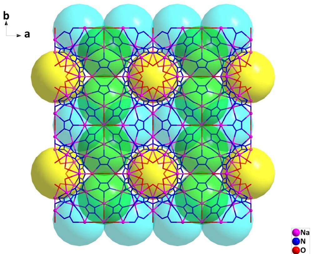
Fig. S12 3D framework of 2 view along c axis.
