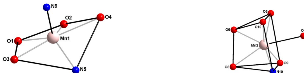
Figure S4. Coordination geometry for Mn1 (distorted pentagonal pyramidal) and Mn2 (distorted monocapped trigonal prism).
