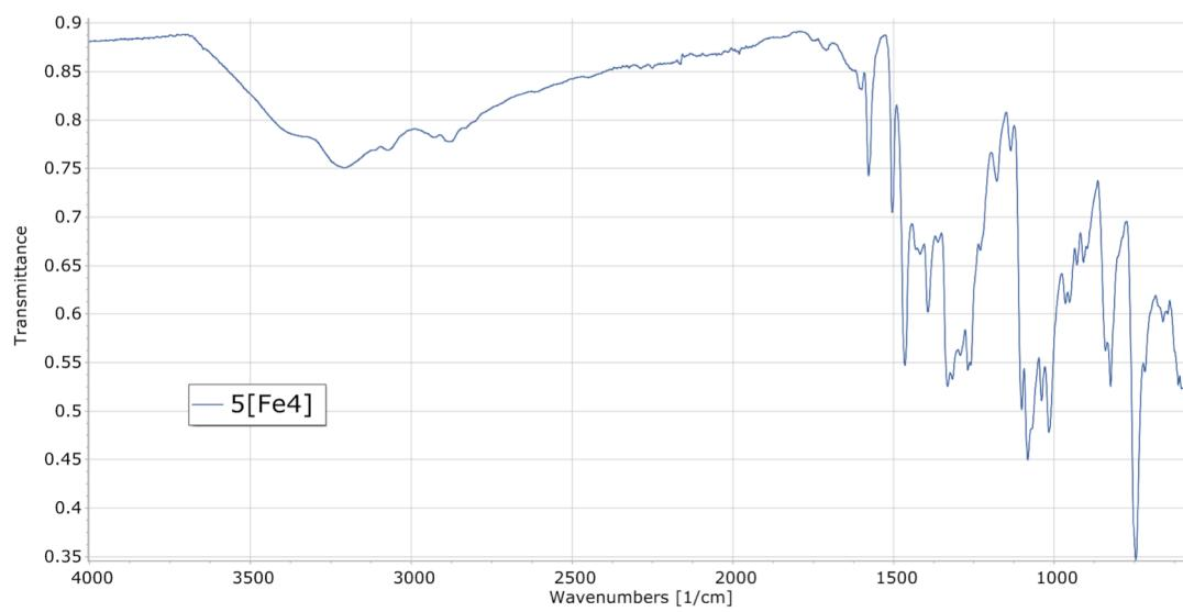
**Figure S5.** Infrared spectrum of Compound 5.
