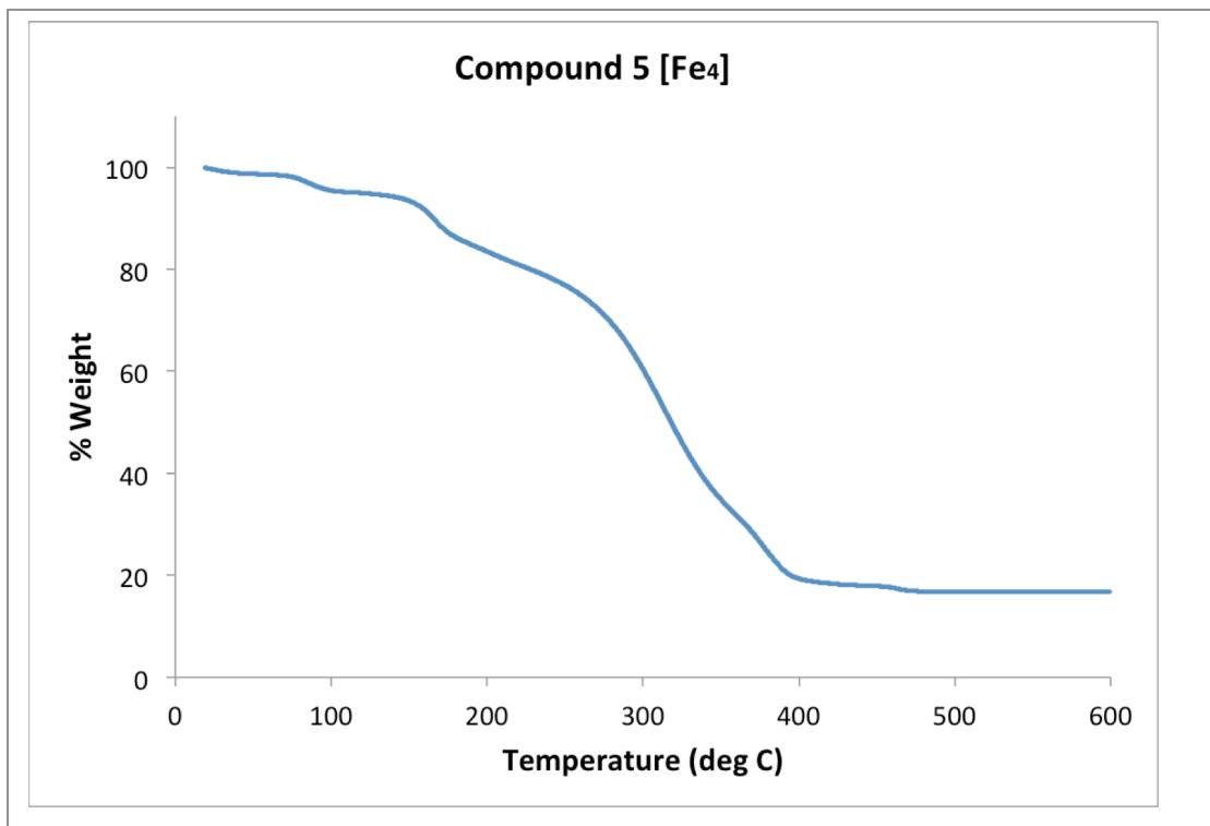
**Figure S13.** Thermogravimetric analysis (TGA) of Compound 5 is presented.
