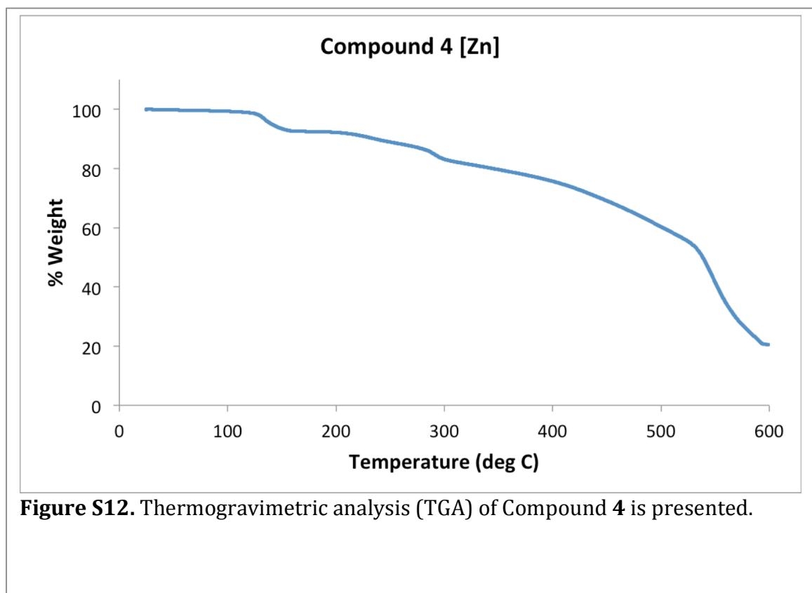
**Figure S12.** Thermogravimetric analysis (TGA) of Compound 4 is presented.
