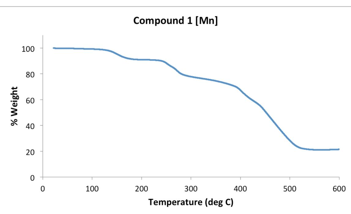
**Figure S9.** Thermogravimetric analysis (TGA) of Compound **1** is presented.
