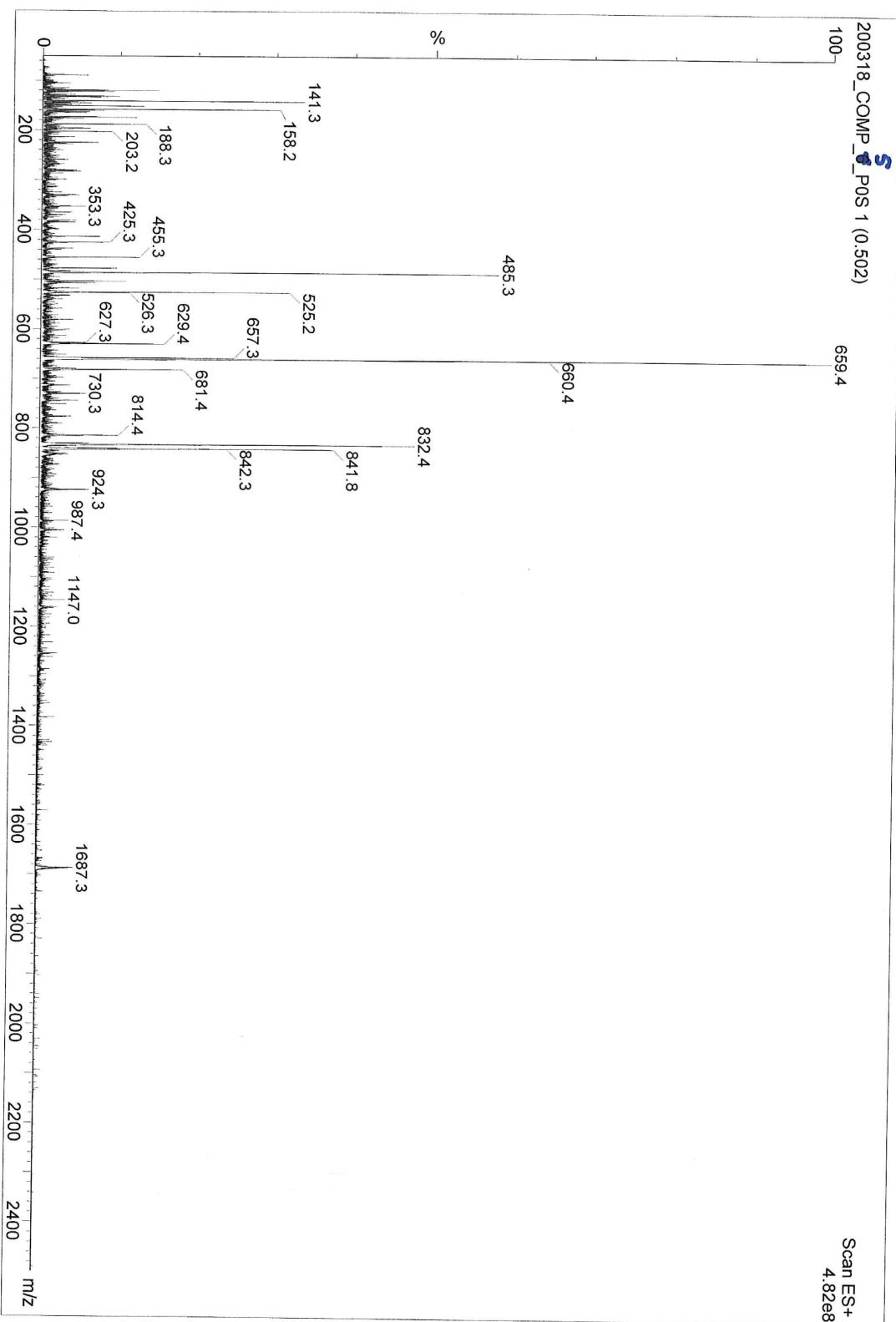
**Figure S22.** ESI-MS of Compound **5** is shown. The peak at  $841(\text{m}/\text{z})$  corresponds to the  $[\text{Fe}_4\text{O}(\text{HL}_2)_2(\text{H}_3\text{L}_3)_2]^{2+}$  fragment.
