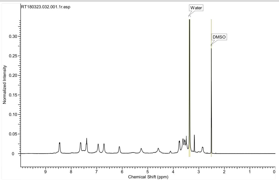
**Figure S16.**  $^1\text{H}$  NMR spectra of Compound 4 in  $\text{DMSO-d}_6$ .
