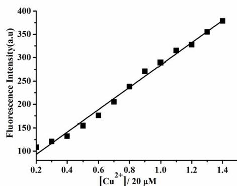
**Figure S12.** Fluorescence intensity calibration curve of probe **L** (20  $\mu\text{M}$ ) as a function of  $\text{Cu}^{2+}$  concentration in  $\text{CH}_3\text{CN}/\text{H}_2\text{O}$  (97/3, v/v, Tris-HCl, pH 7) solution;  $\lambda_{\text{ex}}/\lambda_{\text{em}} = 470 \text{ nm}/525 \text{ nm}$ ;  $Y = 45.19 + 239.0 X$ ,  $R^2 = 0.9910$ , ( $n = 13$ ), 4 ~ 28  $\mu\text{M}$ , LOD = 0.110  $\mu\text{M}$ .
