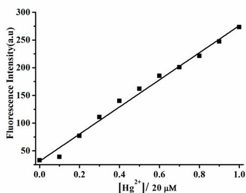
**Figure S10.** Fluorescence intensity calibration curve of probe **L** (20  $\mu\text{M}$ ) as a function of  $\text{Hg}^{2+}$  (measured immediately) concentration in  $\text{CH}_3\text{CN}/\text{H}_2\text{O}$  (97/3, v/v, Tris-HCl, pH 7) solution;  $\lambda_{\text{ex}}/\lambda_{\text{em}} = 360 \text{ nm}/585 \text{ nm}$ ;  $Y = 244.7 X + 31.26$ ,  $R^2 = 0.9893$ , ( $n = 11$ ), 2 ~ 20  $\mu\text{M}$ , LOD = 0.110  $\mu\text{M}$ .
