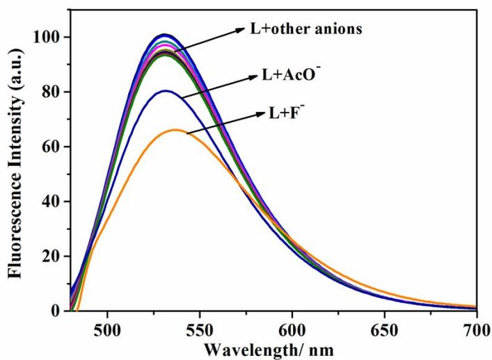
**Figure S7.** Fluorescence spectrum of probe **L** (20  $\mu\text{M}$ ) with 10 equiv. different anions ( $\text{F}^-$ ,  $\text{Cl}^-$ ,  $\text{Br}^-$ ,  $\text{I}^-$ ,  $\text{NO}_3^-$ ,  $\text{HSO}_4^-$ ,  $\text{H}_2\text{PO}_4^-$ ,  $\text{ClO}_4^-$  and  $\text{AcO}^-$ ) in  $\text{CH}_3\text{CN}$  solution;  $\lambda_{\text{ex}}/\lambda_{\text{em}} = 470 \text{ nm}/525 \text{ nm}$ .
