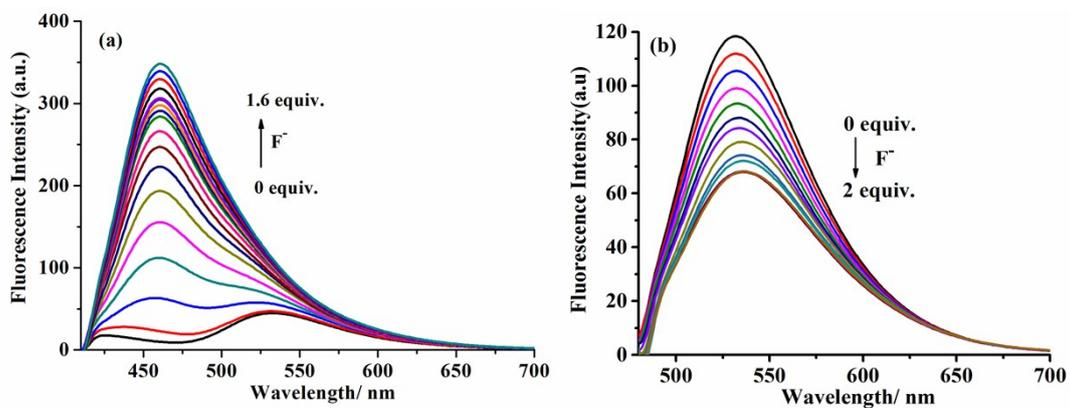
**Figure S8.** Fluorescence spectral titration of probe **L** (20  $\mu\text{M}$ ) with  $\text{F}^-$  in  $\text{CH}_3\text{CN}$  solution; (a)  $\lambda_{\text{ex}}/\lambda_{\text{em}} = 365 \text{ nm}/460 \text{ nm}$ ; (b)  $\lambda_{\text{ex}}/\lambda_{\text{em}} = 470 \text{ nm}/525 \text{ nm}$ .
