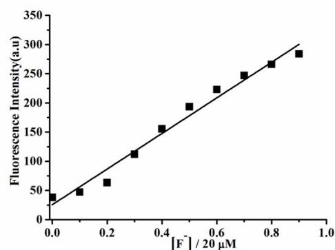
**Figure S13.** Fluorescence intensity calibration curve of probe **L** (20  $\mu\text{M}$ ) as a function of  $\text{F}^-$  concentration in  $\text{CH}_3\text{CN}$ ;  $\lambda_{\text{ex}}/\lambda_{\text{em}} = 365 \text{ nm}/460 \text{ nm}$ ;  $Y = 25.69 X + 305.1$ ,  $R = 0.9764$  ( $n = 10$ ), 2~ 20  $\mu\text{M}$  LOD = 0.106  $\mu\text{M}$ .
