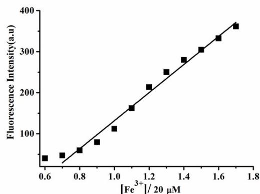
**Figure S11.** Fluorescence intensity calibration curve of probe **L** (20  $\mu\text{M}$ ) as a function of  $\text{Fe}^{3+}$  (measured after 1.5 h) concentration in  $\text{CH}_3\text{CN}/\text{H}_2\text{O}$  (97/3, v/v, Tris-HCl, pH 7) solution;  $\lambda_{\text{ex}}/\lambda_{\text{em}} = 365 \text{ nm}/585 \text{ nm}$ ;  $Y = -210.6 + 342.4 X$ ,  $R^2 = 0.9851$ , ( $n = 12$ ), 12 ~ 36  $\mu\text{M}$  LOD = 0.074  $\mu\text{M}$ .
