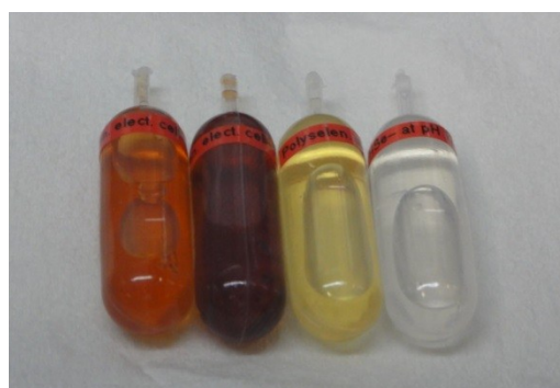
Figure S4. Aliquots of Se solution during the reduction process. The colour of the solution indicates the stage of the process.
