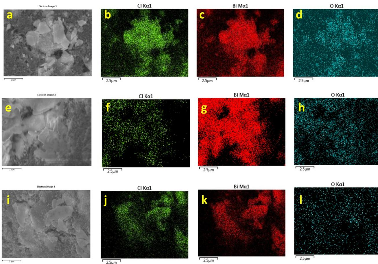
**Supplementary Figure 11.** the SEM images of as-prepared BiOCl (a), the EDX mapping of chloride (b), bismuth (c), and oxygen (d); the SEM images of chloride extraction state of BiOCl (e), the EDX mapping of chloride (f), bismuth (g), and oxygen (h); the SEM images of chloride recovery state of BiOCl (i), the EDX mapping of chloride (j), bismuth (k), and oxygen (l)
