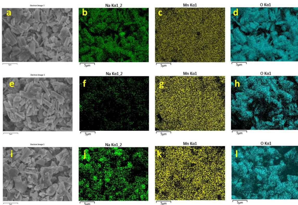
**Supplementary Figure 12.** the SEM images of as-prepared NMO (a) and the corresponding EDX mapping of sodium (b), manganese(c), and oxide (d); the SEM images of sodium extraction state of NMO (e) and the corresponding EDX mapping of sodium (f), manganese(g), and oxide (h); the SEM images of sodium recovery state of NMO (i) and the corresponding EDX mapping of sodium (j), manganese(k), and oxide (l)
