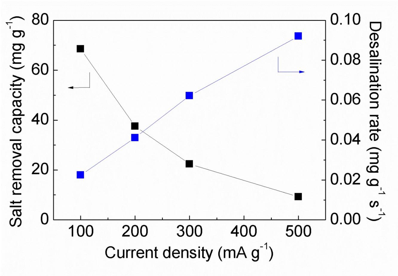
**Supplementary Figure 4.** The salt removal capacity and desalination rate at 100 mA g<sup>-1</sup>, 200 mA g<sup>-1</sup>, 300 mA g<sup>-1</sup>, and 500 mA g<sup>-1</sup>.
