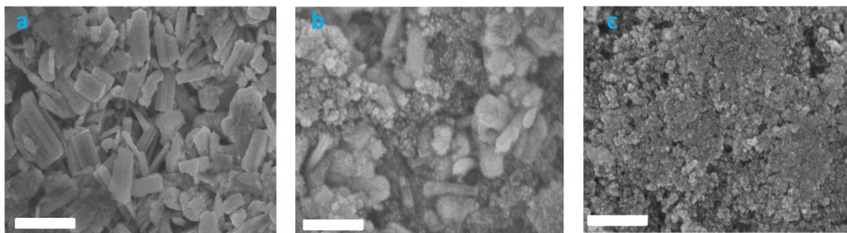
**Supplementary Figure 13.** Morphology change of NMO electrode at initial state (a) and after 20 cycles (b) and 50 cycles(c). Scale bar: 5 $\mu$ m.
