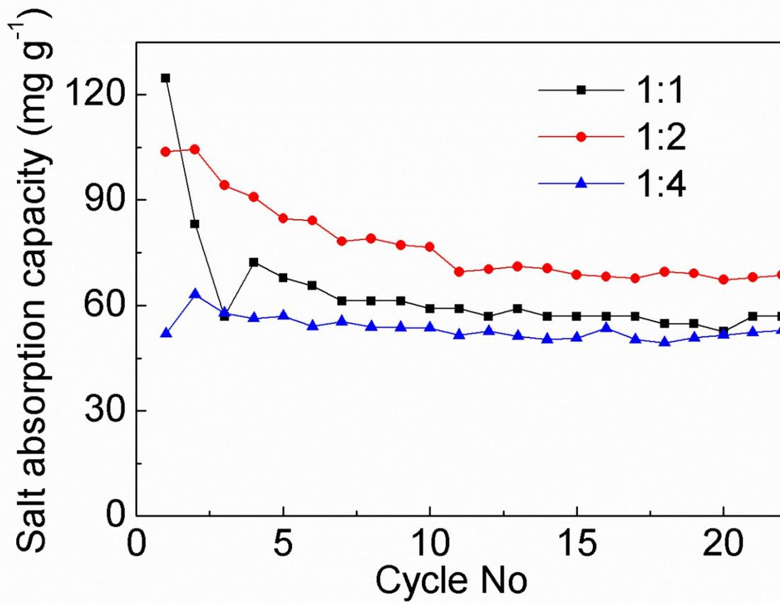
Supplementary Figure 3. the salt removal capacity for the weight ratio of 1:1, 1:2, and 1:4 of BiOCl<sub>3</sub>: NMO
