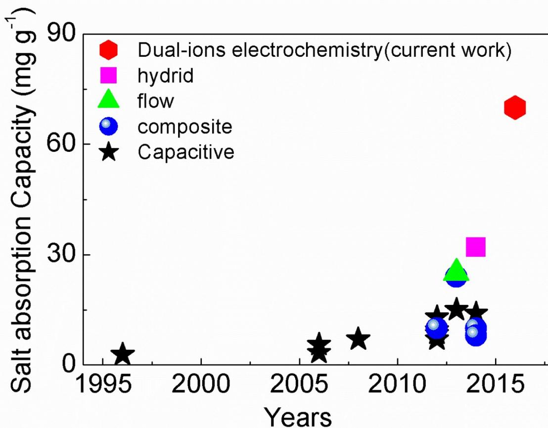
**Supplementary Figure 1.** Historical evolution of maximum salt adsorption capacity for capacitive, composite, hybrid, and flow CDI electrodes <sup>1, 2</sup>, as well as dual-ions electrochemistry deionization (current work).
