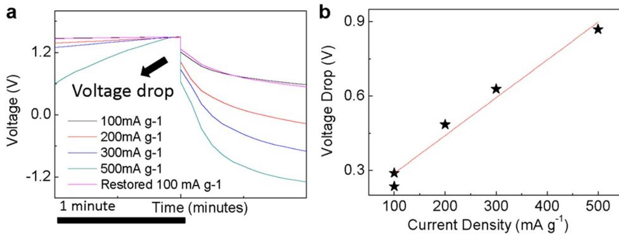
**Supplementary Figure 6.** the voltage drop at different current density, the representative curves were extracted from Figure 2f, black line: cycle 17; blue line: cycle 24; green line: 30; and red line: cycle 36
