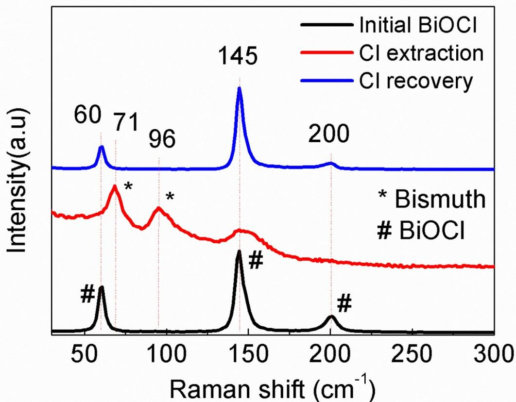
**Supplementary Figure 10.** Raman spectra of initial BiOCl, its state of chloride extraction, and the state of chloride recovery. No peaks were detected from Bi<sub>2</sub>O<sub>3</sub> at the chloride extraction state, indicating its amorphous form.
