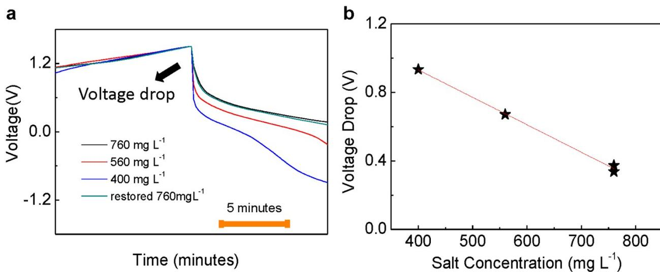
**Supplementary Figure 8.** (a) the voltage drop at different feed concentration, the representative curves were extracted from Figure S5 (d), black line: cycle 7; red line: cycle 32; blue line: 47; and dark cyan: cycle 69
