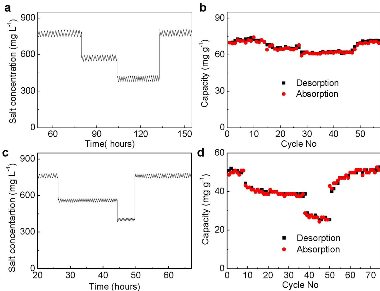
**Supplementary Figure 7.** the influence of feed concentration, (a) the feed concentration change vs. time during cycling and the corresponding salt absorption/desorption capacity(b) at the current density 100 mA g<sup>-1</sup>; (c)the feed concentration change vs. time during cycling and the corresponding salt absorption/desorption capacity(d) at the current density 200 mA g<sup>-1</sup>;
