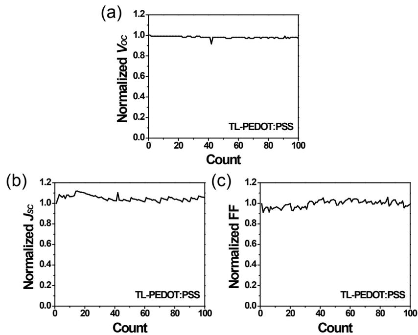
**Fig. S3** Normalized values of (a)  $V_{OC}$ , (b)  $J_{SC}$ , and (c) FF of PSCs after repeated detachment stability test.
