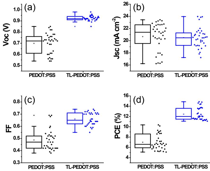
**Fig. S2.** Box charts exhibiting the statistical features of (a)  $J_{sc}$ , (b)  $V_{oc}$ , (c) FF and (d) PCE of all the cells.
