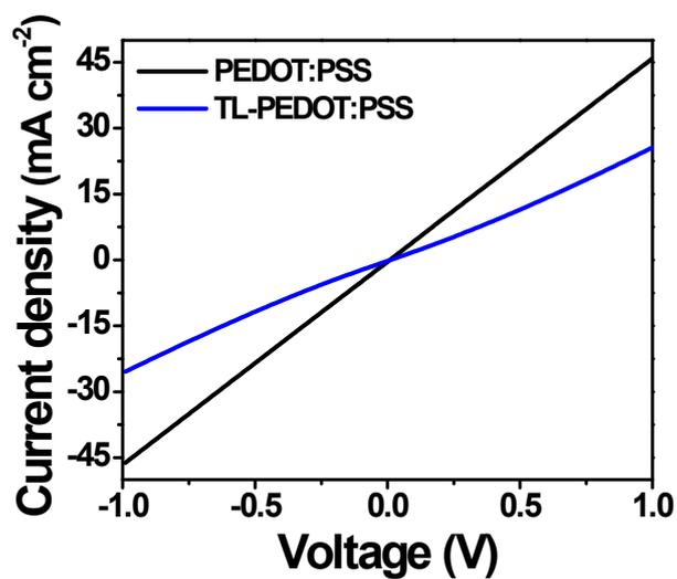
**Fig. S1.** Linear sweep voltammetry curves of FTO/PEDOT:PSS/PEDOT:PSS/FTO and FTO/TL-PEDOT:PSS/TL-PEDOT:PSS/FTO
