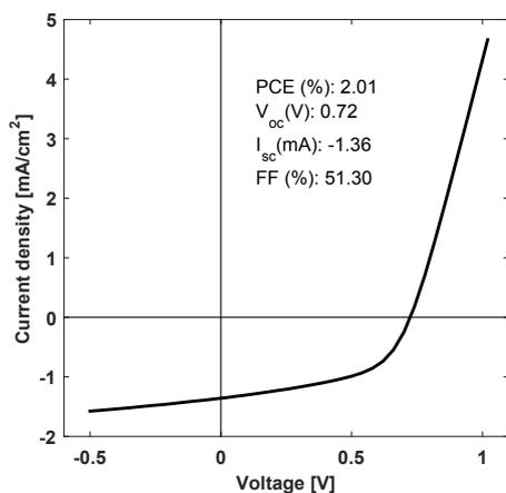
**Figure 14** J–V characteristics of spin coated PBDTTTZ-4:PCBM device with an active area of 0.25 cm<sup>2</sup>.
