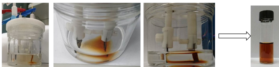
Fig. S2 The transformation process of RE0.025M to BRE0.025M in the three electrode at scan rate of 1000 \text{ mV s}^{-1} .
