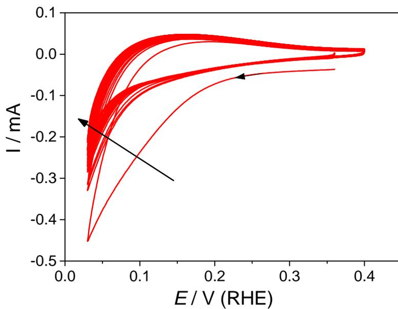
**Fig. S3.** Cyclic voltammograms of Pt/C in 0.5 M H<sub>2</sub>SO<sub>4</sub> + 10 mM DAcPy. Considerable reduction current could be observed in the first cycle, but it declined quickly in the following cycles.
