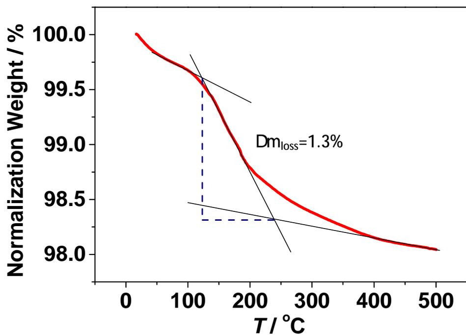
**Fig. S6.** Thermogravimetric curve of DAcPy adsorbed on commercial Pt black in N<sub>2</sub> flow at 10 °C min<sup>-1</sup>. The mass of Pt black was 5 mg, and the specific surface area of Pt black was 20.7 m<sup>2</sup> g<sup>-1</sup> determined by electrochemical hydrogen adsorption/desorption in 0.5 M H<sub>2</sub>SO<sub>4</sub>.
