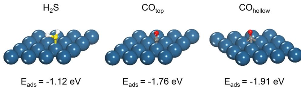
Optimized structures for  $\text{H}_2\text{S}$  and CO adsorption on Pt(111). Blue: Pt; yellow: S; white: H; grey: C; red: O.
