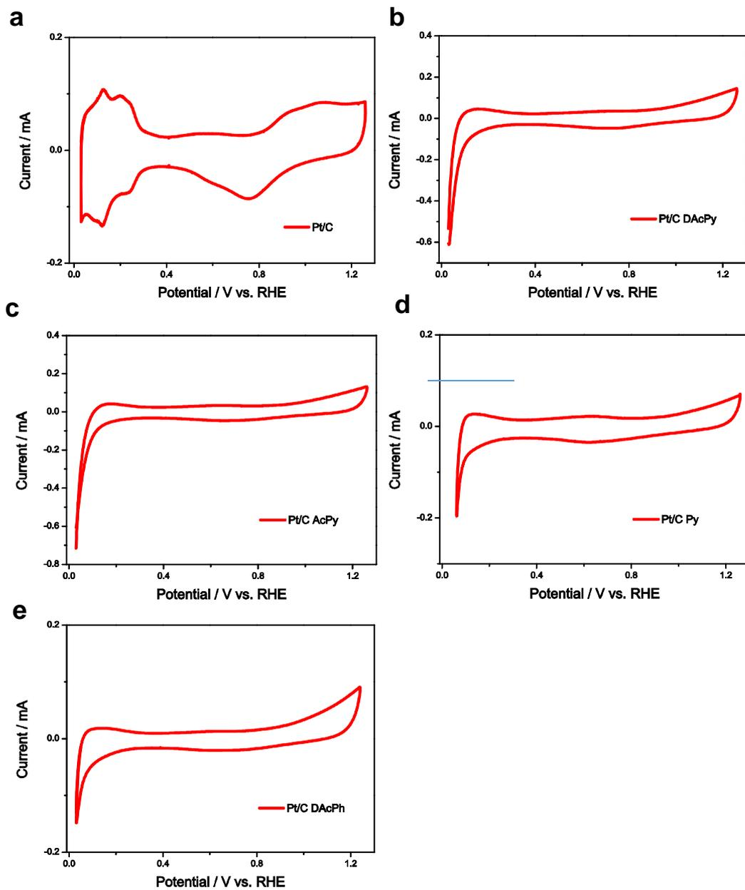
**Fig S2.** Cyclic voltammograms of Pt/C in 0.5 M H<sub>2</sub>SO<sub>4</sub> (a) and with DAcPy (b), AcPy (c), Py (d), and DAcPh (e). The concentrations of DAcPy, AcPy, and Py were 10 mM, but about 3.5 mM for DAcPh (saturated solution). Clearly, all of these organic molecules can be adsorbed on the Pt surface, since hydrogen adsorption/desorption current (0.05~0.35 V) is suppressed greatly.
