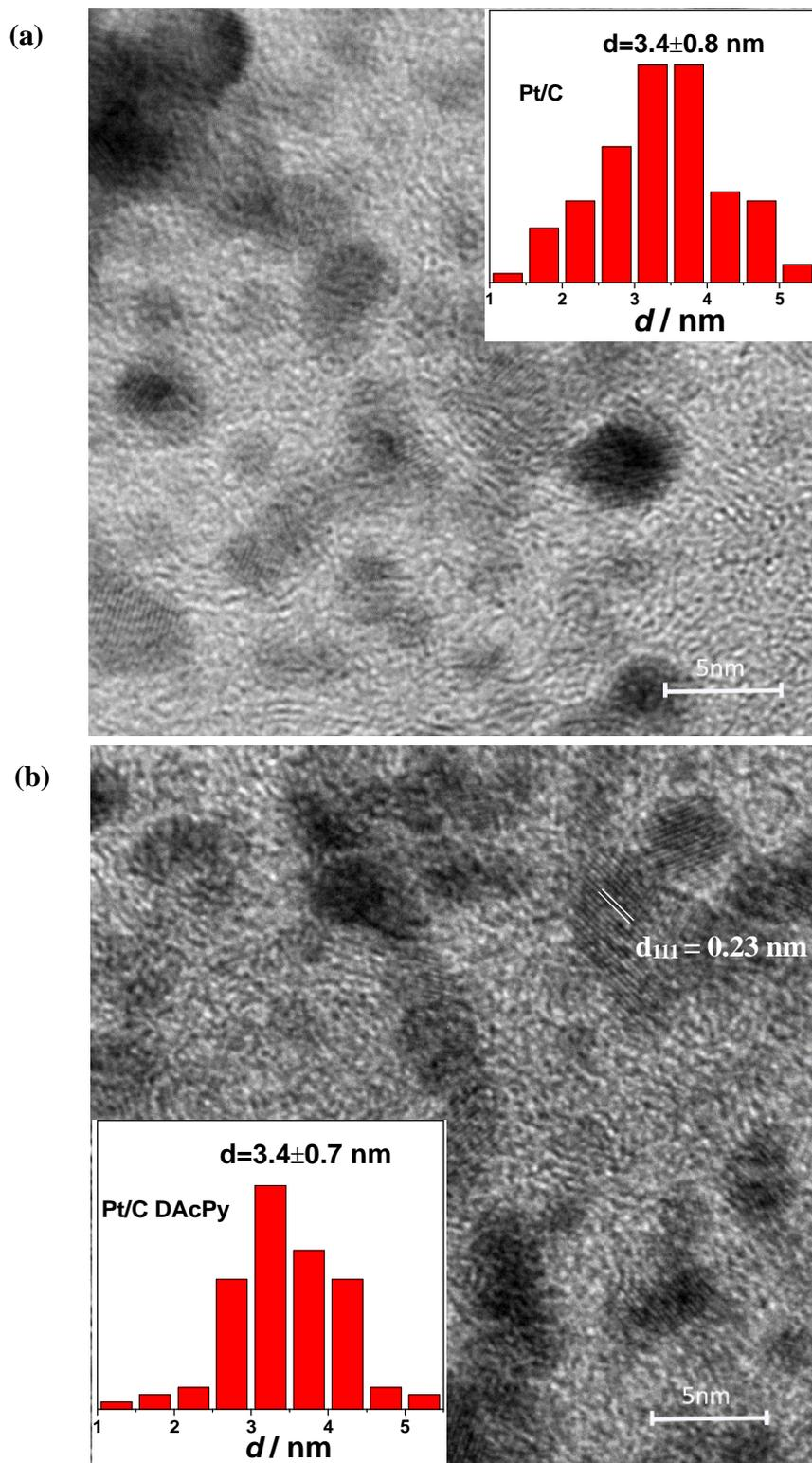
**Fig. S1** HRTEM images of Pt/C (a) and DAcPy-coated Pt/C (b). Size histograms were inset. The lattice space of 0.23 nm, corresponding to (111) diffraction of Pt could be observed.
