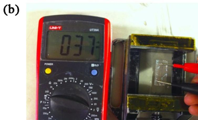
**Fig. S5.** Resistance of the PEN/Ag NW network on the (a) glass/PDMS supporting substrate and peeled away from the glass/PDMS and adhered on a pre-stretched elastomer. During transforming the PEN/Ag NW electrode no significant difference in the resistance was observed.
