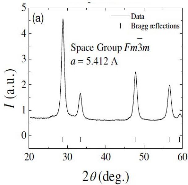
**SI Figure 2.** X-ray diffraction pattern of  $n\text{CeO}_2$ . Powder XRD patterns were collected in the Bragg-Brentano geometry within  $20^\circ$ - $60^\circ$   $2\theta$ -range ( $\lambda=1.5406\text{\AA}$ ).
