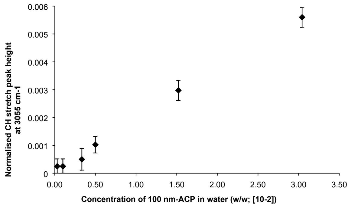
Figure SI-6: Limit of detection for 110 nm-ACP: SRS hyperspectral profiles were obtained from successive dilutions of 110 nm-ACP in standardised dilution water. The peak heights were measured relative to standardised dilution water and were normalised to the peak value for pure 110 nm-ACP, which was assigned a value of 1.
