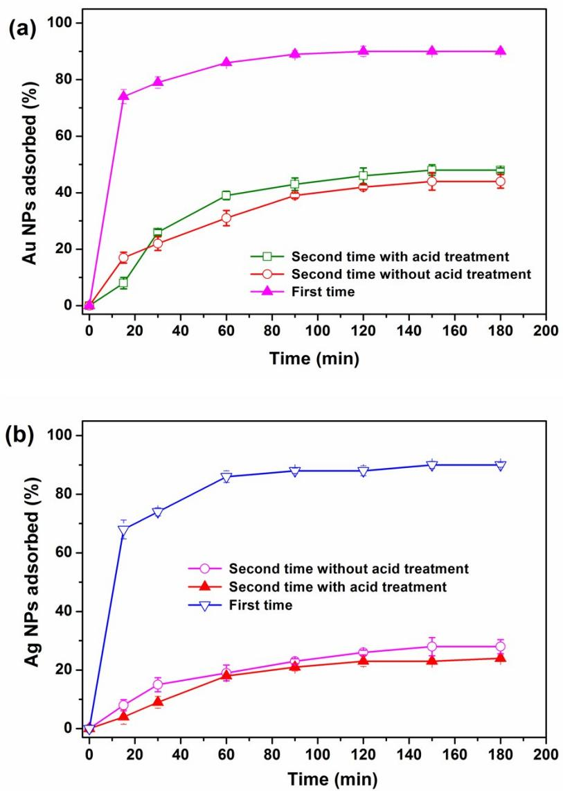
**Figure S7.** The adsorption efficiencies of MCFAs@CS@PDA/PEI for first time adsorption, second time without and with acid treated fibers using citrate capped Au-nanoparticles (a,  $2.72 \times 10^{-4}$  M) and citrate capped Ag-nanoparticles (b,  $6.5 \times 10^{-4}$  M).
