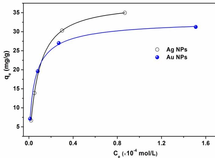
**Figure S5.** Plot of isothermal adsorption for the adsorption of Au and Ag nanoparticles onto MCFAs@CS@PDA/PEI at 303 K.
