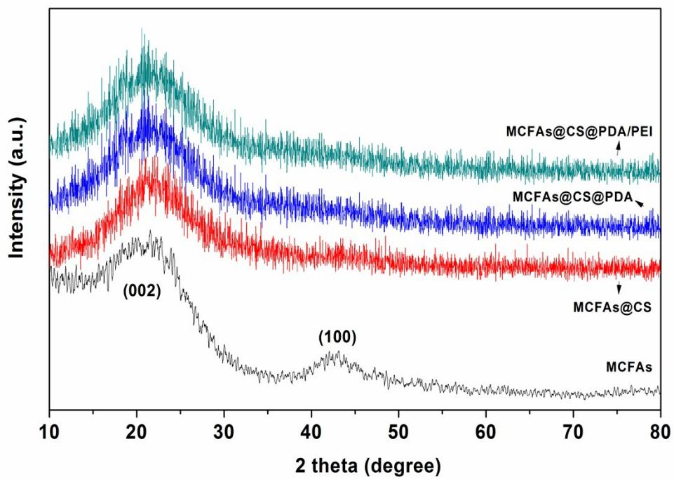
**Figure S9.** XRD patterns of MCFAs, MCFAs@CS, MCFAs@CS@PDA and MCFAs@CS@PDA/PEI composites ( $\lambda = 1.54 \text{ \AA}$ )
