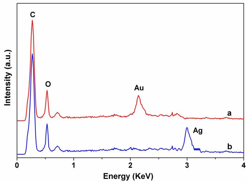
**Figure S4.** EDS data of MCFAs@CS@PDA/PEI after adsorption of (a) Au NPs and (b) Ag NPs.
