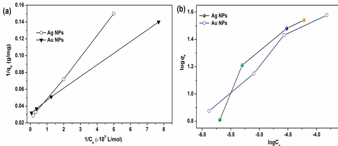
**Figure S3.** Plots of linear Langmuir (a) and Freundlich isotherm (b) models for the adsorption of Au and Ag nanoparticles onto MCFAs@CS@PDA/PEI at 303 K.
