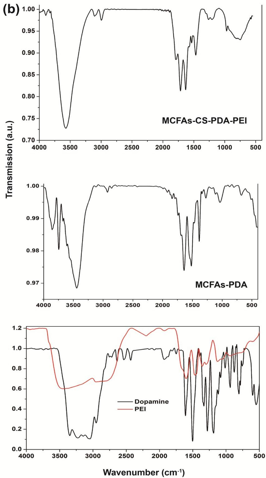
**Figure S8.** FTIR/ATR spectra of the chitosan (CS), MCFAs-CS, MCFAs-COOH and MCFAs (a); MCFAs-CS-PDA-PEI, MCFAs-PDA, dopamine and polyethyleneimine (b).
