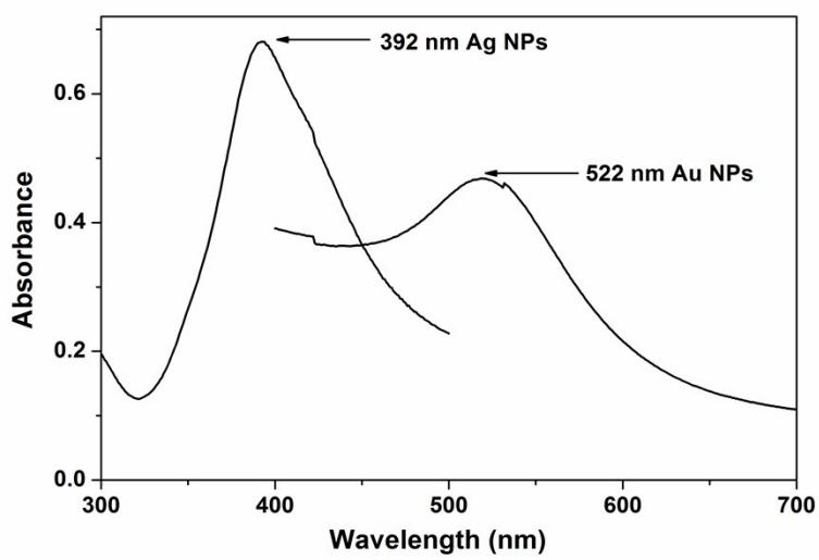
**Figure S2.** UV-Vis spectra of citrate capped Au and Ag nanoparticles.
