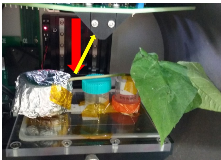
Fig. S2. Setup used to monitor in vivo Zn uptake using a 1 mm \varnothing X-ray beam. The red arrow illustrates the incoming X-ray beam and the yellow one the outgoing Zn X-ray fluorescence.
