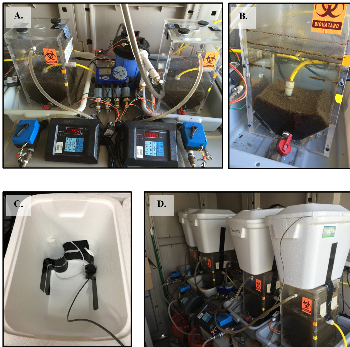
Figure S2. Top: Photos of (A) timers and valves used to control flow of primary and secondary effluent, compressed air, and WAS and (B) an example of one of the SBRs at the end of the settling phase/start of the discharge phase. Bottom: Photos of (C) system used to deliver antibiotic spike solutions and (D) SBR configuration during phase 2 testing.
