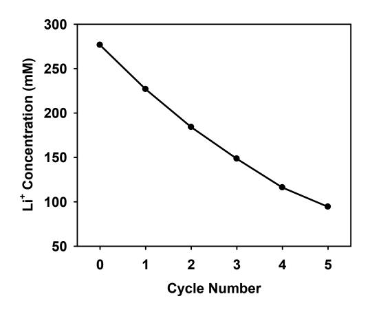
Fig. S1. The concentration of lithium ions in the wastewater during the 5 cycles of LMO/BDD
