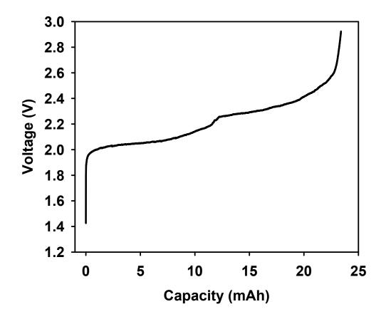
Fig. S2. Voltage profile of LMO/BDD system under operation at 25 mA (100 mA/ $g_{LMO}$  and 12.5 mA/ $cm^2_{BDD}$  of current density)
