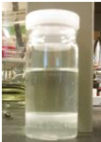
Fig S4: Picture of a typical catalytic test for the epoxidation of methyl oleate (water and EtOAc added to increase the volumes of each phase for clarity). The catalyst ( [(DP^{2+})_3[PPW^{3-}]_2] ) floats between the organic phase (top) and the aqueous phase (bottom).
