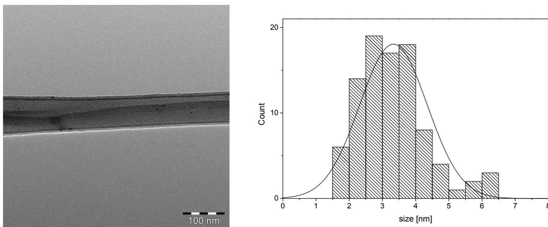
Figure S 3: TEM picture of Ru-NPs dispersed in [C<sub>1</sub>C<sub>1</sub>(EG)MIM]NTf<sub>2</sub> (30  $\mu$ mol metal in 0.3 ml IL, 90  $^{\circ}$ C, 1 h) and histogram of size distribution. The mean particle diameter is 3.3  $\pm$  1.0 nm.
