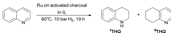
Table S 1: Hydrogenation of quinoline using Ru on activated charcoal in [C<sub>1</sub>C<sub>1</sub>(EG)IM]NTf<sub>2</sub>.
