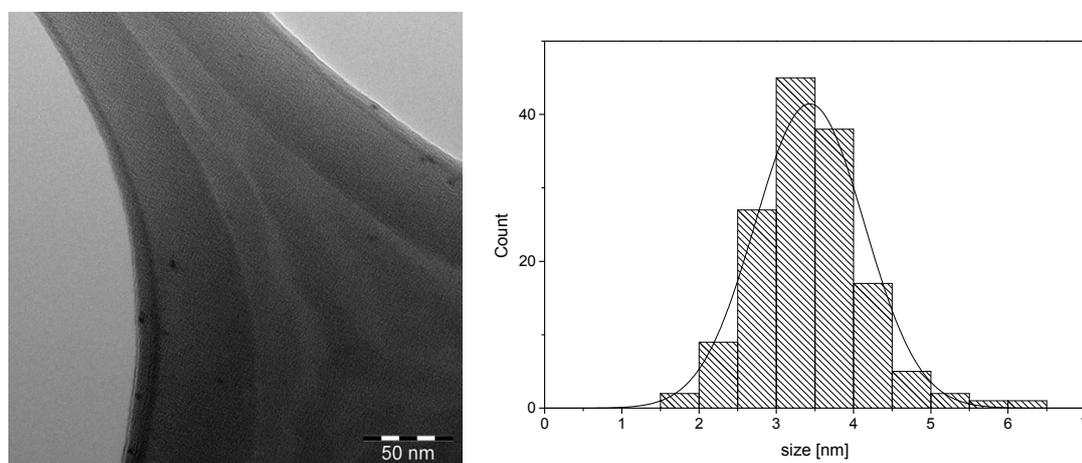
Figure S 5: TEM picture of Ru-NPs dispersed in  $[C_2OHMIM]NTf_2$  (30  $\mu\text{mol}$  metal in 0.3 ml IL, 90  $^{\circ}\text{C}$ , 18 h, after catalysis, hydrogenation of quinoline, 80  $^{\circ}\text{C}$ , 10 bar  $\text{H}_2$ , 19 h) and histogram of size distribution. The mean particle diameter is  $3.4 \pm 0.7$  nm.
