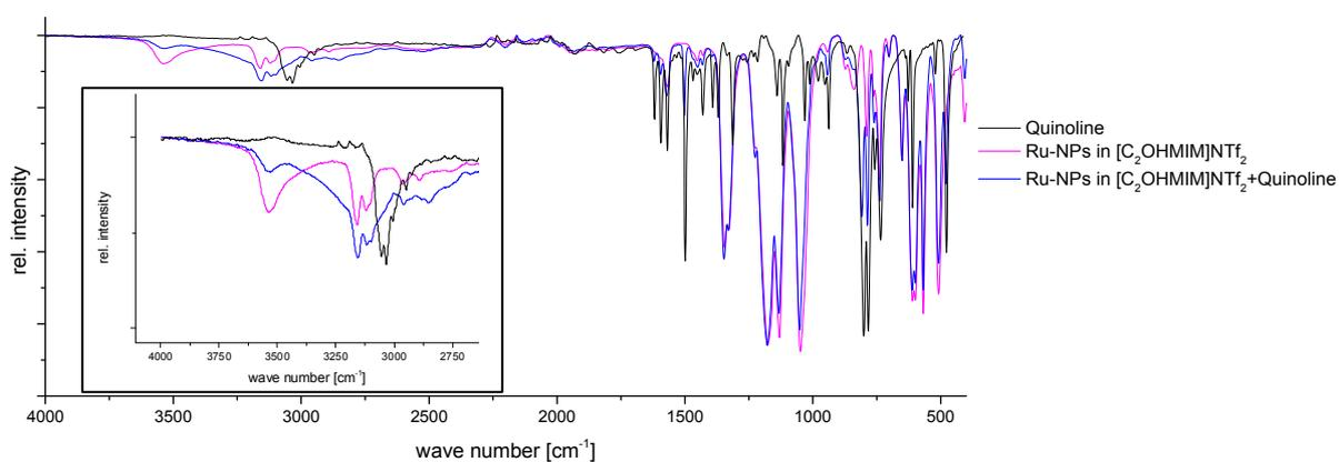
Figure S 9: IR spectra of quinoline, Ru-NPs embedded in [C<sub>2</sub>OHmIM]NTf<sub>2</sub> and a mixture of both.
