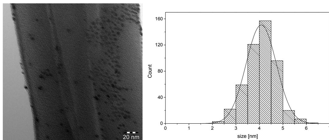
Figure S 6: TEM picture of Ru-NPs dispersed in  $[C_1C_1(EG)MIM]NTf_2$  (30  $\mu\text{mol}$  metal in 0.3 ml IL, 90  $^{\circ}\text{C}$ , 1 h, after six runs of recycling of the hydrogenation of quinoline, 80  $^{\circ}\text{C}$ , 10 bar  $\text{H}_2$ , 19 h) and histogram of size distribution. The mean particle diameter is  $4.1 \pm 0.6$  nm.
