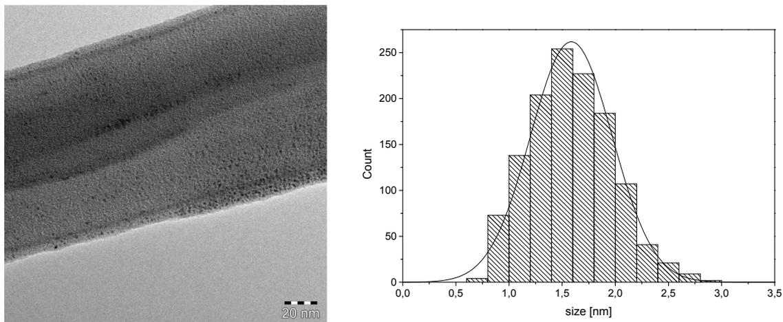
Figure S 1: TEM picture of Ru-NPs dispersed in [BMMIM]NTf<sub>2</sub> (38  $\mu$ mol metal in 0.3 g IL, 90  $^{\circ}$ C, 18 h, after catalysis, hydrogenation of quinoline, 80  $^{\circ}$ C, 10 bar H<sub>2</sub>, 5h) and histogram of size distribution. The mean particle diameter is 1.6  $\pm$  0.4 nm.
