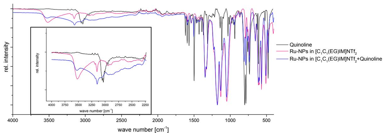
Figure S 8: IR spectra of quinoline, Ru-NPs embedded in [C<sub>1</sub>C<sub>1</sub>(EG)IM]NTf<sub>2</sub> and a mixture of both.
