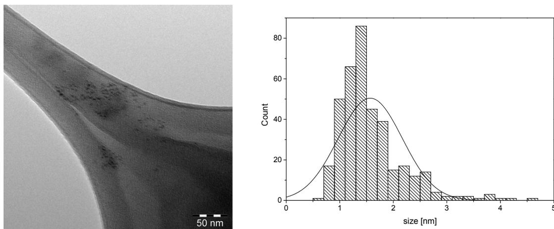
Figure S 2: TEM picture of Ru-NPs dispersed in [BMIM]NTf<sub>2</sub> (38  $\mu$ mol metal in 0.3 g IL, 90  $^{\circ}$ C, 18 h) and histogram of size distribution. The mean particle diameter is 1.6  $\pm$  0.6 nm.
