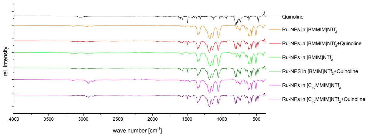
Figure S 7: IR spectra of quinoline, Ru-NPs embedded in different imidazolium based ILs and mixtures of both.
