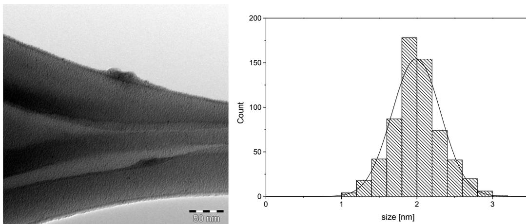
Figure S 4: TEM picture of Ru-NPs dispersed in  $[C_{10}MMIM]NTf_2$  (38  $\mu\text{mol}$  metal in 0.3 g IL, 90  $^{\circ}\text{C}$ , 18 h, after catalysis, hydrogenation of quinoline, 80  $^{\circ}\text{C}$ , 10 bar  $\text{H}_2$ , 5 h) and histogram of size distribution. The mean particle diameter is  $2.0 \pm 0.3$  nm.
