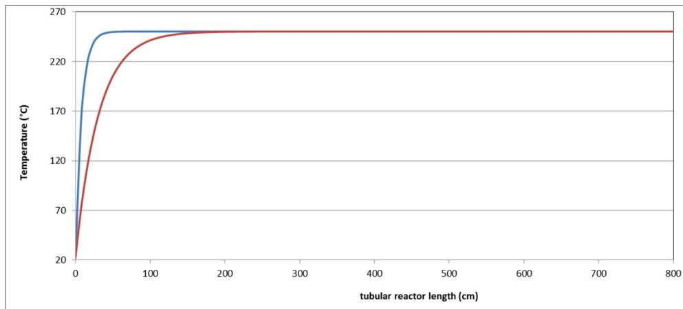
**Figure S11.** The red and blue curves illustrate the theoretical temperature distribution along the tubular reactor for an internal diameter of 500 and 1000  $\mu\text{m}$ , respectively.
