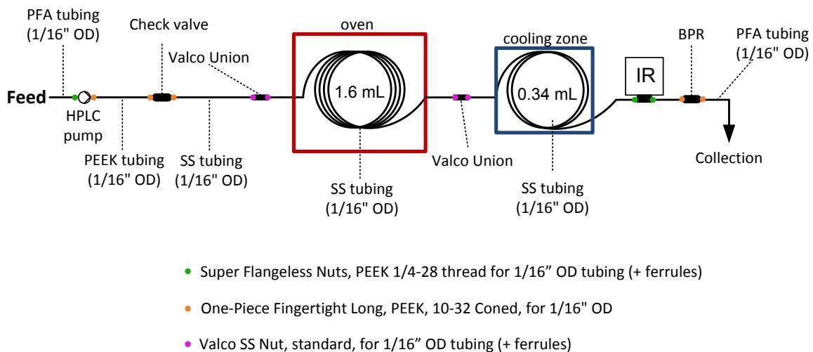
**Figure S1.** Microfluidic thermolysis setup
