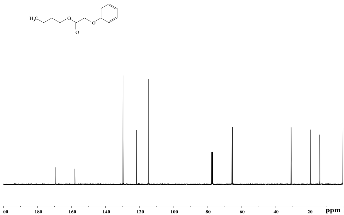
^{13}\text{C} NMR spectrum of butyl 2-phenoxyacetate ( \text{CDCl}_3 , 126 MHz)
