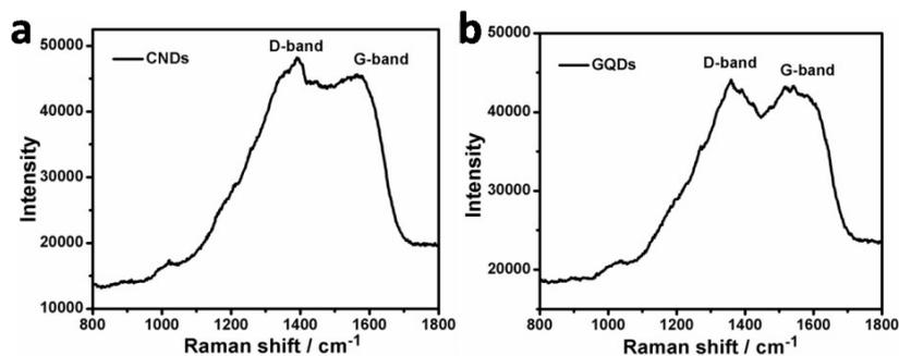
**Fig. S4** Raman spectra of the (a) CNDs and (b) GQDs.
