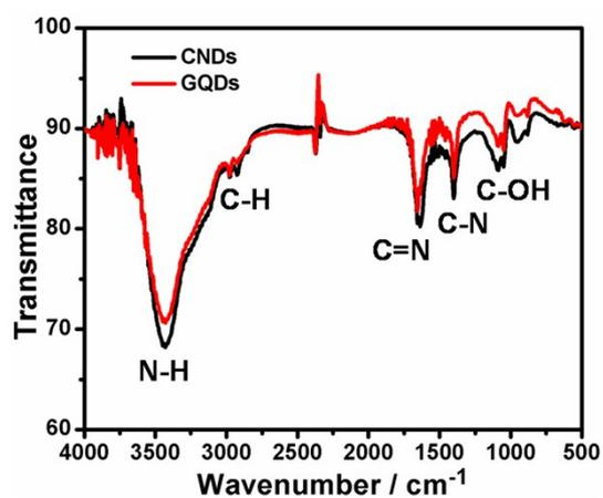
**Fig. S2** FT-IR spectra of the CNDs and GQDs.
