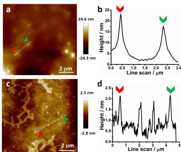
**Fig. S3** AFM images of the (a) CNDs and (c) GQDs; (b) measured height profile along the white line in (a); (d) measured height profile along the white line in (c).
