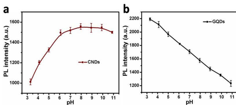
**Fig. S7** Variation in the PL intensities of CNDs and GQDs with the different pH value.
