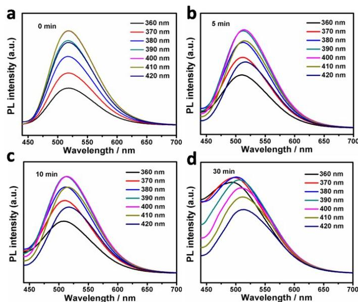
**Fig. S8** The emission spectra of CNDs with different exposure times. (a) 0 min; (b) 5 min; (c) 10 min and (d) 30 min. The powder of Xe lamp is 140 W. EX: 400 nm;  $C_{\text{CNDs}}$ : 10  $\mu\text{g/ml}$ .
