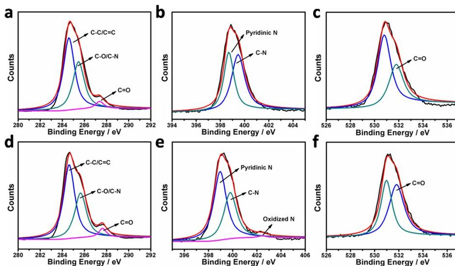
**Fig. S6** The high-resolution XPS spectra of the CNDs and GQDs. (a) C1s; (b) N1s and (c) O1s spectra of CNDs. (d) C1s; (e) N1s and (f) O1s spectra of GQDs.
