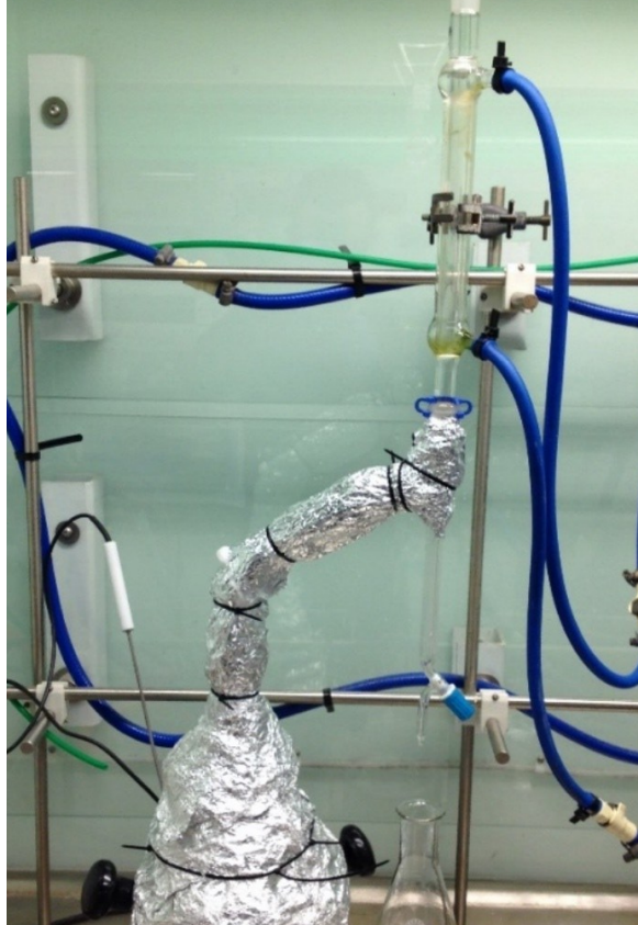
Figure S3. The Dean Stark-type reactive distillation apparatus which was used to produce TMTHF on a litre scale.
