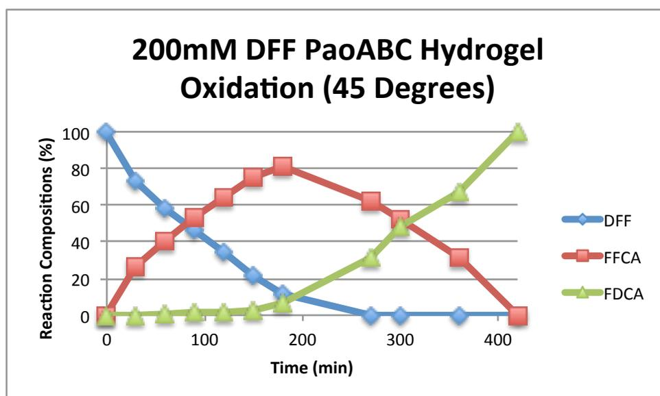
**Figure S30** Time course analysis of the oxidation of 200 mM DFF by PaoABC Hydrogel at 45°C
