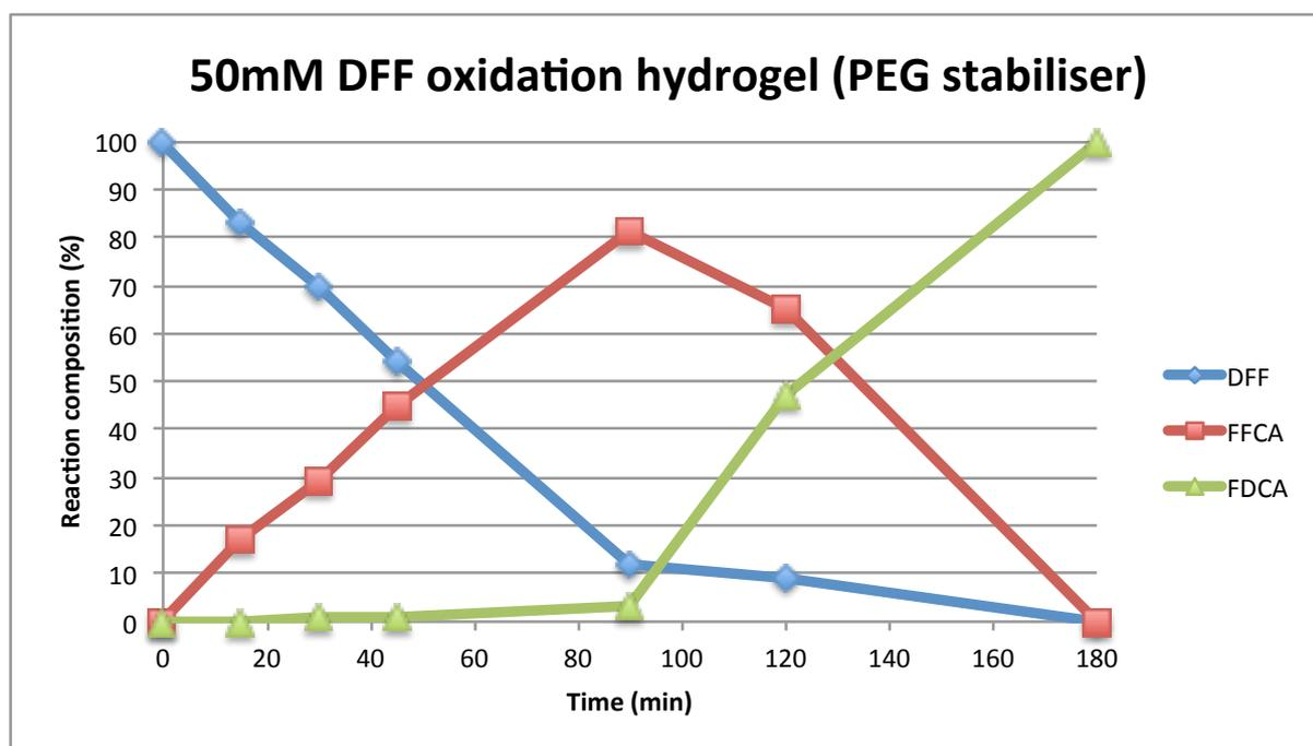
**Figure S13** Time course analysis of the oxidation of 50 mM DFF by PaoABC hydrogel (PEG stabilised)
