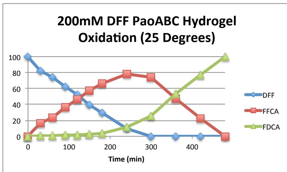
**Figure S26** Time course analysis of the oxidation of 200 mM DFF by PaoABC Hydrogel at 25°C
