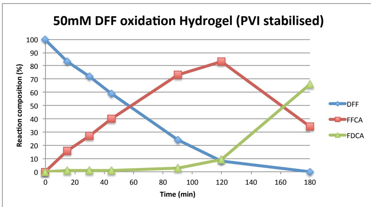
**Figure S11** Time course analysis of the oxidation of 50 mM DFF by PaoABC hydrogel (PVI stabilised)
