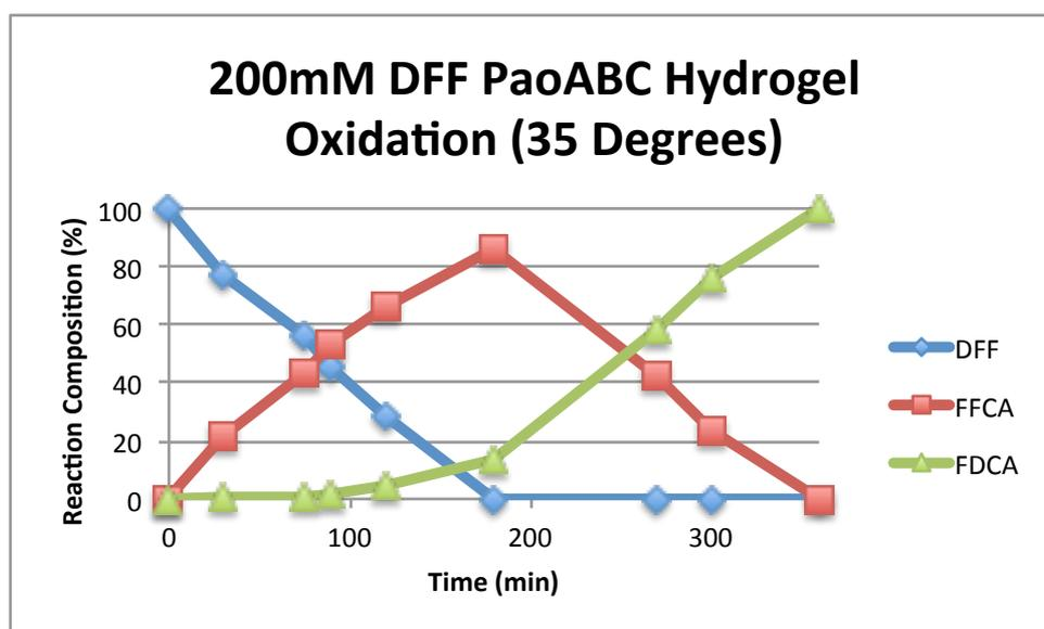
**Figure S28** Time course analysis of the oxidation of 200 mM DFF by PaoABC Hydrogel at 35°C
