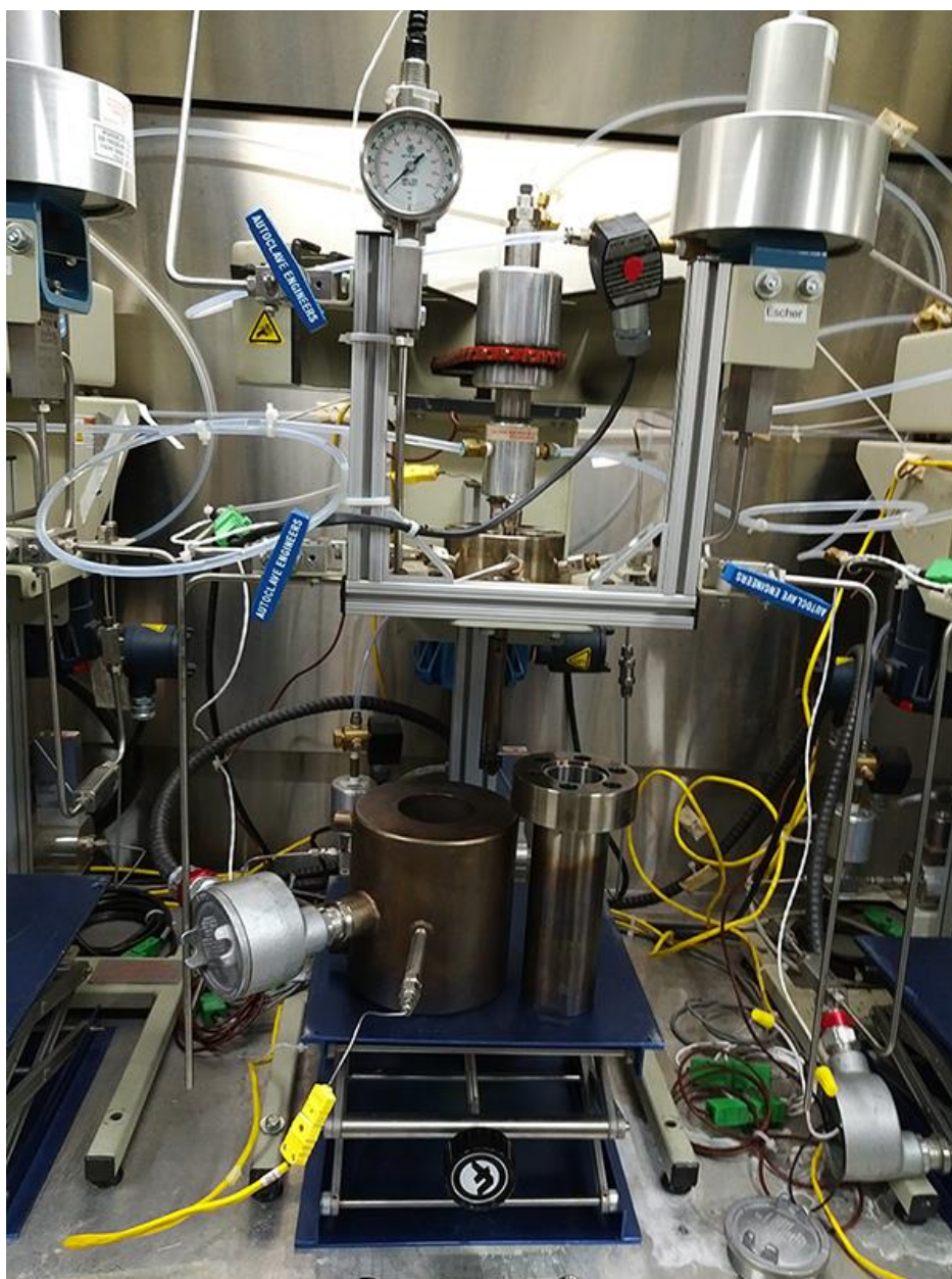
Figure S16: Overall Reactor set-up at the University of Guelph High-Pressure Hydrogenation Facility.
