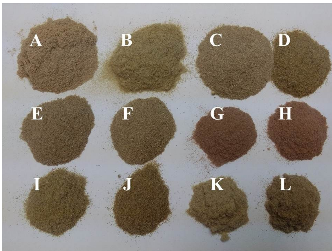
Electronic supplemental information 3 Morphological structure of untreated and pretreated corn stover by different combinatorial pretreatment strategies. A, untreated corn stover; B, pretreated corn stover in Case 1; C, pretreated corn stover in Case 2; D, pretreated corn stover in Case 3; E, pretreated corn stover in Case 4 Step 1; F, pretreated corn stover in Case 5 Step 1; G, pretreated corn stover in Case 6 Step 1; H, pretreated corn stover in Case 7 Step 1; I, pretreated corn stover in Case 4 Step 2; J, pretreated corn stover in Case 5 Step 2; K, pretreated corn stover in Case 6 Step 2; L, pretreated corn stover in Case 7 Step 2.
