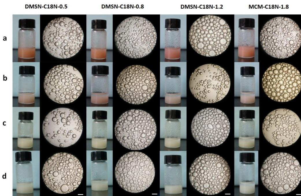
**Fig. S4** Photographs and microscopic images of emulsion systems with DMSN-C18N-X and MCM-C18N-1.8. Emulsion formation: 60 mg silica nanospheres, 1 mL of H<sub>2</sub>O (including Rh  $3.0 \times 10^{-3}$  mmol, P/Rh=15) and 1 mL of 1-dodecene. The emulsions were kept under static conditions for different time intervals (scale bar, 200  $\mu$ m). (a) newly formed, (b) after 1 day, (c) after 3 days, (d) after 10 day.
