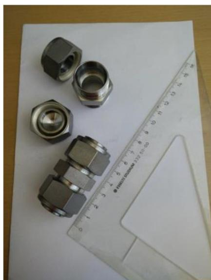
**Fig S15.** Photo of reactors made of one stainless steel Swagelok unit (SS-1210-6) and two stainless steel plugs (SS-1210-P).
