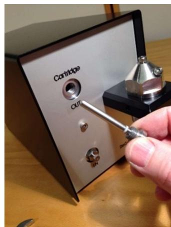
**Fig S4.** Cartridge installation.
