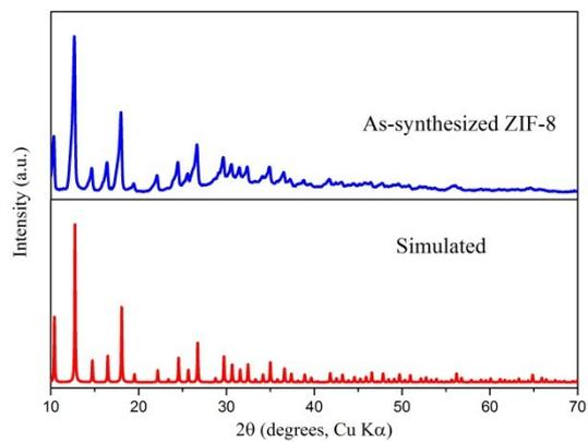
Fig. S1 XRD pattern of the as-prepared ZIF-8.
