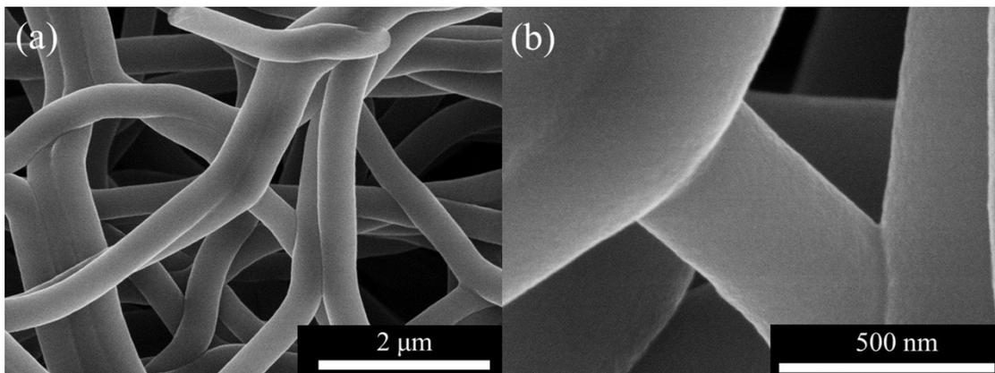
Fig. S6 FE-SEM images of CFs at different magnifications.
