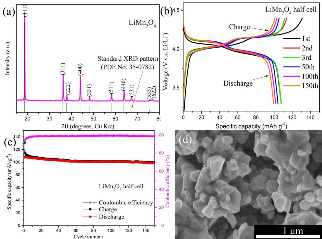
**Fig. S9** (a) XRD pattern of the as-prepared  $\text{LiMn}_2\text{O}_4$ ; (b) Charge/discharge profiles of  $\text{LiMn}_2\text{O}_4$  cathode within a voltage range of 3.3-4.4 V; (c) Cycling performance of  $\text{LiMn}_2\text{O}_4$  electrode at a current density of  $100 \text{ mA g}^{-1}$ ; (d) FE-SEM image of  $\text{LiMn}_2\text{O}_4$  nanoparticles.
