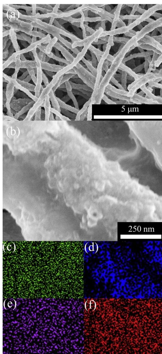
Fig. S8 (a and b) FE-SEM images of the Mn<sub>3</sub>O<sub>4</sub>/NPCFs-1.4 electrode after 100 cycles at different magnifications. (c-f) Elemental mapping images of C, N, O and Mn, respectively.
