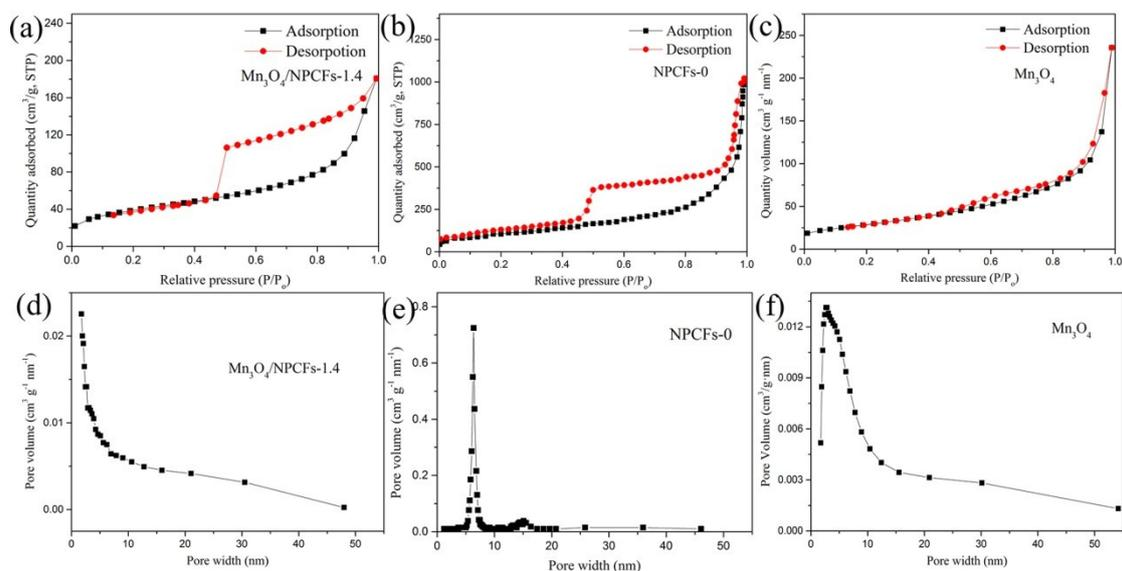
Fig. S4 Nitrogen adsorption–desorption isotherms of the as-synthesized products (a-c) and their corresponding pore size distribution curves (d-f) calculated from the adsorption branch by the BJH model.
