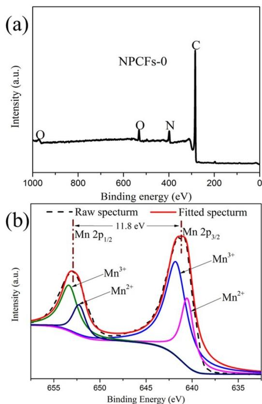
Fig. S3 (a) XPS survey spectra of NPCFs-0; (b) High-resolution XPS spectra of deconvoluted Mn 2p peak for the Mn<sub>3</sub>O<sub>4</sub>/NPCFs-1.4 product.
