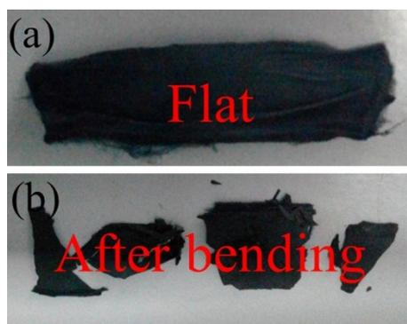
Fig. S2 Digital photographs of CFs mats before and after bending.
