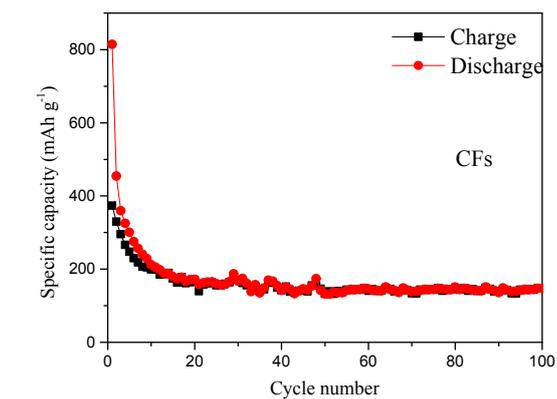
Fig. S7 Cycling test of CFs at a current density of 100 mA g<sup>-1</sup>.
